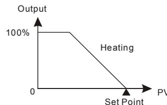
Figure 3: PID Control, Heating Control
