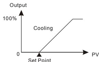
Figure 2: PID Control, Cooling) Control
