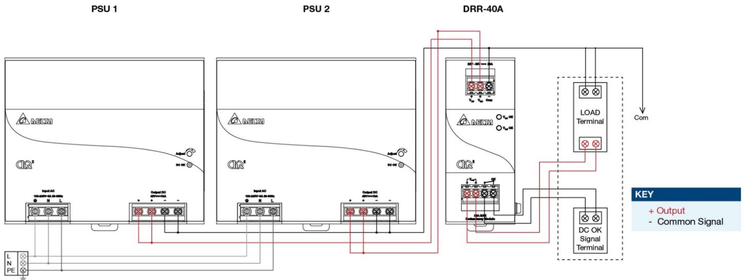
Fig. 3 Redundancy / Parallel Operation Connection Diagram
