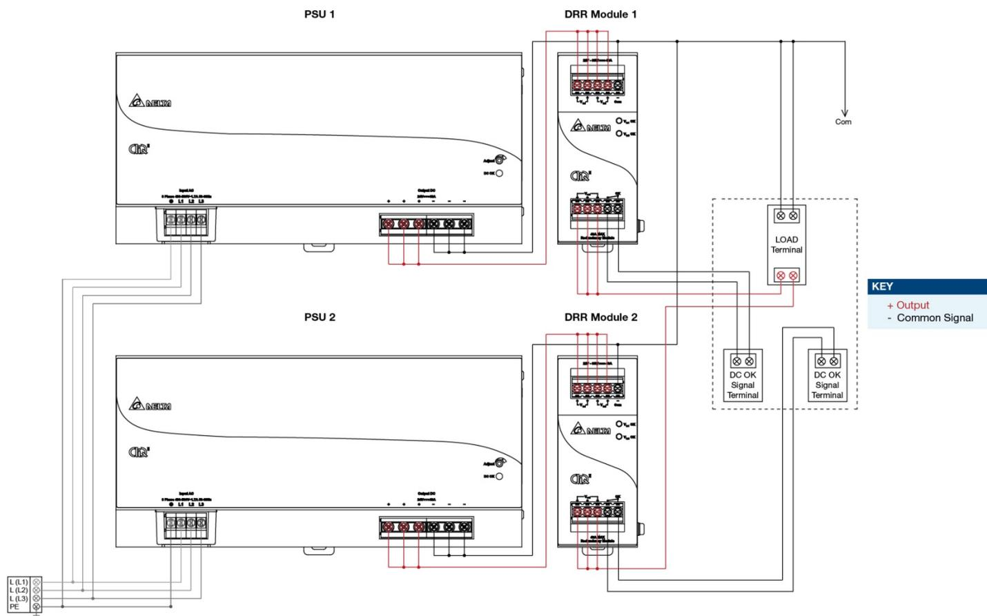
Fig. 3 Redundancy / Parallel Operation Connection Diagram
