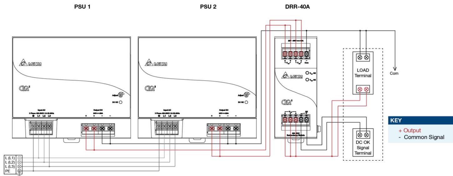
Fig. 3 Redundancy / Parallel Operation Connection Diagram
