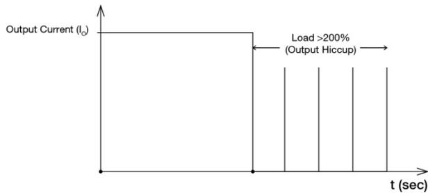
It is not recommended to prolong the duration of  $I_O$  when it is <200% but >100%, since it may cause damage to the PSU.
