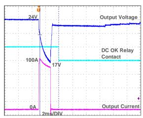
Fig. 7.2 APB 500% of nominal output current for 2ms
