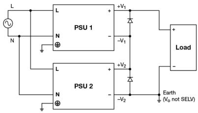
Fig. 10 Series Operation Connection Diagram
