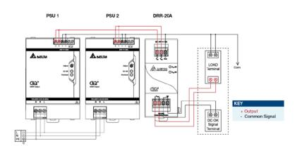
Fig. 8 Redundancy Operation Connection Diagram
