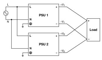
Fig. 9 Parallel Operation Connection Diagram
