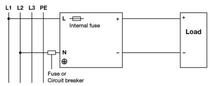
Fig. 12 2 of 3 Phase System Input Operation Connection Diagram
