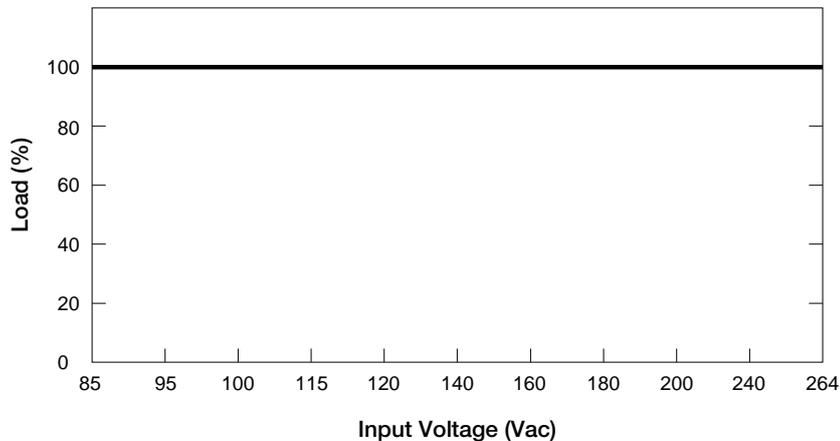
■ No output power de-rating for the input voltage range
