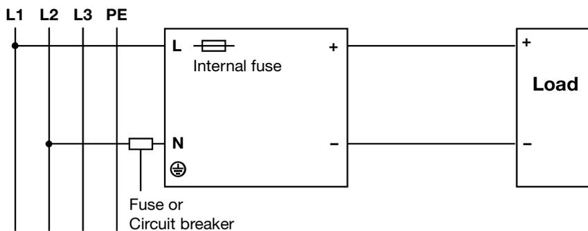
Fig. 12 2 of 3 Phase System Input Operation Connection Diagram
