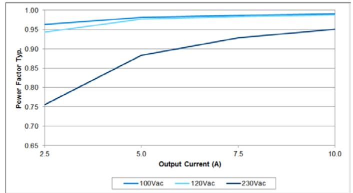
Fig. 4 Power Factor Vs Output Load at 24V
