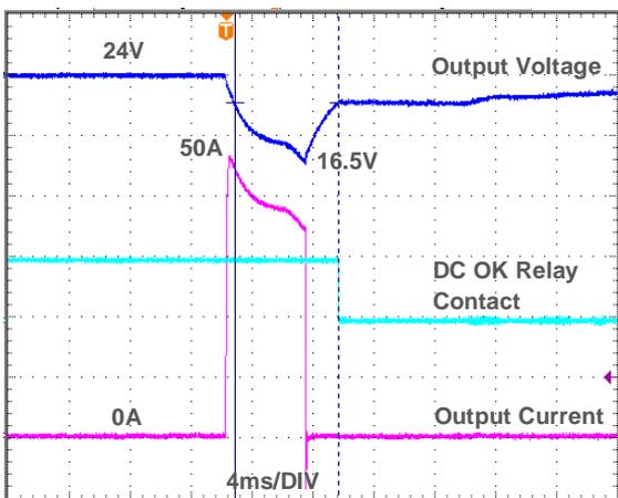
Fig. 7.3 APB 500% of nominal output current for 5ms
