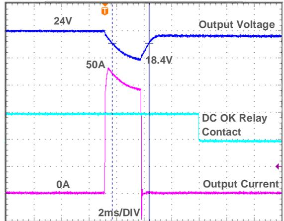
Fig. 7.2 APB 500% of nominal output current for 2ms
