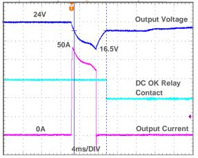
Fig. 7.3 APB 500% of nominal output current for 5ms
