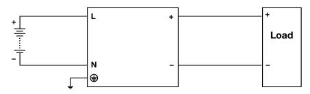
Fig. 11 DC Input Operation Connection Diagram
