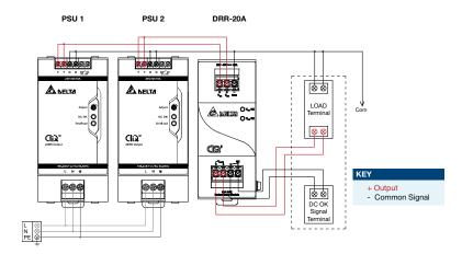
Fig. 8 Redundancy Operation Connection Diagram
