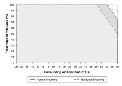
Fig. 5De-rating for Vertical Mounting Orientation<br/>> 60°C de-rate power by 2.5% / °C
