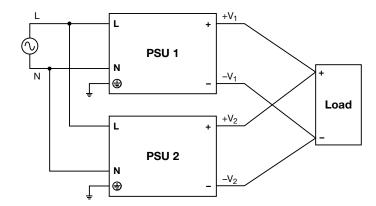
Fig. 9 Parallel Operation Connection Diagram
