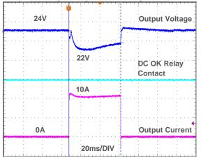
Fig. 7.1 APB 200% of nominal output current for 50ms
