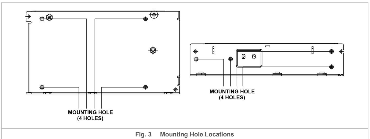
Fig. 3 Mounting Hole Locations
