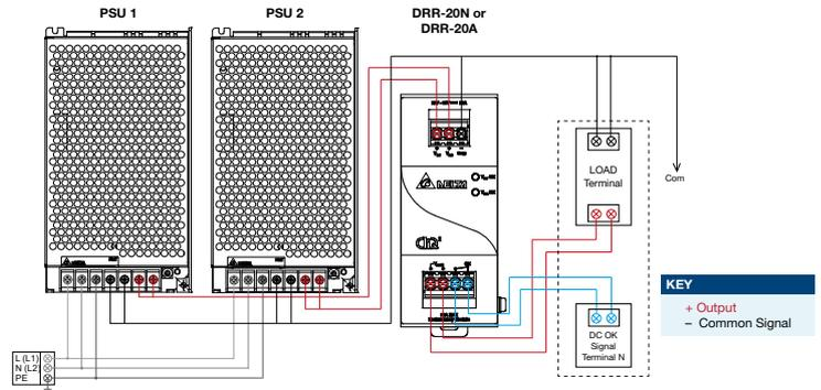
Fig. 5 Redundancy Operation Connection Diagram
