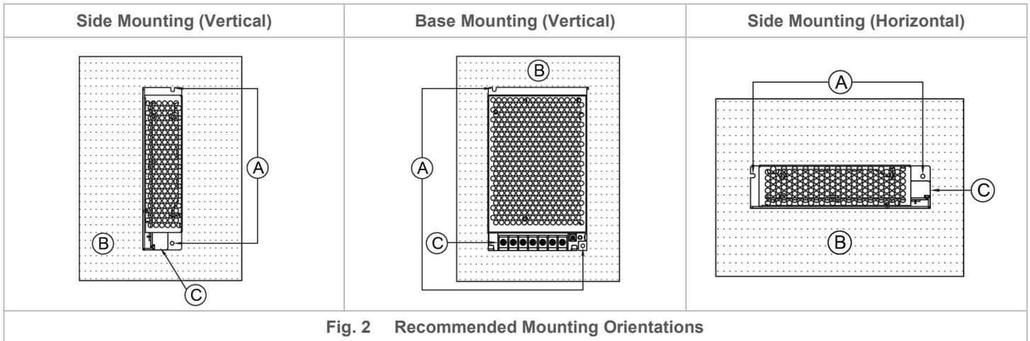
Fig. 2 Recommended Mounting Orientations
