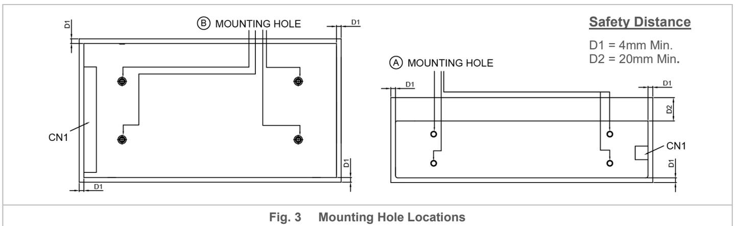
Ensure the mounted device is kept at  $\geq 4$  mm (0.16 inch) safety distance at all sides from other components and equipments. In addition, to ensure sufficient convection cooling, always maintain a distance of  $\geq 20$  mm (0.79 inch) from fan ventilated surfaces while the device is in operation. Please insert an insulation sheet between the system and product, if the safety distance is  $< 4$  mm (0.16 inch).
