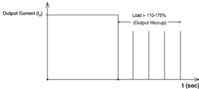
It is not recommended to prolong the duration of  $I_o$  when it is <110% but >100%, since it may cause damage to the PSU.
