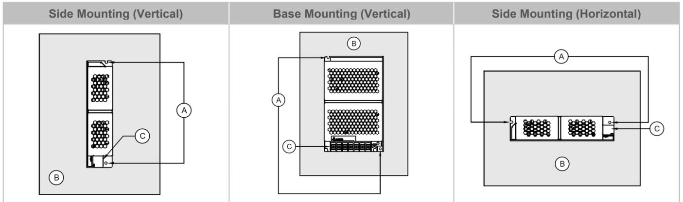
Fig. 2 Mounting Orientation
