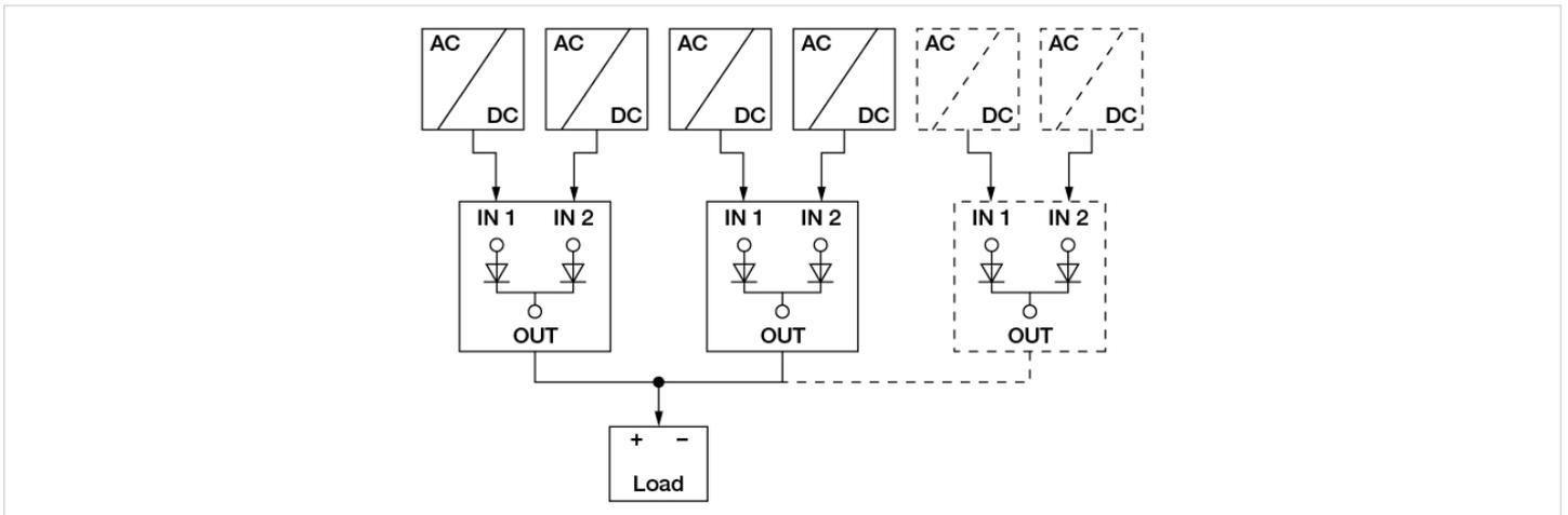
Connecting only one PSU to one DRR module to reduce the stress of the diodes and hence increase the reliability.
