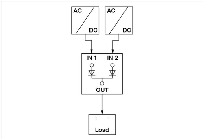
Using 1 more PSU as the redundant unit.
