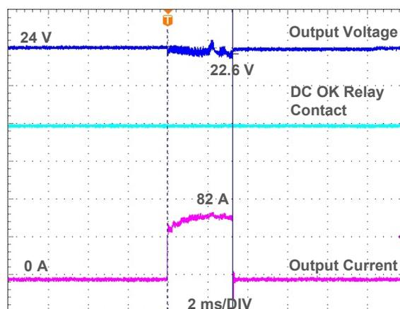
Fig. 8.2 APB 400% of nominal output current for 2 ms
