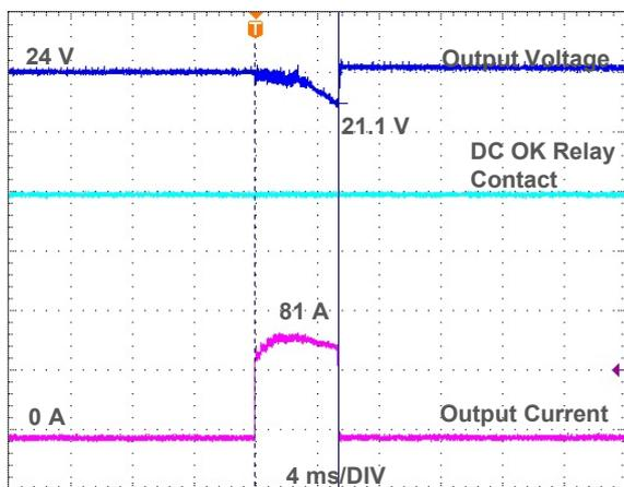
Fig. 8.3 APB 400% of nominal output current for 5 ms
