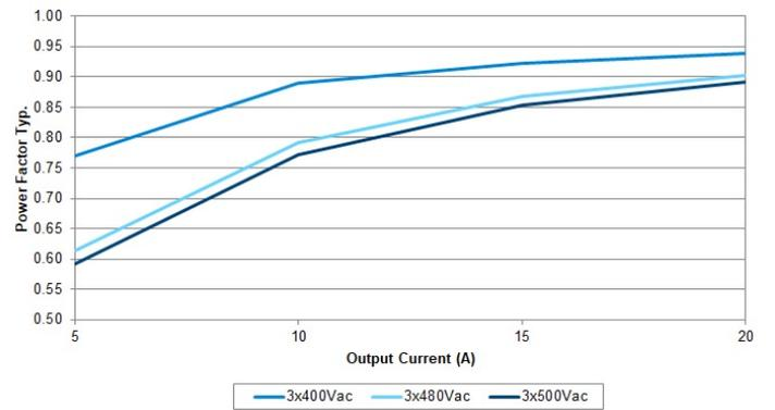
Fig. 4 Power Factor VS Output Load at 24 V
