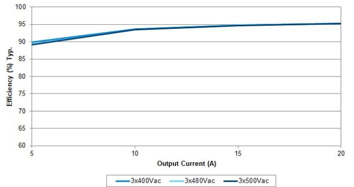
Fig. 2 Efficiency VS Output Load at 24 V
