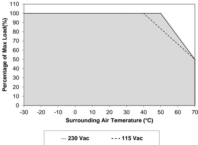
**Fig. 1 De-rating for Vertical Mounting Orientation**
