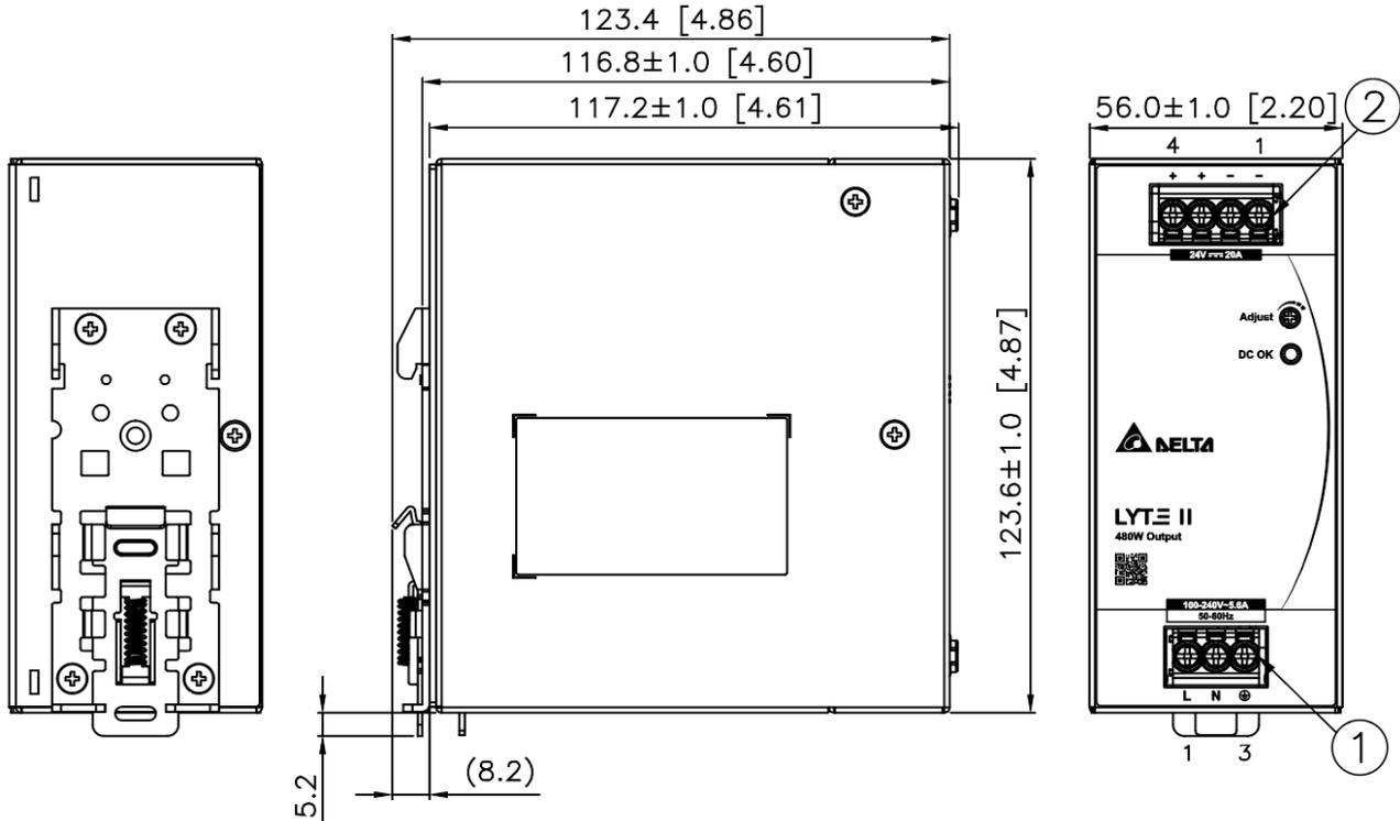
\*Unless otherwise specified tolerance of dimension are  $\pm 0.5$  mm
