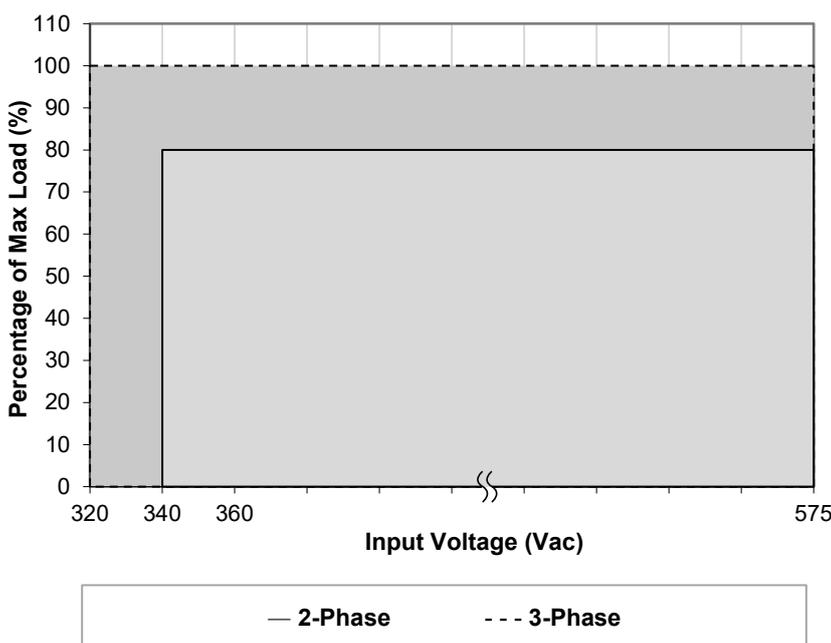
**Fig. 2 De-rating for AC Input Voltage**
