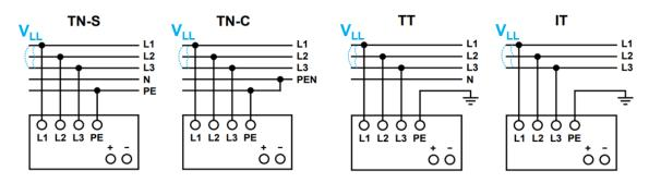
Fig. 4 AC Input Operation Connection Diagram
