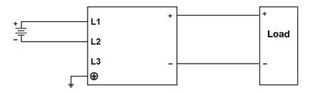
Fig. 5 DC Input Operation Connection Diagram
