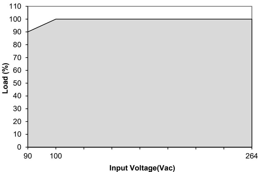
**Fig. 2 De-rating for AC Input Voltage**
