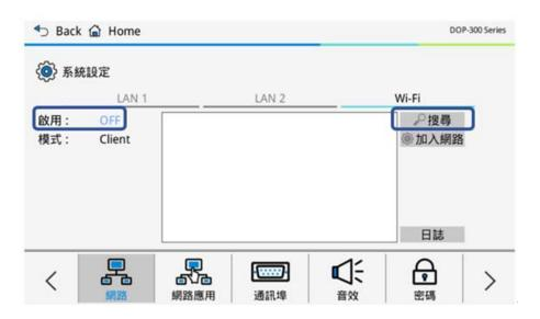
13. After searching, select the network name that can be connected and enter the account number and password to connect.
