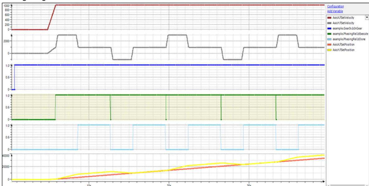
1. Run `DMC_GearIn`, establish a master-slave relationship, and then use `MC_MoveVelocity` to make the master axis run at the same speed.
