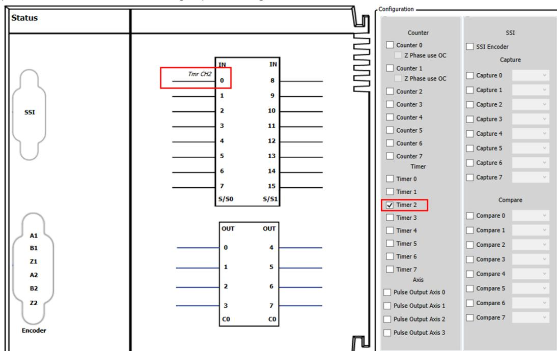
2. After using the FB DFB\_HTmr in the POU to activate the high-speed timer(bEnable = True), it starts receiving and counting the pulses from the external signals(IN 0) based on the timing mode set in Timer Configuration, then the timed value would be displayed in the output dwTimerValue.
