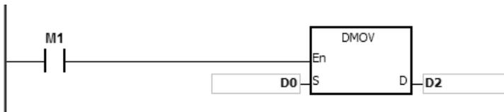
When M1 is ON, the data in (D1, D0) is transferred to (D3, D2).
