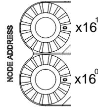
Example: If users need to set the node address of AH10PFBS-5A to 26 (decimal value), they have to turn the knob corresponding to  $x16^1$  to "1", and the knob corresponding to  $x16^0$  to "A".
