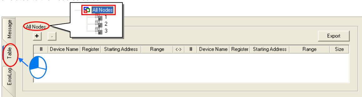
If the users click **+**, a new piece of data will be added to the table. A piece of data is composed of two parts. The left part of the data in the figure below indicates that the data demanding node AH-01 will store the data demanded in L0 in itself, and the right part of the data in the figure below indicates that the data supply node AH-02 will supply the data in L0 in itself.
