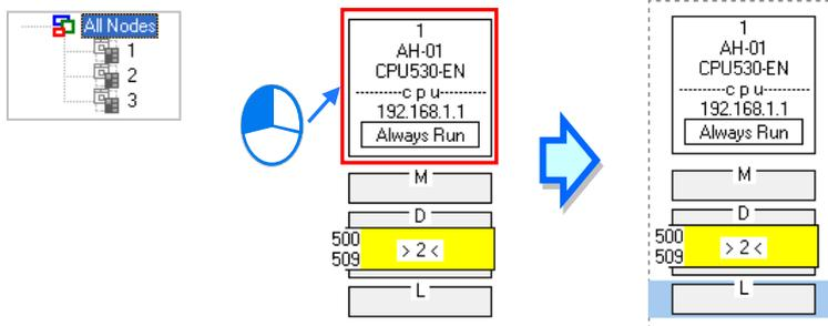
Once a node is selected, the node will be designated as a data demanding node. After the users click a device block in the node selected, a blue cursor will appear. After the users click a device block in another node (a data supply node), a green cursor will appear. The users can only click a device block in a data supply node. They can not select the node, otherwise the node will be designated as a data demanding node.
