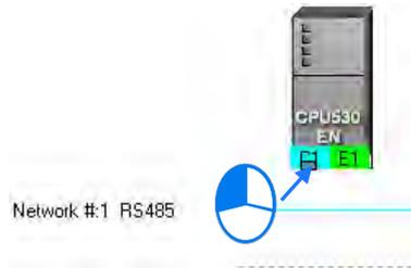
The users move the mouse cursor to the existing network while holding the left mouse button down. If the network matches the port, the port will connect to the network after the users release the left mouse button.
