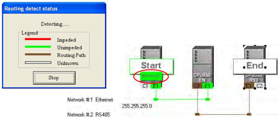
(4) After the detection is complete, the detection result will be shown in the working area.
