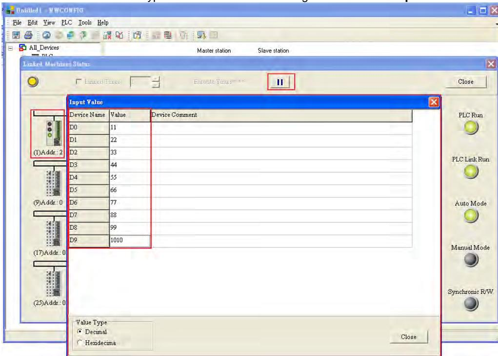
**Step 4:** The users have to right-click **(1) Addr.: 2**, and click **Read Register** on the context menu. The values in the **Input Value** window indicate that the data exchange is performed correctly.
