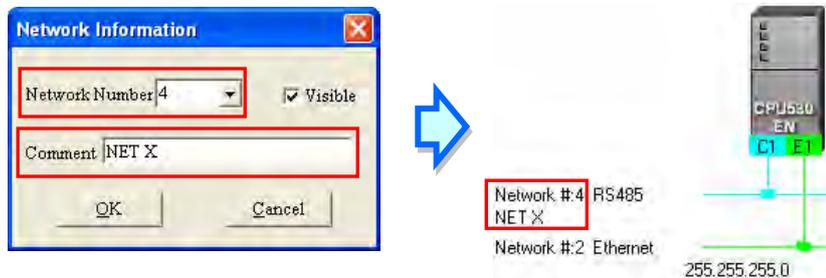
If the users unselect the **Visible** checkbox in the **Network Information** box, the network and the devices connected to the network will become invisible, the other devices connected to the other networks will still be displayed, and the lines connected to the network will become dotted lines. Please refer to section 9.2.5 for more information about hiding/displaying devices or networks.
