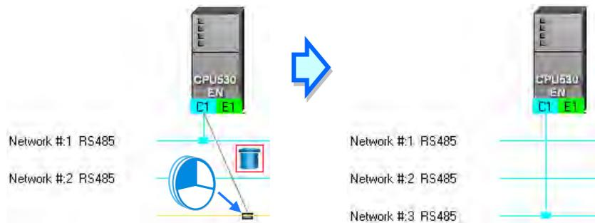
If the users release the left mouse button after they drag the connection point to another network which matches the port, the port will be connected to the network.
