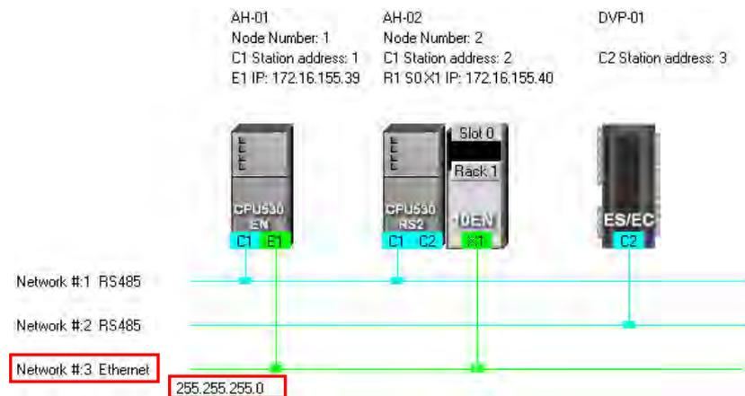
If the ports connected to an Ethernet network are not in the same domain, or are not assigned the same subnet mask, a warning sign will appear. If the ports connected to an Ethernet network are not assigned the same subnet mask, the strictest subnet mask will be shown.
