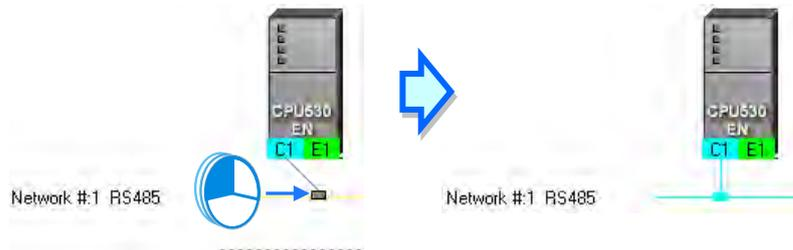
If the users move the mouse cursor to the dotted line while holding the left mouse button down, the port will connect to a network which matches the port.
