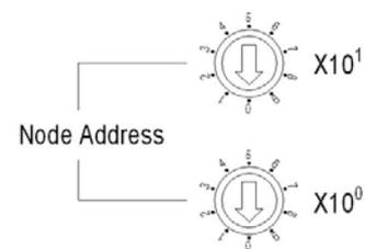
Example: If users want to set the communication address of AHRTU-DNET-5A to 26, they can turn the knob corresponding to  $x10^1$  to 2, and turn the knob corresponding to  $x10^0$  to 6.
