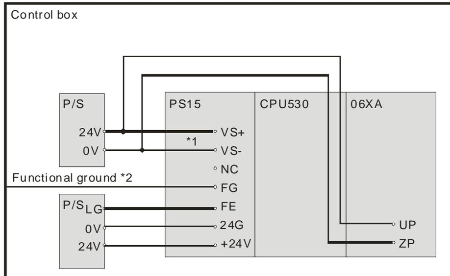
\*1. 24V on the external power supply is connected to VS+ and VS- on the power supply module. VS+ and VS- can be used to detect whether the voltage of the external power supply is stable.
