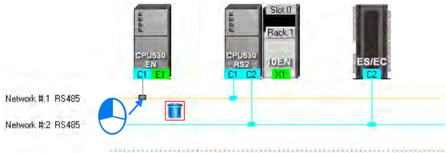
If the users release the left mouse button after they drag the connection point to the small picture representing a trash, the connection between the network and the port will be canceled.
