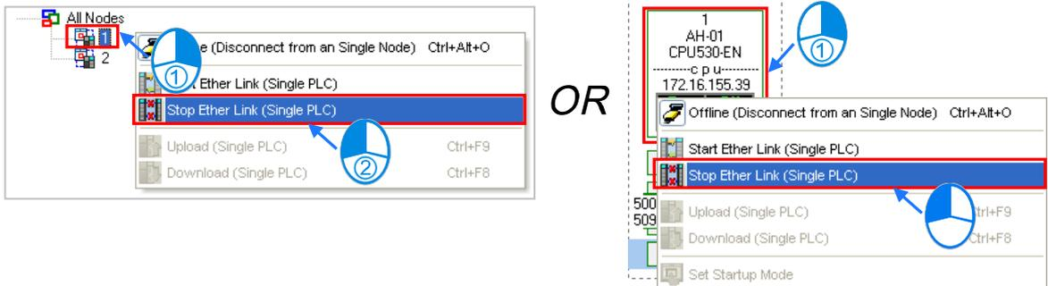
● **Making multiple nodes stop the execution of an Ether Link**
