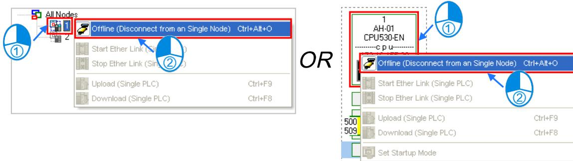
When the data demanding node selected is not monitored,
