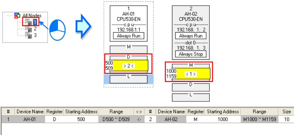
If a specific node on the node list is selected, the node in the display area will be selected. After the users select **All Nodes** on the node list, they can click the information about a node in the display area if they want to select the node. If the users click a device block in a node, the node will not be selected. After a node is selected, a dotted frame will appear.
