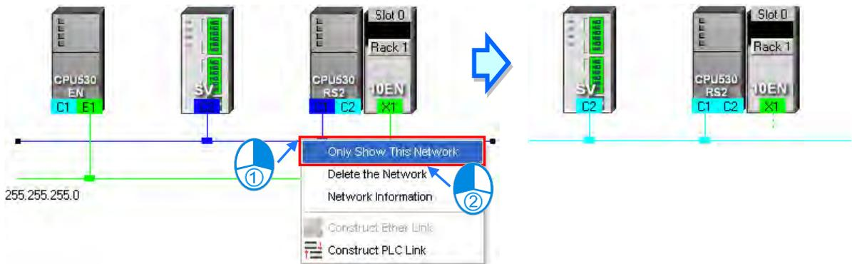
● **Hiding a network and the devices connected to the network**
