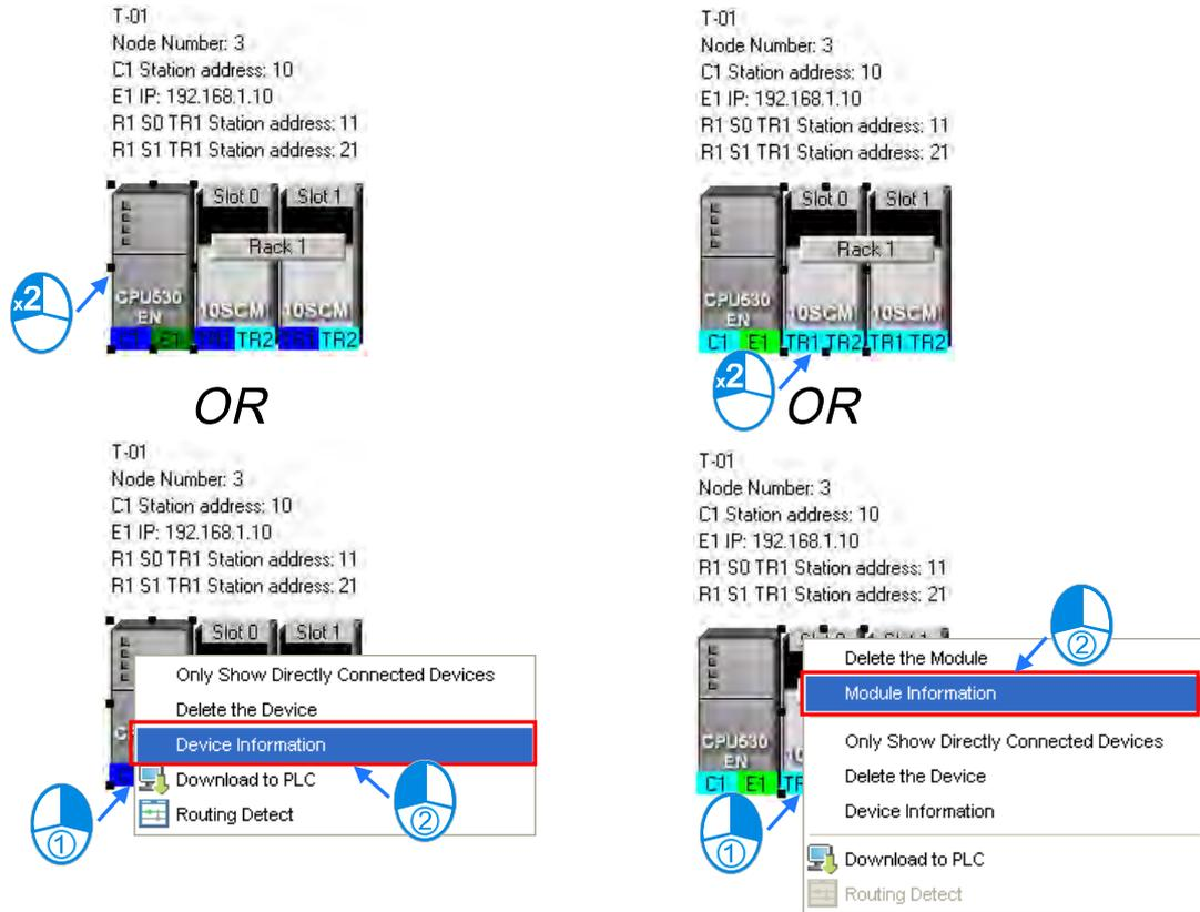
In the **Device Information** window, there are two tabs. The page displayed in the window depends on the device selected.
