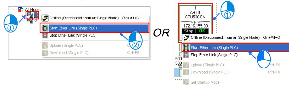
● **Making multiple nodes start the execution of an Ether Link**
