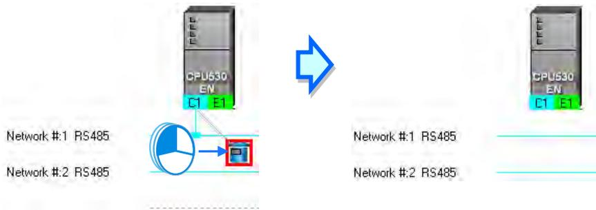
If the users drag the connection point to the dotted line, the system will connect the port to the new network added.
