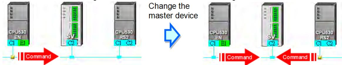
\* In addition to the conditions mentioned above, users have to prevent two devices or more than two devices from sending reading/writing commands simultaneously in any conditions.
