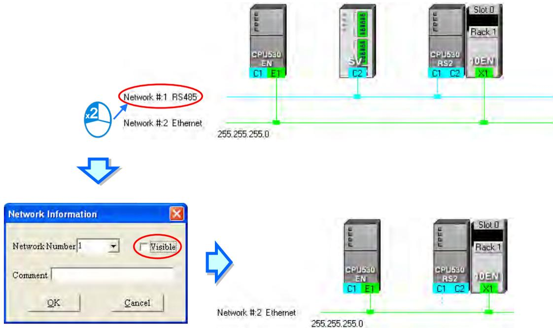
● **Hiding/Displaying the devices which are not connected to any networks**
