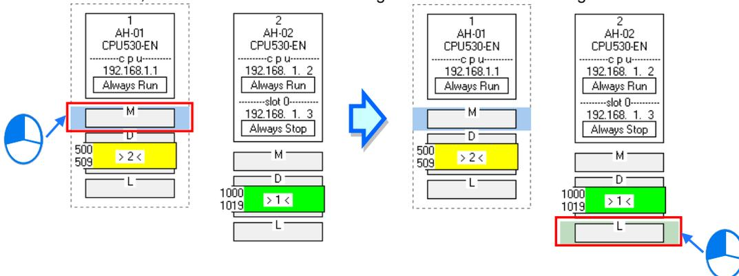
The users can click
