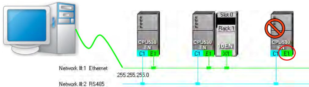
If the connection type that the driver selected uses is Ethernet, the system will carry out communication according to the IP addresses assigned to the devices in NWCONFIG. Before the communication is carried out, users have to make sure that the IP addresses actually assigned to the devices are the same as the IP addresses set in NWCONFIG, and the networks actually created are the same as the networks created in NWCONFIG. Otherwise, an error will occur if the communication is carried out.
