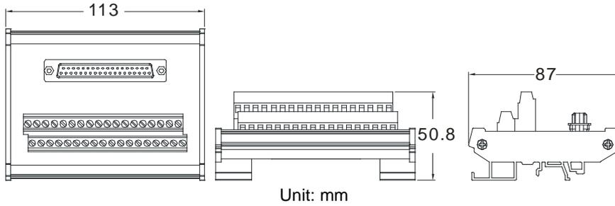
● Latch connector, I/O extension cable, and external terminal module
