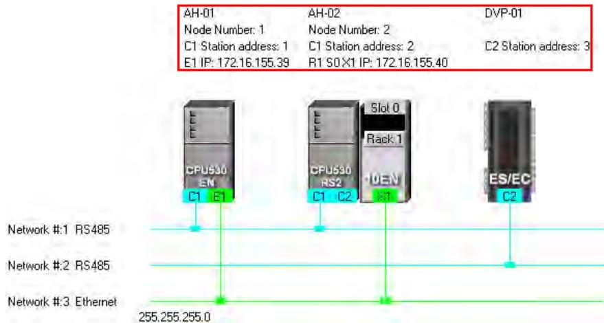
In addition to the information about the nodes, the network numbers assigned to the networks and the network types of the networks are shown. If a network is an Ethernet network, the subnet mask assigned to the ports connected to the network will be shown.
