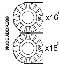
Example: If users need to set the node address of AHRTU-PFBS-5A to 26 (decimal value), they have to turn the knob corresponding to  $x16^1$  to "1" and the knob corresponding to  $x16^0$  to "A".
