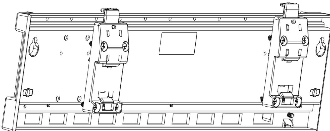
3. Install the backplane on a DIN rail.
