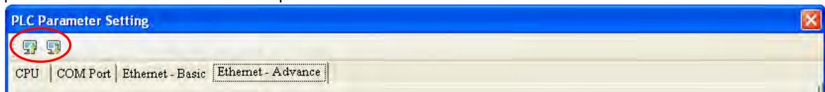
After the users select the **Ethernet-Advance** checkbox, and click **OK** in the **Transfer Setup** window, the parameters related to the **Ethernet-Advance** checkbox will be downloaded or uploaded, including the parameters related to the data exchange set in the previous section.
