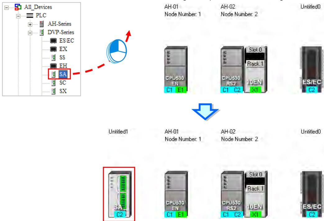
The users can add a user-defined Modbus device to the working area. After the users select **MODBUS Device** on the device list, and add it to the working area in one of the two ways described above, the **Custom Device** window will appear. The users have to type a name in the **Name** box, select a number in the **The number of ports** drop-down list box, and click **OK**. (A user-defined Modbus device can have three ports at most.)
