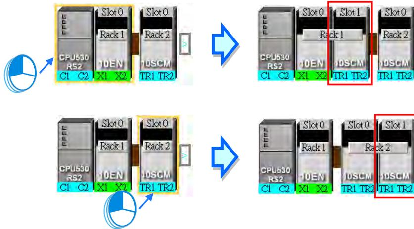
After the users drag an AH10SCM series module to
