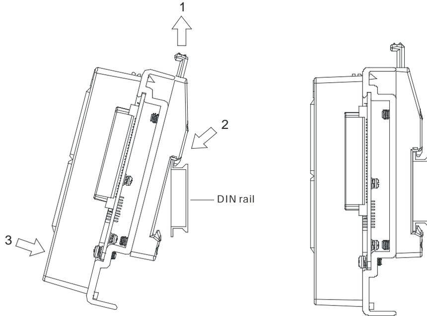
● **Removing a DIN rail**
