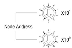
Example: If users want to set the communication address of AH10DNET-5A to 26, they can turn the knob corresponding to  $x10^1$  to 2, and turn the knob corresponding to  $x10^0$  to 6.
