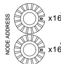
Example: If the station address of AH10COPM-5A is 16#26, users have to turn the knob corresponding to  $x16^1$  to position 2, and turn the knob corresponding to  $x16^0$  to position 6.
