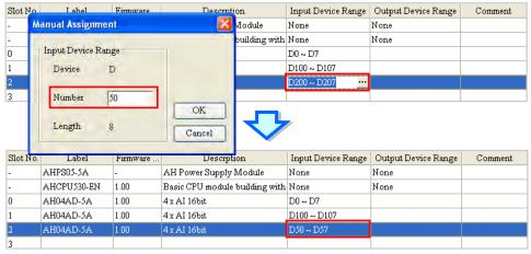
The input device addresses assigned to a module added follow D50~D57 rather than D100~D107. As a result, D58~D65 are assigned to AH04AD-5A which is installed in slot 3.
