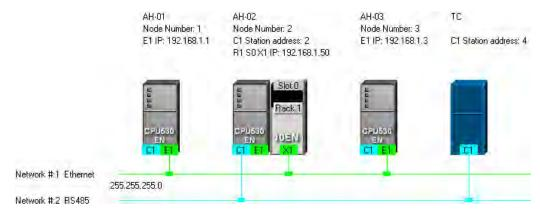
(5) Create a mechanism for data exchange performed by means of a PLC Link or an Ether Link. A PLC Link and an Ether Link operate independently. The users can create them in any order. The addresses involved in data exchange can not overlap, otherwise an error will occur after the data exchange is performed. It is recommended that the users should set addresses which are involved in data exchange according to the programs in the projects created.
