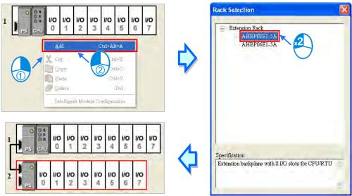
Right-click the left side of a rack, click **Add** on the context menu, and double-click an extension rack which will be added in the **Rack Selection** window. The extension rack will be under the rack.
