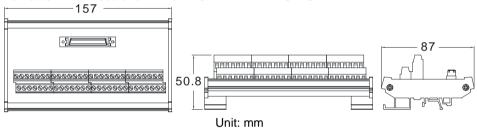
5. External terminal module for AH15PM-5A: DVPAETB-IO34C
