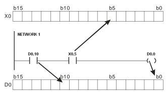
Users can access the state of DX0.0 and that of DY0.0 in a program. The state of DX0.0 and that of DY0.0 are not limited by scan time. They are refreshed immediately in a program.
