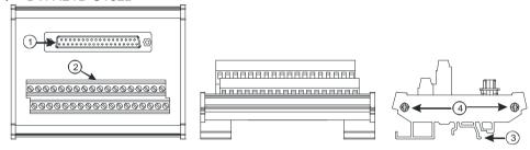
4. External terminal modules for AH32AN02P-5B
