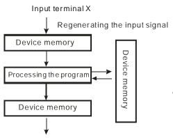
Regenerating the output signal and sending it to the output terminal
