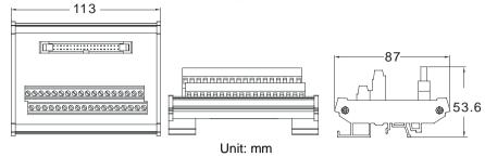
4. External terminal module for AH32AN02P-5C/AH64AN02P-5C: DVPAETB-OT32A
