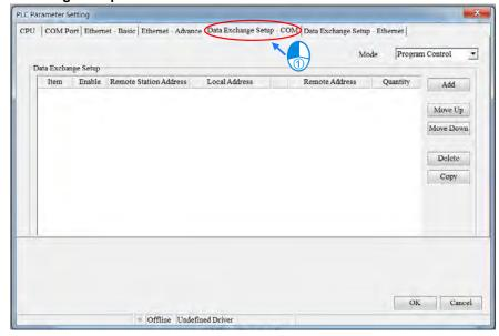
Owing to the fact that no data is set, there is a blank table in the **Data Exchange Setup** section. After **Add** is clicked, an item will be inserted. After the item is double-clicked, the **Item 1** window will appear.
