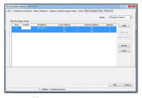
After the users click in the PLC Parameter Setting window, parameters set will be downloaded. After the users click in the upper left corner of the PLC Parameter Setting window, parameters in the PLC used will be uploaded.
