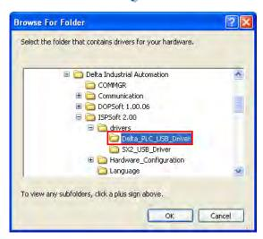
(4) After the correct driver is found in the folder denoted by the path, the system will install the driver. If the **Hardware Installation** window appears during the installation, please click **Continue Anyway**.
