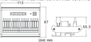
◆ External terminal module for AH32AN02P-5C/AH64AN02P-5C: DVPAETB-OR16B
