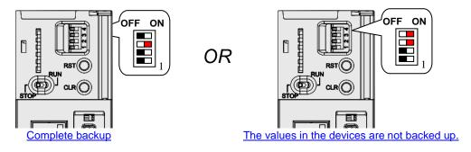
(2) Press the CLR button on the CPU module for five seconds. When the system backup is executed, the SYSTEM LED indicator blinks. After the system backup is complete, the SYSTEM LED indicator is OFF.
