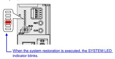
\* Whenever power is supplied to a CPU module, the system checks the state of DIP switch 2. If DIP switch 2 is turned ON, a system restoration is executed automatically. As a result, users must turn DIP switch 2 OFF after a system restoration is complete. In addition, the hardware configuration and the backplanes which are involved in a system restoration must be the same as those previously involved in the system backup in order to prevent an error from occurring.
