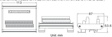
3. External terminal module for AH32AN02T-5C/AH64AN02T-5C: DVPAETB-OT32A
