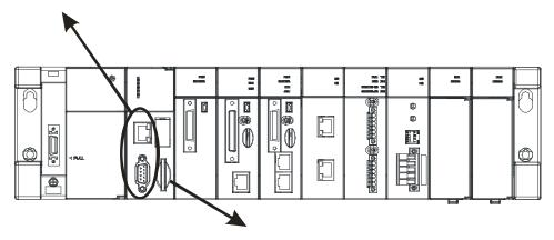
Users can restore or back up a system rapidly through the built-in SD interface in an AH500 series CPU module.
