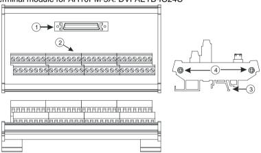
4. External terminal module for AH15PM-5A: DVPAETB-IO34C
