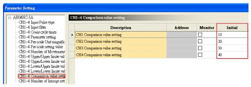
(3) After the users click **CH1~4 number of interrupt setting**, they can type interrupt numbers in the **Initial** cells. If the number of pulses received by a channel is the same as the comparison value set for the channel, the corresponding I/O interrupt will be executed. However, if no POU is assigned to the I/O interrupt, or the POU assigned to the I/O interrupt is not downloaded to the special high-speed module, an error will occur in the special high-speed module.
