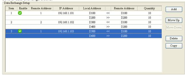
The users can manage the items in the table by means of the buttons at the right side of the table. The buttons are described below.
