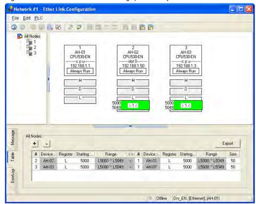
The figure below is a table related to data exchange performed by means of an Ether Link.
