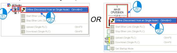
When the data demanding node selected is not monitored, on the toolbar is not pressed. If another node is monitored, will be pressed.
