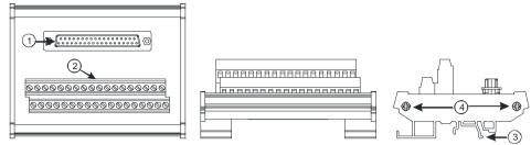
3. External terminal modules for AH32AN02T-5B
