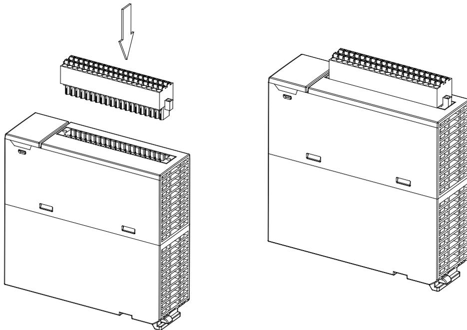
2. Press the clip in the direction indicated by the arrow. Secured the high-density terminal block with screws.
