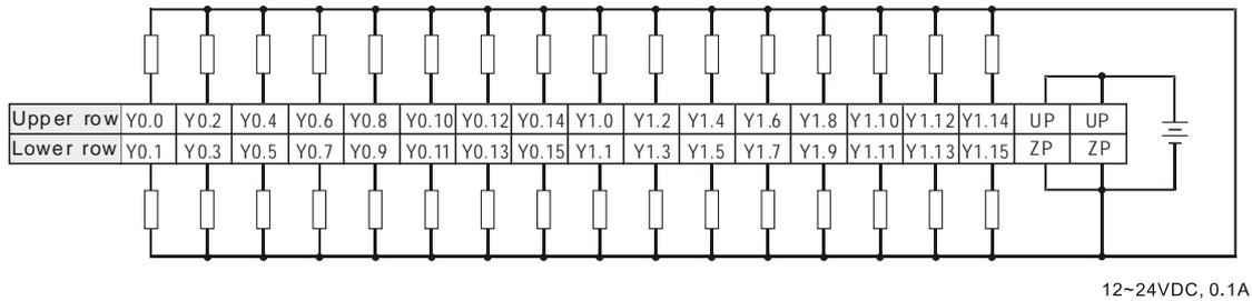
Wiring the external terminal module UB-10-OR32B:
