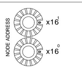
Example: If the station address of AH10COPM-5A is 16#26, users have to turn the knob corresponding to x16<sup>1</sup> to position 2, and turn the knob corresponding to x16<sup>0</sup> to position 6.
