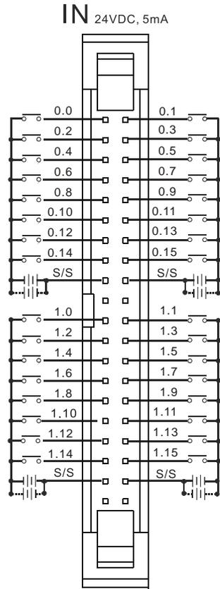
Wiring the external terminal module UB-10-ID32A:
