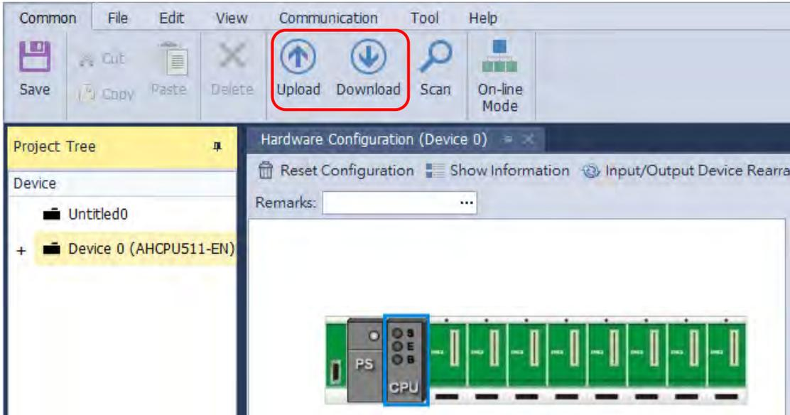
After the users select the **COM** checkbox under the tab of **HWCONFIG Data Exchange**, and click **Download**, the parameters related to the **COM** will be downloaded.
