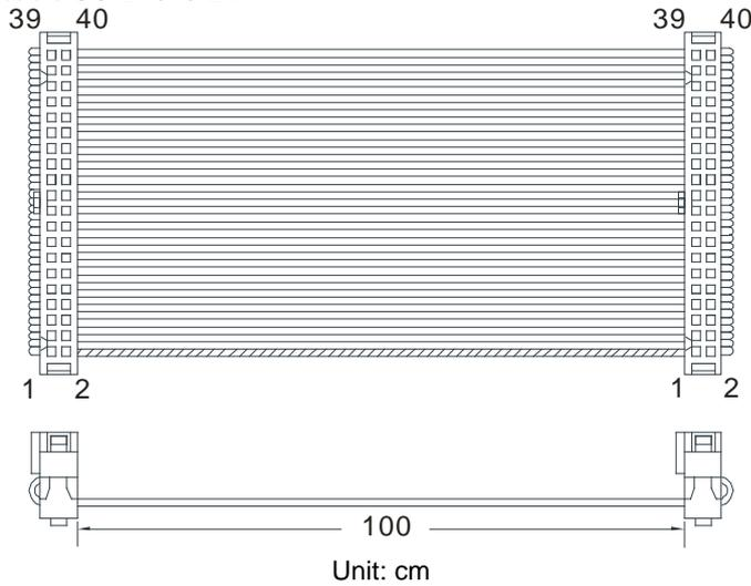
2. External terminal module for AH32AM10N-5C/AH64AM10N-5C: UB-10-ID32A
