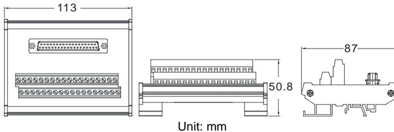
3. External terminal modules for AH32AN02T-5B
