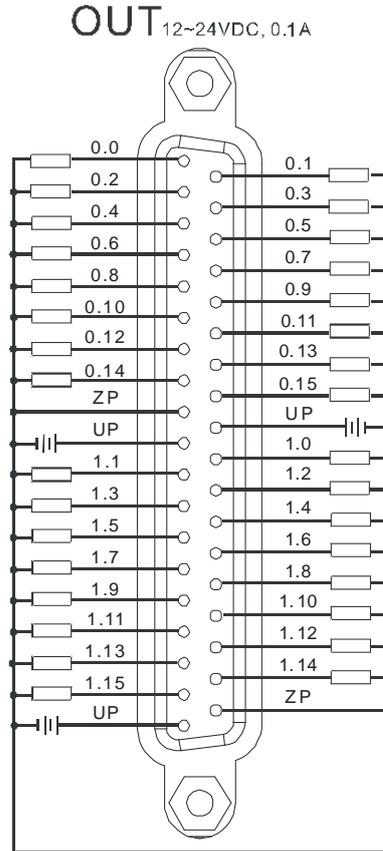
Wiring the external terminal module UB-10-OT32B:
