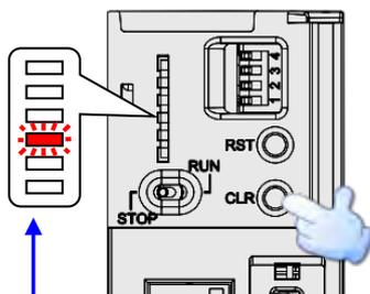
[When the system backup is executed, the SYSTEM LED indicator blinks.](#)
