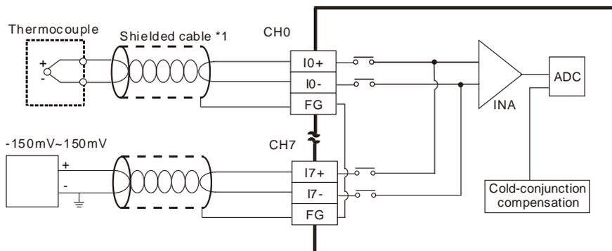
\*1. The cable connected to the input terminal should be the cable or the shielded twisted pair cable which can be connected to type J, type K, type R, type S, type T, type E, or type N thermocouple, and should be kept separate from other power cables and cables which generate noise.
