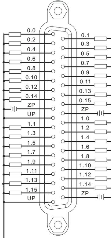
Wiring the external terminal module UB-10-OT32B:
