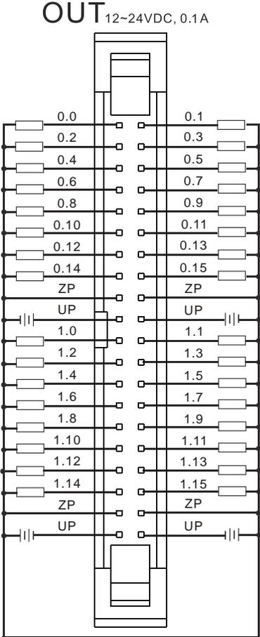
Wiring the external terminal module UB-10-OT32A:
