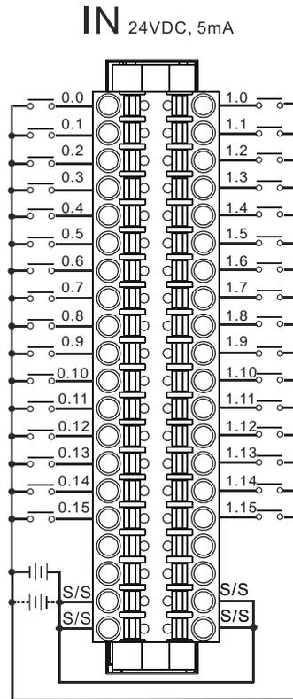
4.7.12 Wiring AH32AM10N-5B
