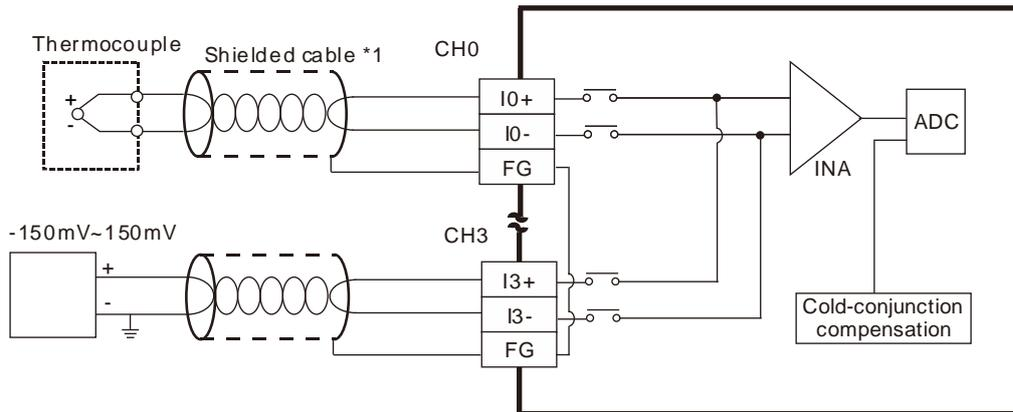
\*1. The cable connected to the input terminal should be the cable or the shielded twisted pair cable which can be connected to a type J, type K, type R, type S, type T, type E, or type N thermocouple, and should be kept separate from other power cables and cables which generate noise.
