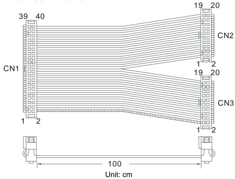
6. External terminal module for AH32AN02T-5C/AH64AN02T-5C: UB-10-OR16A
