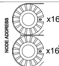
Example: If the node address of AHRTU-PFBS-5A is 26 (decimal value), users have to turn the knob corresponding to  $x16^1$  to position 1, and turn the knob corresponding to  $x16^0$  to position A.
