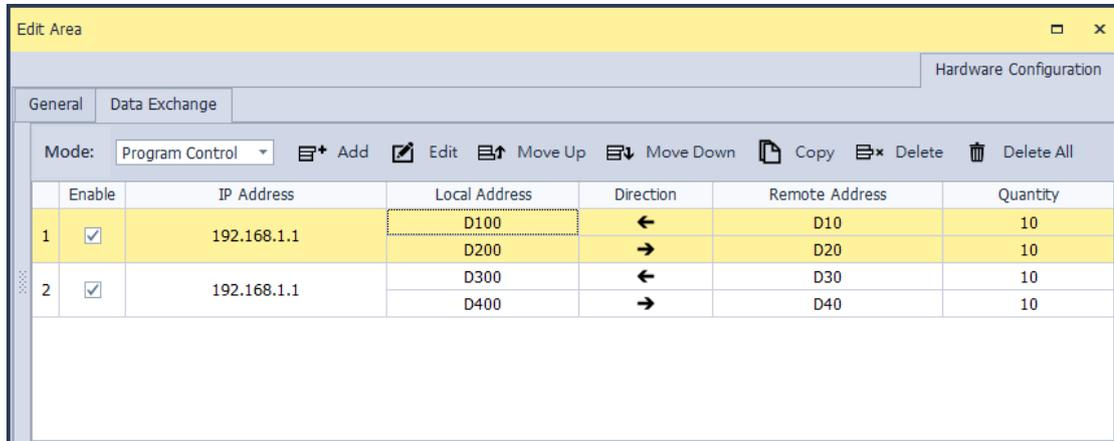
Users can manage the items in the table by using the function buttons on the top.
