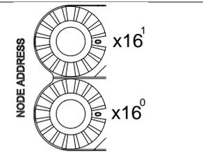
Example: If the node address of AH10PFBM-5A/AH10PFBS-5A is 26 (decimal value), users have to turn the knob corresponding to  $\times 16^1$  to position 1, and turn the knob corresponding to  $\times 16^0$  to position A.  $26$  (decimal value) =  $1A$  (hexadecimal value) =  $1 \times 16^1 + A \times 16^0$
