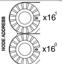
Example: If users need to set the node address of AHRTU-PFBS-5A to 26 (decimal value), they have to turn the knob corresponding to  $x16^1$  to "1" and the knob corresponding to  $x16^0$  to "A".
