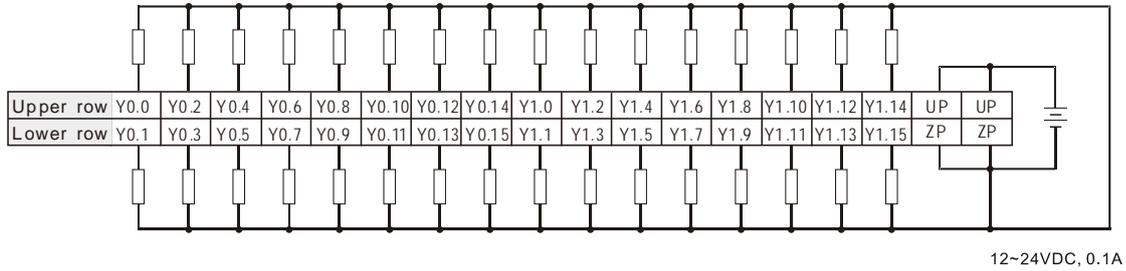
Wiring the external terminal module UB-10-OR16B:
