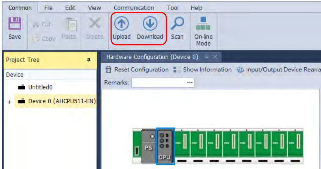
After the users select the **Ethernet** checkbox under the tab of **HWCONFIG Data Exchange**, and click **Download**, the parameters related to the **Ethernet** will be downloaded.
