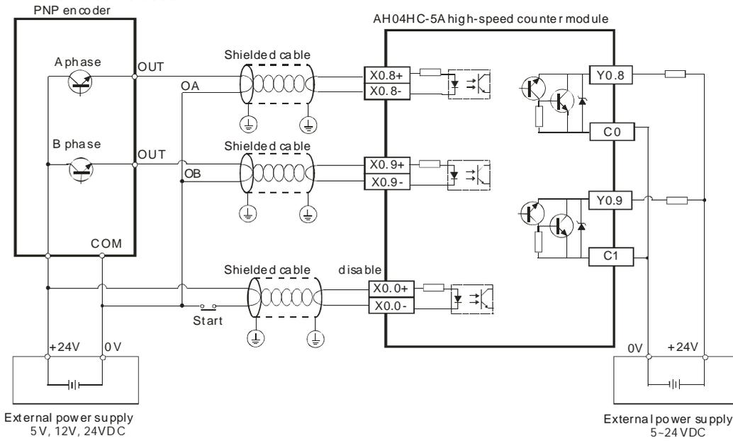
4.13.3.2 Wiring the Differential Input Terminals
