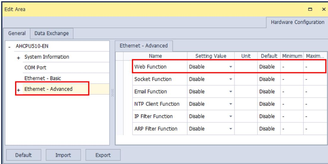
The screenshot shows the 'Edit Area' window for hardware configuration. The left sidebar shows a tree view with 'Ethernet - Advanced' selected. The main area displays a table of network functions:
