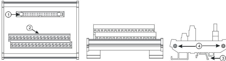
6. External terminal module for AH32AN02P-5C/AH64AN02P-5C
