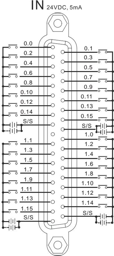
Wiring the external terminal module UB-10-ID32B:
