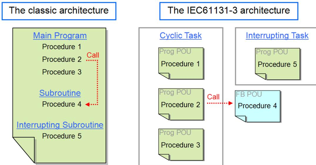
The figure below is a project created in ISPSOFT. Program 4 is a POU of the function block type. The cyclic programs and the interrupt program are POUs of the program type.
