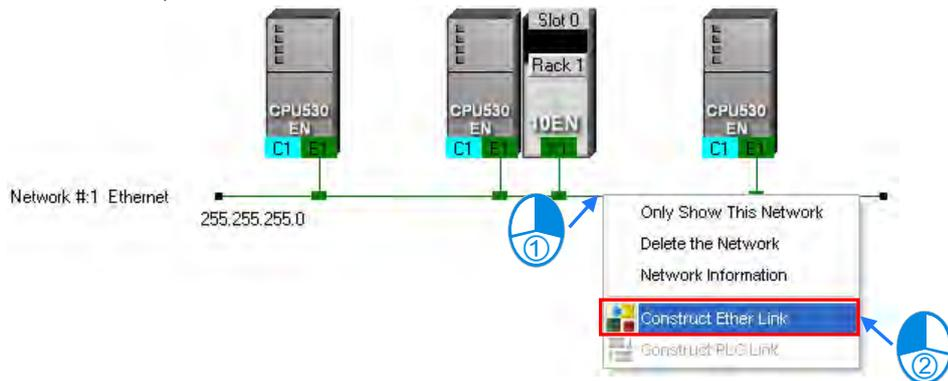
The **Ether Link Configuration** window is shown below.
