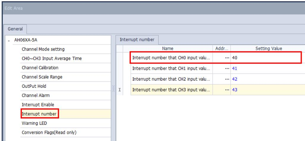
If an input signal received by input channel 0 exceeds the range, the external interrupt I40 will be triggered. However, if no POU is assigned to the external interrupt I40, or the POU assigned to the external interrupt I40 is not downloaded to the special high-speed module, an error will occur in AH06XA-5A.
