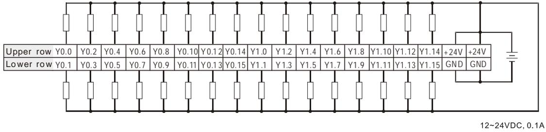
Wiring the external terminal module UB-10-OR16A:
