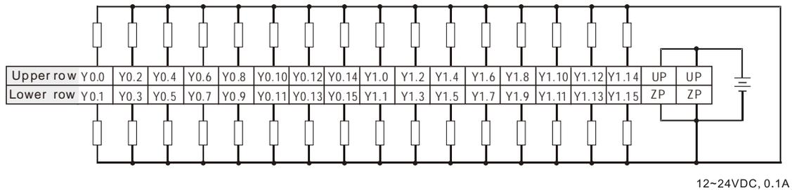
Wiring the external terminal module UB-10-OR16B:
