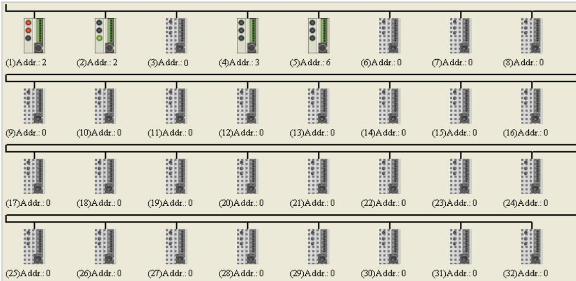
The small pictures in the monitoring area indicate the status of the main station rather than the statuses of the slave stations. The small pictures in the monitoring area are described below.
