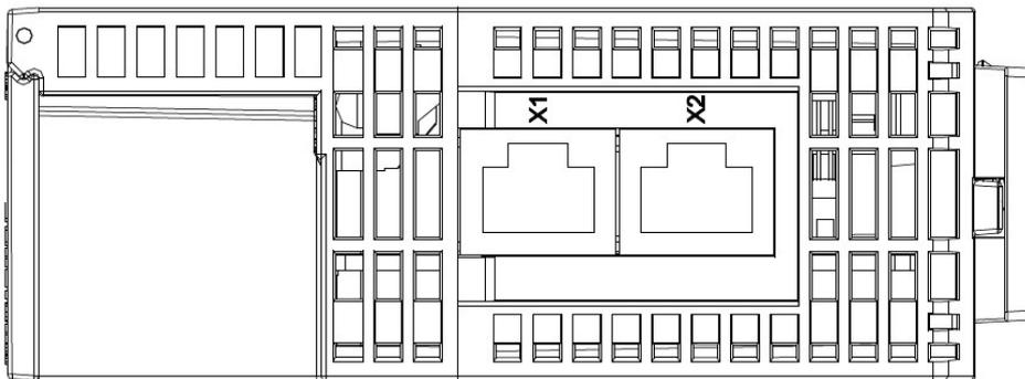
Note: when using port X1 or X2 to make a connection, do not create a loop; otherwise the communication between devices will fail.
