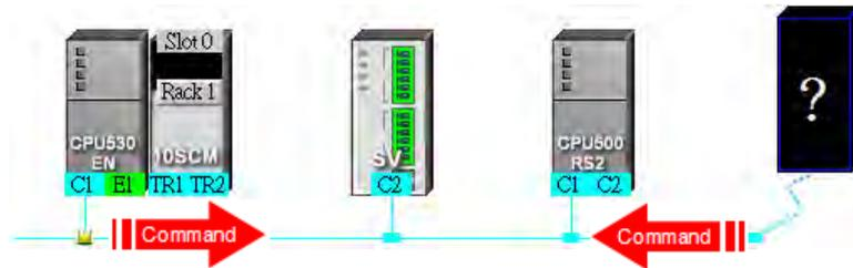
Besides, if the users do not set the parameters related to a PLC Link in the original master station again before they designate another device as a master station, an error occurs when more than one device sends reading/writing commands. As a result, if the users want to designate another device as a master station, they have to make sure that the original master station does not execute the original PLC Link.
