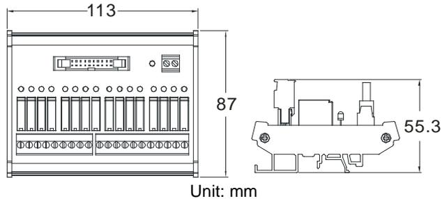
7. External terminal module for AH32AN02P-5C/AH64AN02P-5C: UB-10-OR16B
