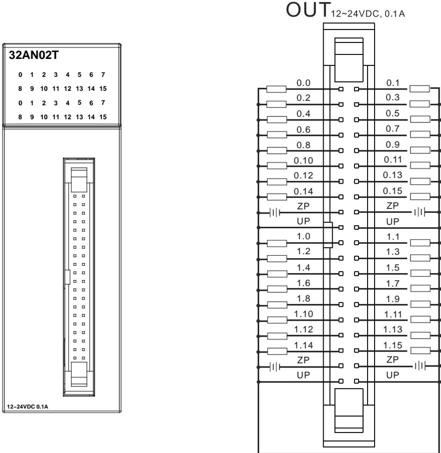
Wiring the external terminal module UB-10-OT32A:
