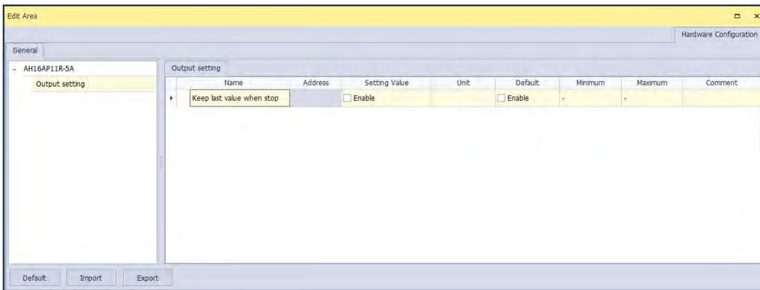
The hardware configuration is not complete until the parameters in the CPU module and AH16AP11R-5A are set. However, the configuration and the setting must be downloaded to the CPU module so that they can take effect. The configuration and the setting are saved here, and will be downloaded with the program in the project later.
