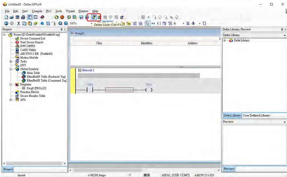
Step 2: Entering the debugging mode (PLC should be in the state of RUN)
