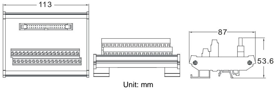
4. External terminal module for AH32AN02P-5C/AH64AN02P-5C: UB-10-OT32A
