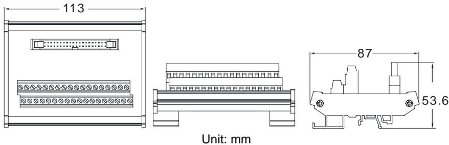
3. External terminal module for AH32AN02T-5C/AH64AN02T-5C: UB-10-OT32A
