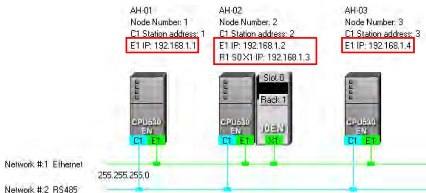
NWCONFIG can also carries out communication through routing.
