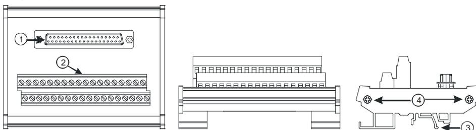
3. External terminal modules for AH32AN02T-5B
