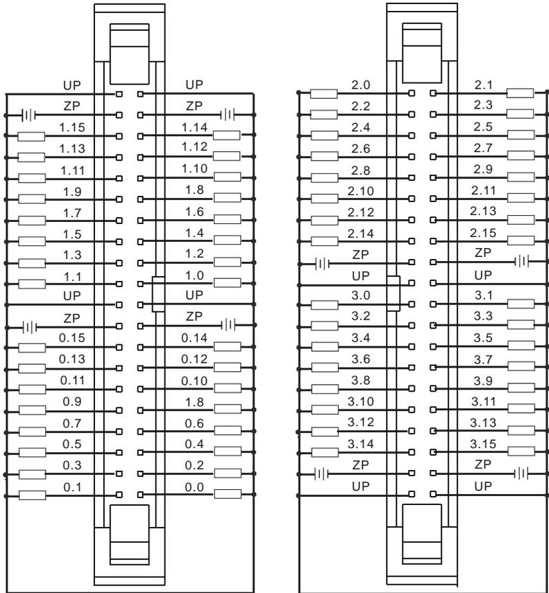
Wiring the external terminal module UB-10-OT32A:
