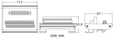
3. External terminal modules for AH32AN02T-5B
