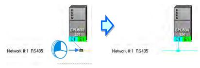
If the users move the mouse cursor to the dotted line while holding the left mouse button down, the port will connect to a network which matches the port.
