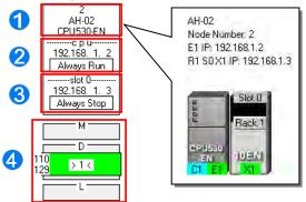
The information is composed of a node number, a PLC name, and a model name.
