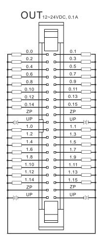
Wiring the external terminal module UB-10-OT32A:
