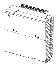
2. Press the clip in the direction indicated by the arrow. Secured the high-density terminal block with screws.
