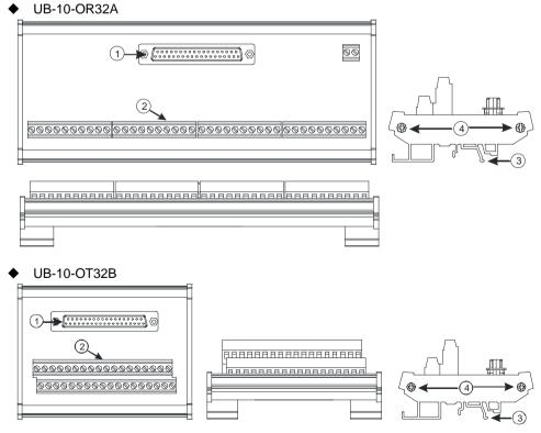
4. External terminal modules for AH32AN02P-5B
