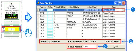
After users click the **Radix** cell for a device, they can select a method of representing the value in the device on the drop-down list.
