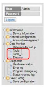
h. Note: The data monitor table must be downloaded to the device otherwise even if the data monitor table is created, it cannot be monitored.
