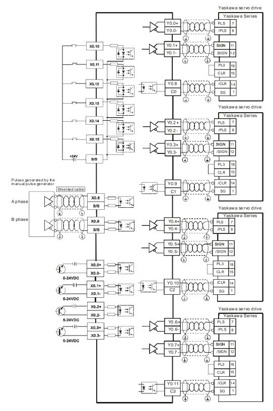
Wiring AH10PM-5A and an Yaskawa SGDV series servo drive
