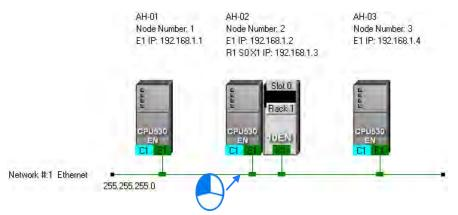
After the users click **Download to PLC** on the **PLC** menu, or **Download** window will appear. After the users select the **Routing Table** checkbox in the **Optional Download** window, and click **OK**, the routing tables produced will be downloaded to the nodes connected to the Ethernet network.
