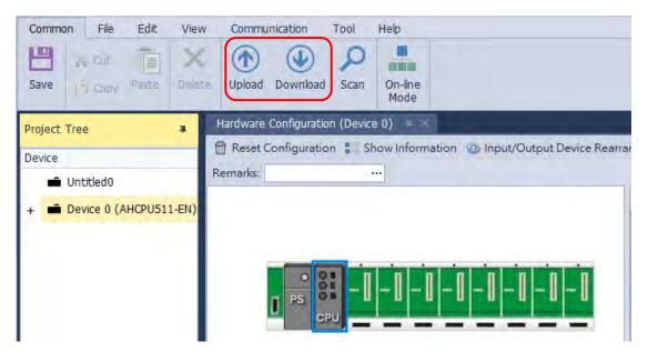
After the users select the **Ethernet** checkbox under the tab of **HWCONFIG Data Echange**, and click **Download**, the parameters related to the **Ethernet** will be downloaded.
