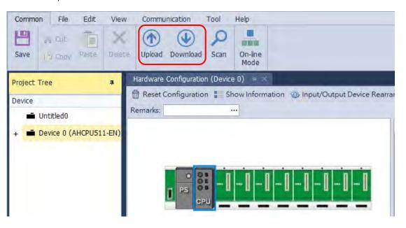
After the users select the **COM** checkbox under the tab of **HWCONFIG Data Echange**, and click **Download**, the parameters related to the **COM** will be downloaded.
