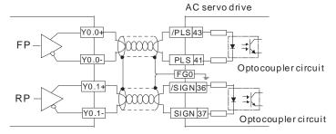
• Wiring differential output terminals on AH05PM-5A/AH10PM-5A/AH15PM-5A, and an ASDA-B series AC servo drive
