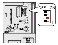
(2) Restore the power supply. After the system detects that DIP switch 2 is ON, the system restoration is executed. When the system restoration is executed, the SYSTEM LED indicator blinks. After the system restoration is complete, the SYSTEM LED indicator is OFF.
