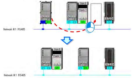
• Deleting a single device by means of a context menu
