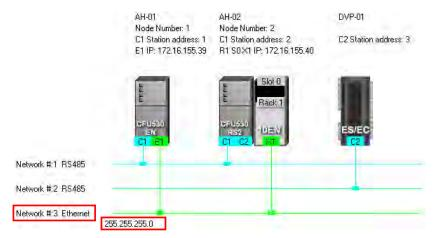
If the ports connected to an Ethernet network are not in the same domain, or are not assigned the same subnet mask, a warning sign will appear. If the ports connected to an Ethernet network are not assigned the same subnet mask, the strictest subnet mask will be shown.
