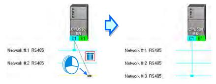
If the users release the left mouse button after they drag the connection point to another network which matches the port, the port will be connected to the network.
