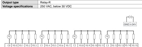
Wiring the external terminal module UB-10-OR16A:
