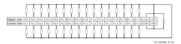
Wiring the external terminal module UB-10-OR16A:
