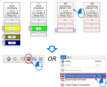
If the users want to delete all the asynchronous devices at the same time, they can click **Synchronize All Nodes** on the **Edit** menu, or **II** on the toolbar.
