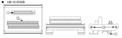
3. External terminal modules for AH32AN02T-5B
