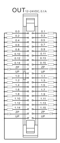
Wiring the external terminal module UB-10-OT32A:
