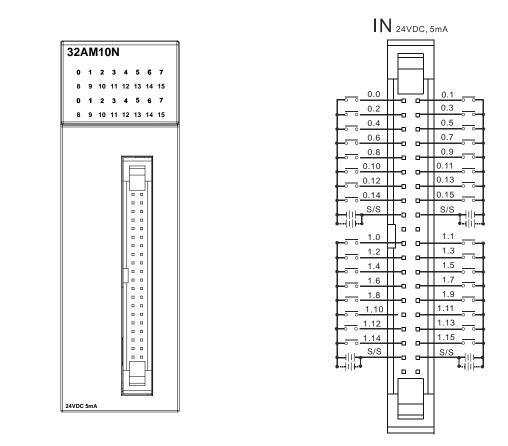
Wiring the external terminal module UB-10-ID32A: Upper row X0.0 X0.2 X0.4 X0.6 X0.8 X0.10 X0.12 X0.14 X1.0 X1.2 X1.4 X1.6 X1.8 X1.10 X1.12 X1.14 S/S S/S 1 Lower row X0.1 X0.3 X0.5 X0.7 X0.9 X0.11 X0.13 X0.15 X1.1 X1.3 X1.5 X1.7 X1.9 X1.11 X1.13 X1.15 S/S S/S Ī 24 V DC, 5 mA
