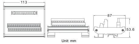
3. External terminal module for AH32AN02T-5C/AH64AN02T-5C: UB-10-OT32A
