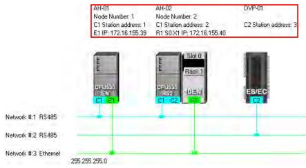
In addition to the information about the nodes, the network numbers assigned to the networks and the network types of the networks are shown. If a network is an Ethernet network, the subnet mask assigned to the ports connected to the network will be shown.
