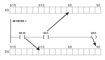
Users can access the state of DX0.0 and that of DY0.0 in a program. The state of DX0.0 and that of DY0.0 are not limited by scan time. They are refreshed immediately in a program.
