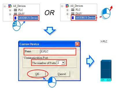
The users can add network modules to the working area. However, if the devices deployed in the working area include AH500 series CPU modules for which projects are created, the users can not connect network modules to the CPU modules. If the users want to connect network modules to the CPU modules, they have to close the NWCONFIG window, configure the network modules in HWCONFIG, and save the setting in HWCONFIG. After the users open the NWCONFIG window again, the system will update the network
