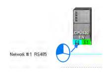
The users move the mouse cursor to the existing network while holding the left mouse button down. If the network matches the port, the port will connect to the network after the users release the left mouse button.
