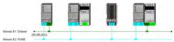
After the users click **Delete Selections** on the **Edit** menu, click **on** the toolbar, or press Delete on the keyboard, the objects selected will be deleted. However, the PLC for which a project is created and the modules connected to the PLC can not be deleted. Besides, if a PLC is deleted, the modules connected to the PLC will also be deleted.
