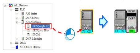
If the PLC does not support the network module selected, the mouse cursor becomes (2).
