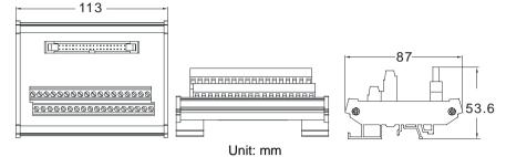
4. External terminal module for AH32AN02P-5C/AH64AN02P-5C: UB-10-OT32A
