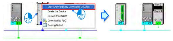
Only displaying the devices connected to a network
