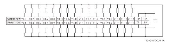
Wiring the external terminal module UB-10-OR16B:
