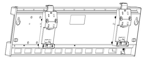
Install the backplane on a DIN rail.
