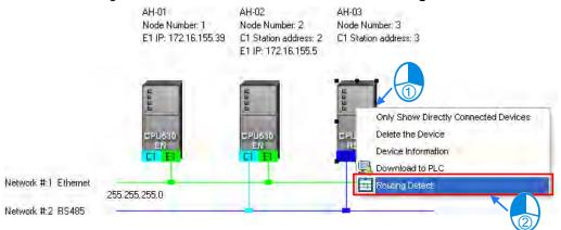
(3) After Routing Detect is clicked, the display of the network architecture in the working area will change, and the Routing detect status window will appear. The way in which the node which is designated as the first station is connected to the computer is also shown in the working area. Please see the red circle in the figure below.
