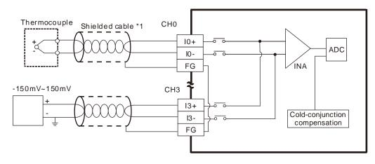
\*1. The cable connected to the input terminal should be the cable or the shielded twisted pair cable which can be connected to a type J, type K, type R, type S, type T, type E, or type N thermocouple, and should be kept separate from other power cables and cables which generate noise.
