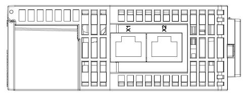
Note: when using port X1 or X2 to make a connection, do not create a loop; otherwise the communication between devices will fail.
