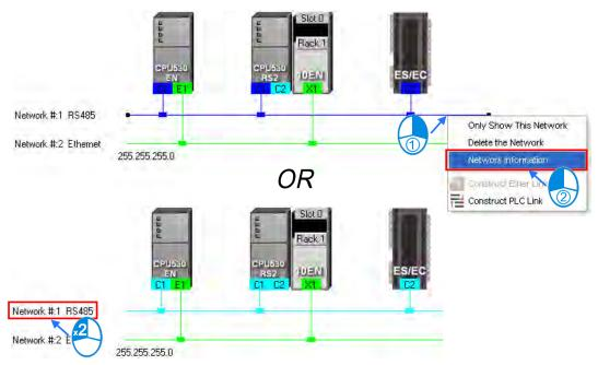
In the **Network Information** window, the users can select a network number which is not assigned to any network in the **Network Number** drop-down list box. Besides, the users can type a comment in the **Comment** box. After the users complete the setting of the attributes of the network, and click **OK** in the **Network Information** window, the attributes of the network will be updated immediately.
