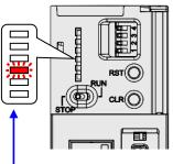
When the system restoration is executed, the SYSTEM LED indicator blinks.
