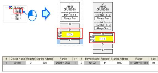
If a specific node on the node list is selected, the node in the display area will be selected. After the users select **All Nodes** on the node list, they can click the information about a node in the display area if they want to select the node. If the users click a device block in a node, the node will not be selected. After a node is selected, a dotted frame will appear.
