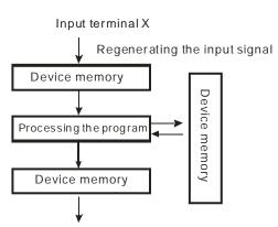
Regenerating the output signal and sending it to the output terminal
