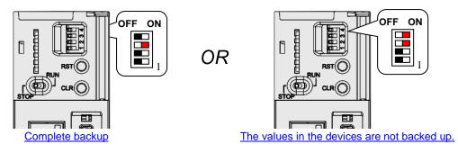
(2) Press the CLR button on the CPU module for five seconds. When the system backup is executed, the SYSTEM LED indicator blinks. After the system backup is complete, the SYSTEM LED indicator is OFF.
