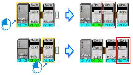
After the users drag an AH10SCM series module to at the right side of a node, an extension rack will be added to the node.
