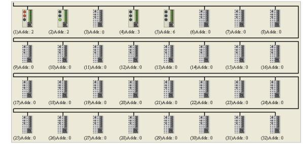
The small pictures in the monitoring area indicate the status of the main station rather than the statuses of the slave stations. The small pictures in the monitoring area are described below.
