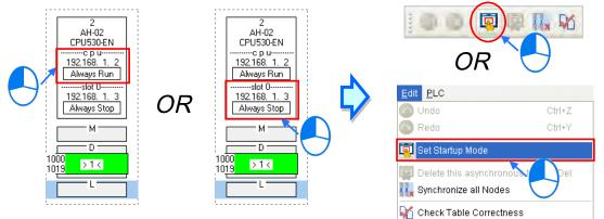
After the users use one of the methods described above, the Starting Mode Setup window will appear. The page displayed in the window varies with the information selected. The users can click the tabs in the window. Select a mode in the **Start Mode** drop-down list box. If **SM Flag** is selected, the users can select an initial state in the **Download State** drop-down list box. After an initial state is selected, the users can click **OK**.
