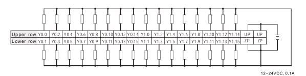
Wiring the external terminal module UB-10-OR16B:
