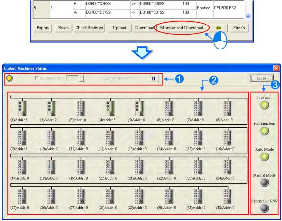
**1** Setting area: The users can set the PLC Link constructed.
