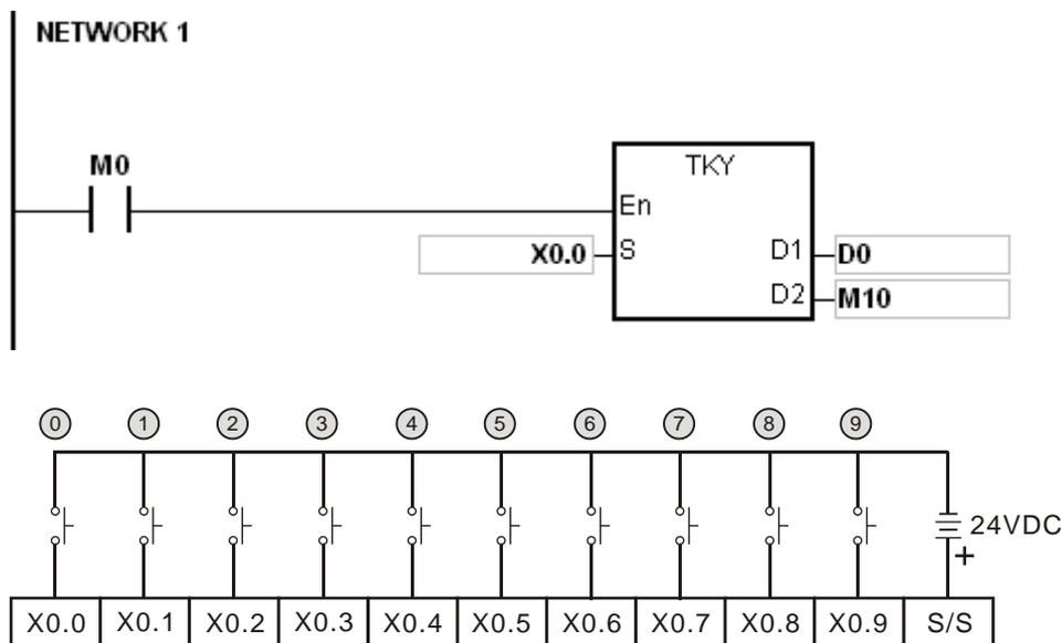
Note: The digital input module AH16AM10N-5A is used in this example.
