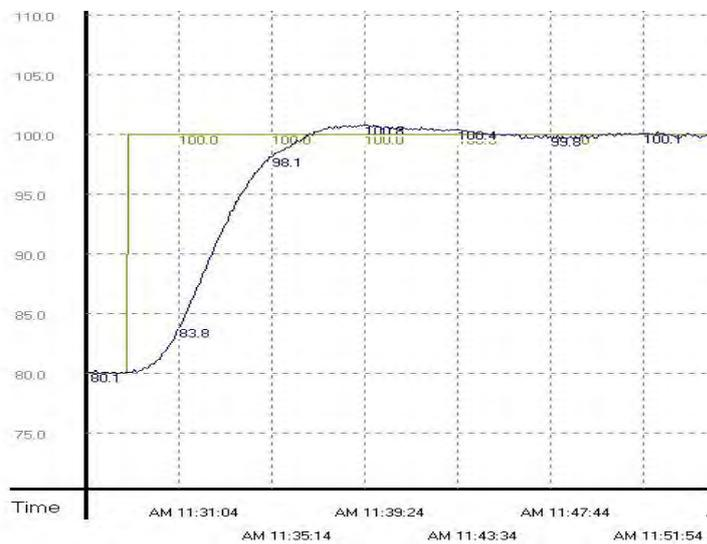
This graph shows that when the target temperature changes from 80°C to 100°C, the automatically tuned parameters still work to control the temperature in a reasonable amount of time.
