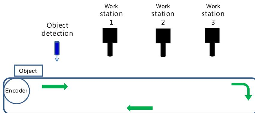
**Step 1:** use the input point X0.4 as the object detection interrupt, HC202 as the high-speed counter for the encoder and output point Y0.0 as the first output point for the work station.
