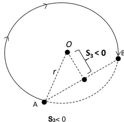
5. The figures below show 2 arc-travel path examples (solid lines) when the point B is in Quadrant I and IV with different setting values in  $S_3$  (shift the central angle). ( $r$ : radius)
