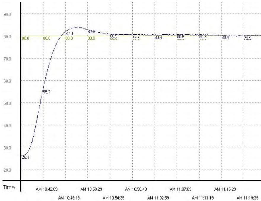
This graph shows that using automatically tuned parameters can result in a good temperature control result. It only takes about twenty minutes to control the temperature. The following graph shows the result of changing the target temperature from 80°C to 100°C.
