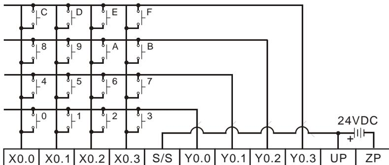
Note: The transistor output module AH16AP11T-5A is used in this example.
