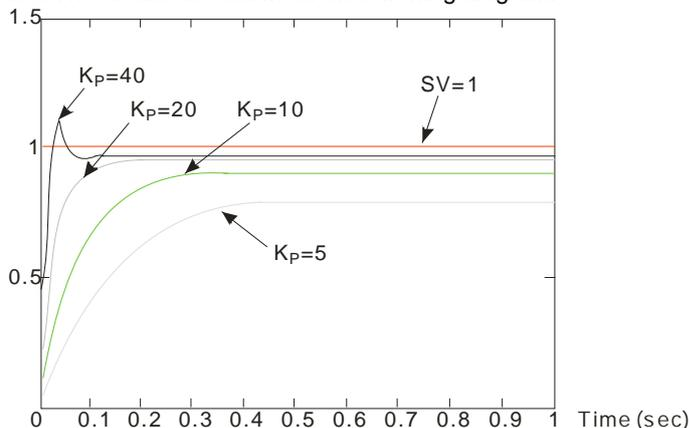
**Step 2:** When the  $K_P$  is 40, there is overreaction. When the  $K_P$  is 20, the reaction curve of PV is close to SV, and there is no overreaction. However, due to the fast start-up, the transient output value (MV) is big. Neither 40 nor 20 is a suitable value. When the  $K_P$  is 10, the reaction curve of PV approaches SV smoothly. When  $K_P$  is 5, the reaction is too slow. Therefore,  $K_P = 10$  is the best choice.
