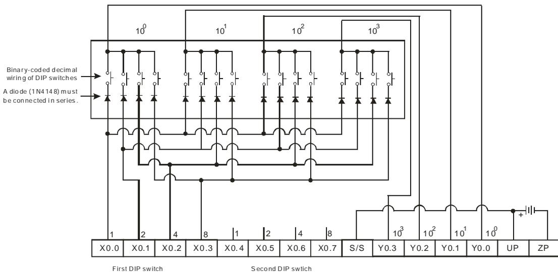
Note: The transistor output module AH16AP11T-5A is used in this example.
