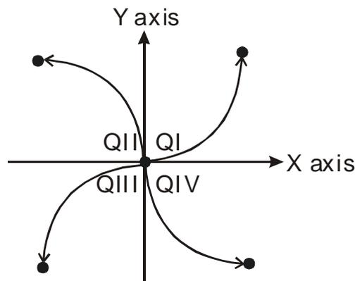
3. Since the distances between the starting positions and the target positions in the X and Y axes are not the same, and the travel path will be formed by a 90 degree arc of an ellipse. This function is useful for applications that draw elliptical arcs.
