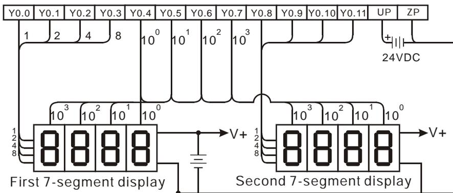
Note: The transistor output module AH16AN01T-5A is used in this example.
