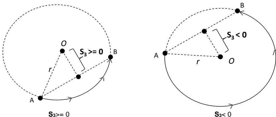
5. The figures below show 2 arc-travel path examples (solid lines) when the point B is in Quadrant I and IV with different setting values in  $S_3$  (shift the central angle). ( $r$ : radius)
