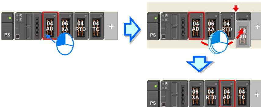
\* When rearranging the module position, the input/output device range, comment, internal parameters, corresponding device D and advanced parameters for intelligent modules are also rearranged with the module.
