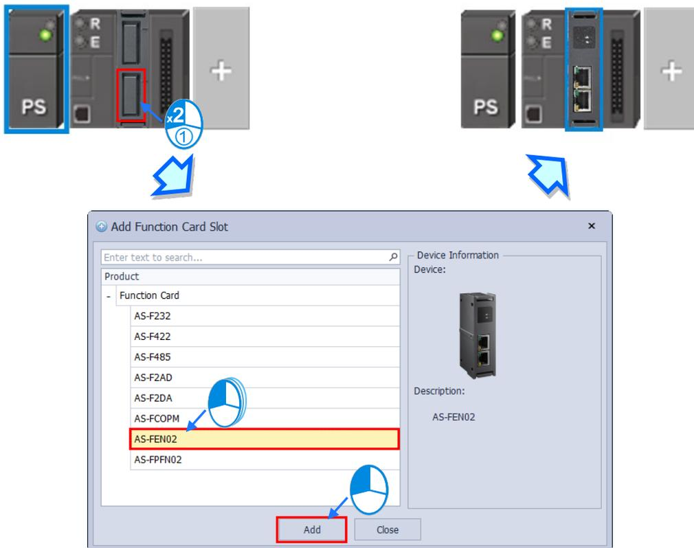
You can also set AS-FEN02 card in the Edit Area. Set AS-FEN02 as **Manual Select Card** (Note: If AS-FEN02 card is selected from **Manual Select Card**, then Function Card 1 cannot be set.) After that you can set up Ethernet communication parameters.
