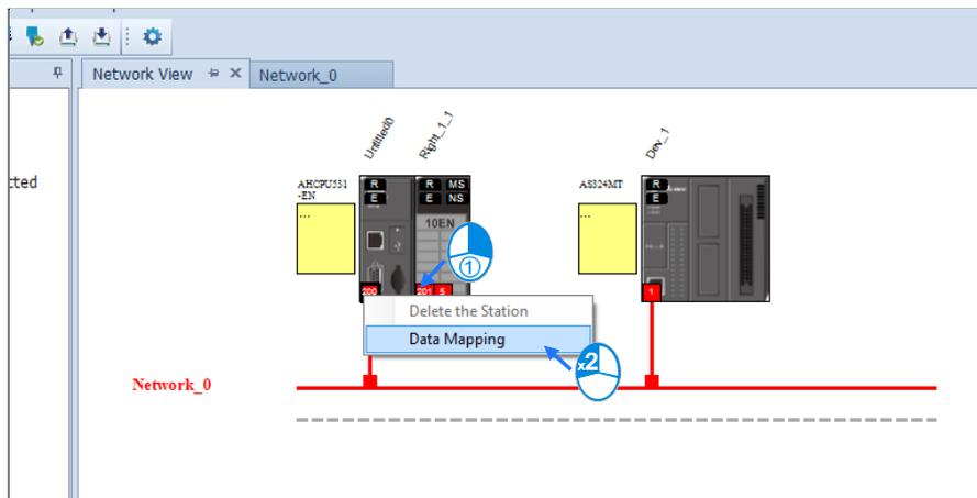
The system creates a Data Mapping Tab, shown for Network\_0.
