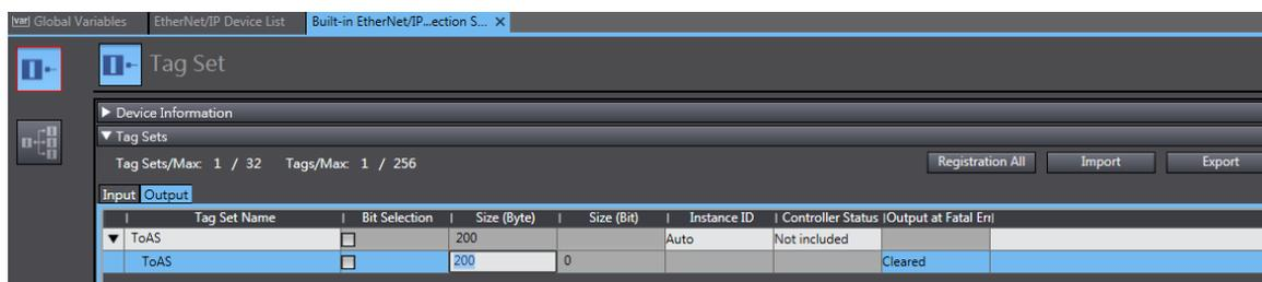
10. Click **Controller** and then **Synchronize...** from the menu bar to synchronize the setting with OMRON Scanner.
