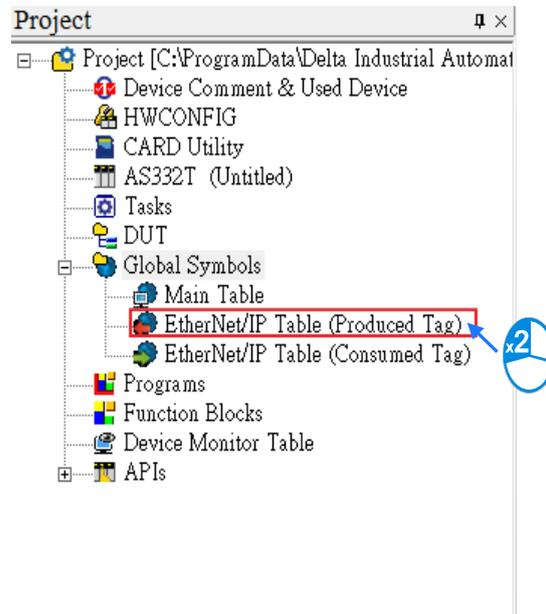
2. Double-click **EtherNet/IP Table (Produced TAG)** to create a Produced TAG.
