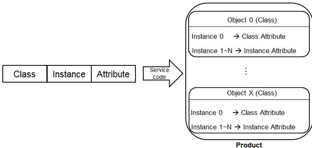
You can use API 2208 EIPRW instruction or explicit messages to read / write objects. The supported EtherNet/IP objects are listed in the following table. Refer to Section 9.8.2 for the data type definitions. Refer to Section 9.8.3 ~ 9.8.19 for object contents.
