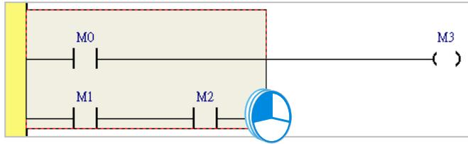
To select several networks, press and hold the Ctrl key on the keyboard and click the networks. You can also select a range of networks by pressing and holding Shift on the keyboard, clicking the first network within the range, and then clicking the last network within the range.
