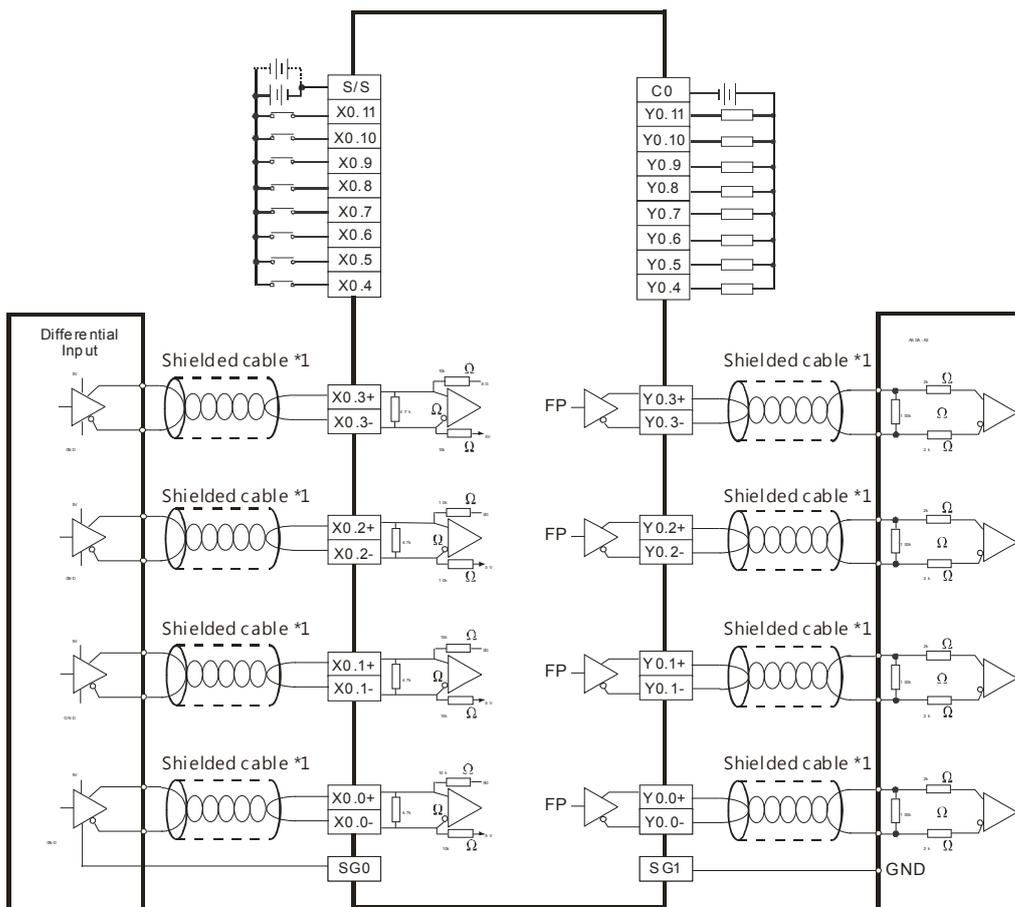
● Wiring the External Terminal Module UB-10-ID16A
