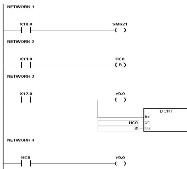
1. X10.0 drives SM621 to determine counting direction (up/down) of HC0.
