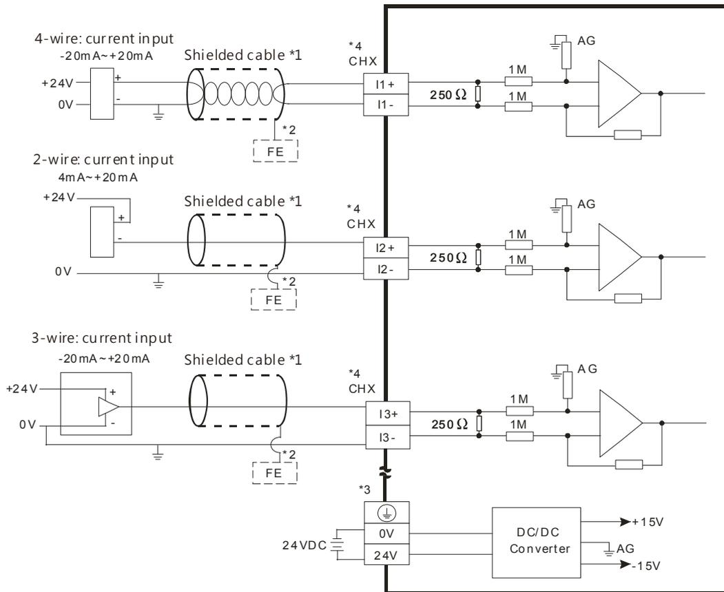
\*1. Use shielded cables to isolate the analog input signal cable from other power cables.
