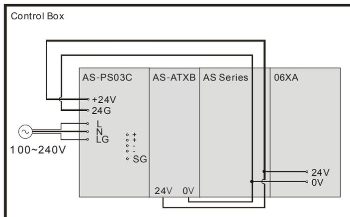
\*1. The live wire and the neutral wire in the AC power cable are connected to L and N on the power supply module respectively. To prevent incorrect system operation, the ground in the AC power cable must be connected to LG on the power supply module.
