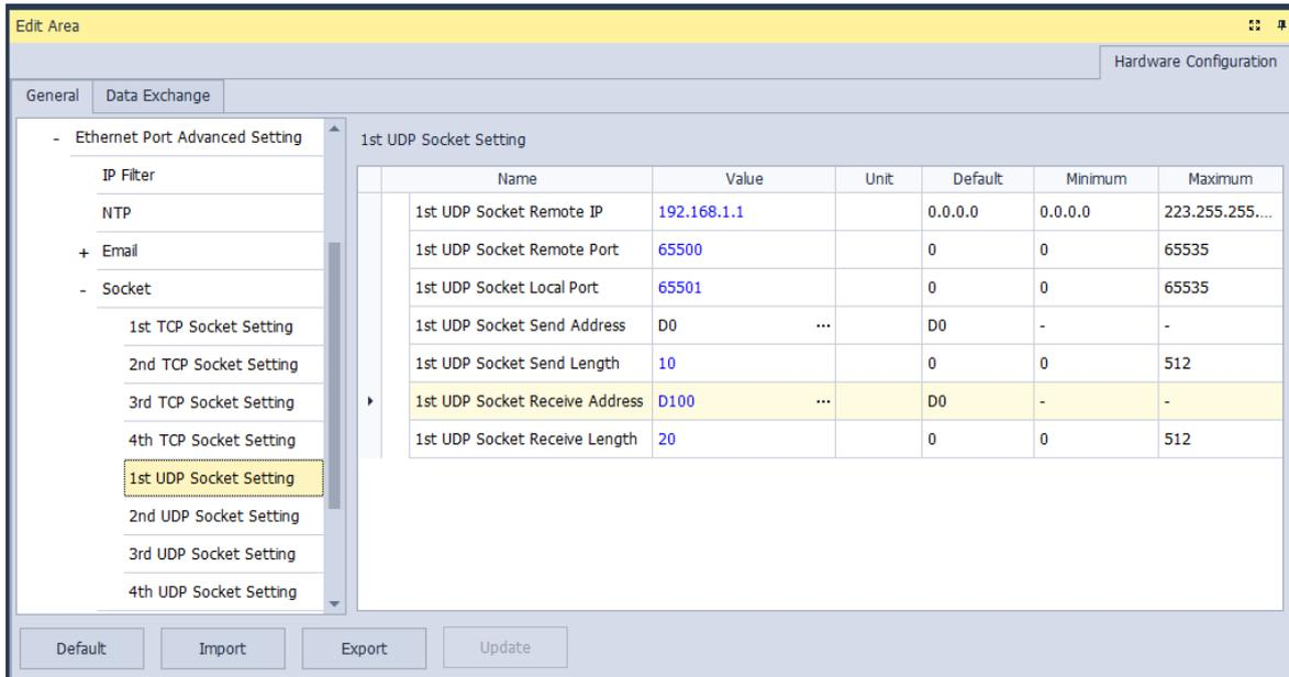
The parameters in the **TCP Socket Setting** are the same as the parameters in the **UDP Socket Setting** except that there is no **Keep Alive Timer** parameter in the UDP Socket Setting. The parameters in the TCP and UDP Socket Setting are described below.
