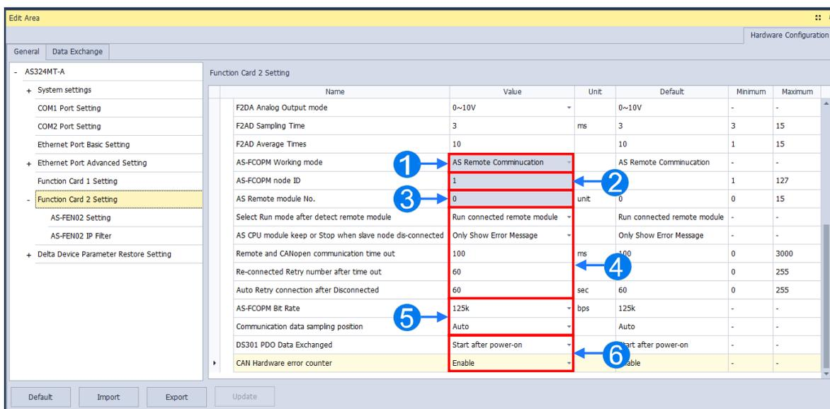
❶ Select AS Remote Control/Delta Servo Drives and AS Remote Module/CANopen DS301 from the **AS-FCOPM working mode** box. The AS Remote Module and Delta Servo Drives adopts communication protocols exclusive to Delta servo products and AC motor drives. In addition, the AS Remote Module and Delta Servo Drives are also applied in connecting remote I/O AS series as well as CANopen DS301 for the application of DS301 standard protocol.
