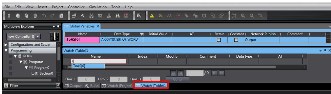
Modify the values according to the display format. Make sure the value in the **Online Value column** is the same as the value in the **Modify column**.
