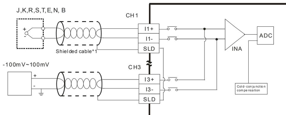
\*1. The cable connected to the input terminal should be the cable or the shielded twisted pair cable connected to a type J, K, R, S, T, E, N, B thermocouple. It should be kept separate from other power cables and cables that generate noise.
