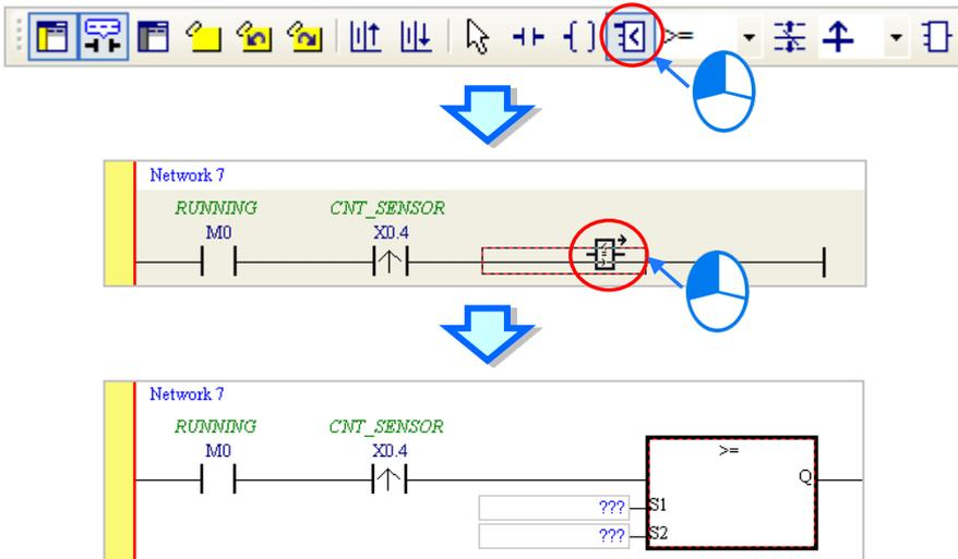
Write the program shown below. In ISPSOft, K precedes a decimal value and H precedes a hexadecimal value. To type a decimal value in ISPSOft, type it directly. To type a hexadecimal value in ISPSOft, type "16#" and the hexadecimal value; e.g. 16#7FFF. In ISPSOft, 8# precedes an octal value, and 2# precedes a binary value.
