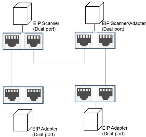
When a switch is needed for the particular topology, the switch should support the DLR function. If not, the connection might fail.
