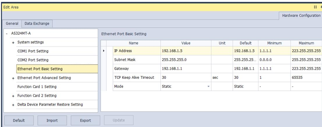
**Mode** sets the addressing mode of the IP of the CPU module.
