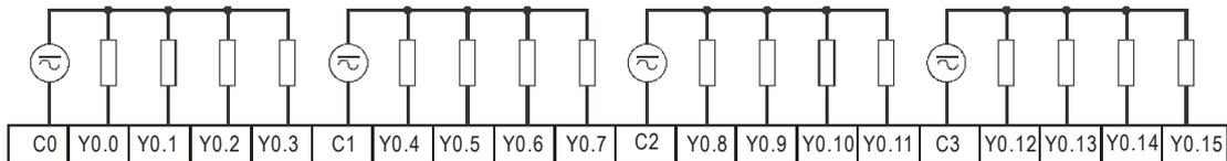
Note: UB-10-OR16A can be used with AS Series and DVP Series. The indications on the UB-10-OR16A board is for DVP Series. For the definitions of terminal connections for AS Series, you can see the reference table below. Or refer to the enclosed sticker for AS Series.
