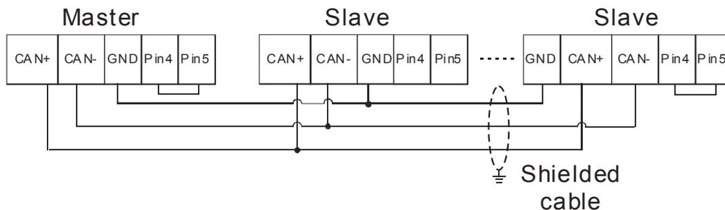
1. It is recommended to use Daisy Chain for connection and be sure to use terminal resistor in the beginning and the end of the terminal arrangement.
