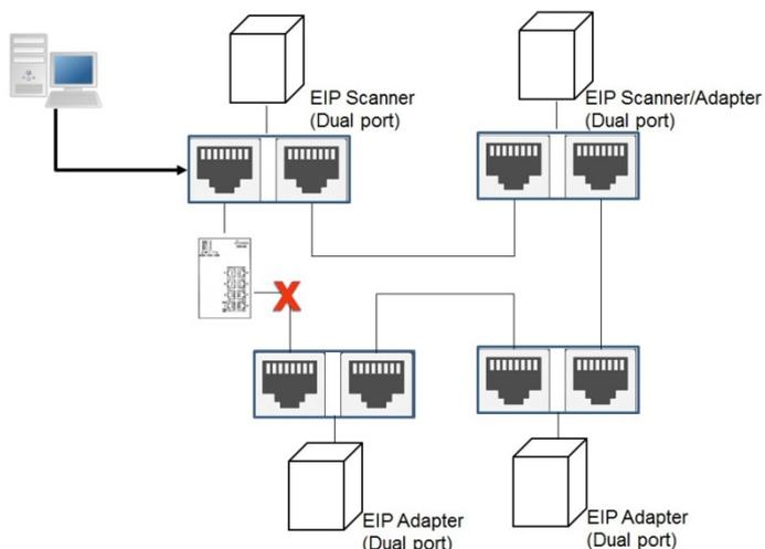
Alternatively, you can use an EIP tap to connect your PC so that the ring topology stays intact.
