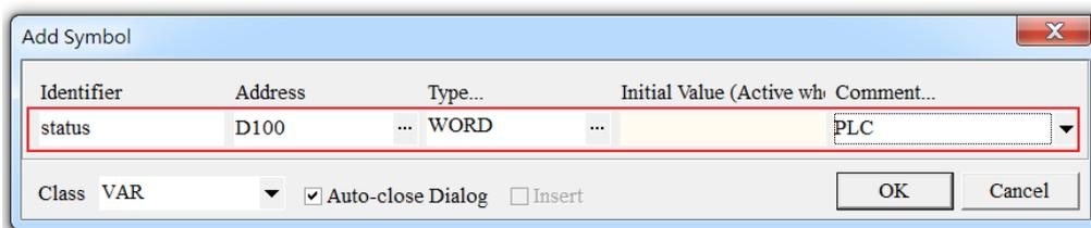
After the settings are complete, download the TAG to the PLC. Other EIP devices can access the Produced TAG with their Consumed TAG. For information on creating a Consumed TAG, refer to the EIP device manual.
