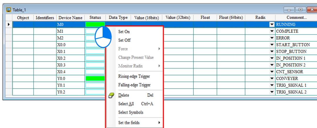
You can test and debug the program you created in this chapter through the monitoring table you created in this section. Refer to Chapter 18 in the ISPSOFT User Manual for more information about testing and debugging a program.
