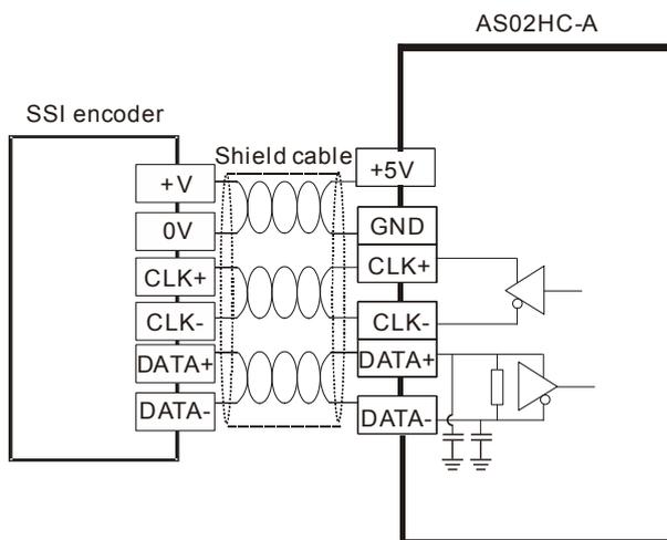
Note: The power supply of the SSI encoder you are using may NOT be 5 VDC, check for the actual power supply of your SSI encoder.
