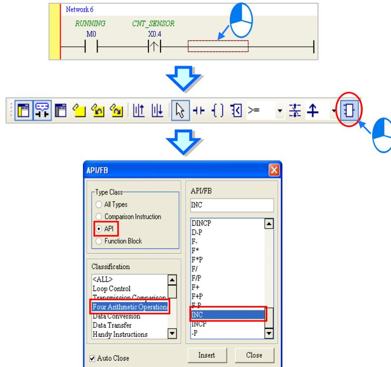
After you insert the instruction, assign a device address to the operand, and write the program shown below.
