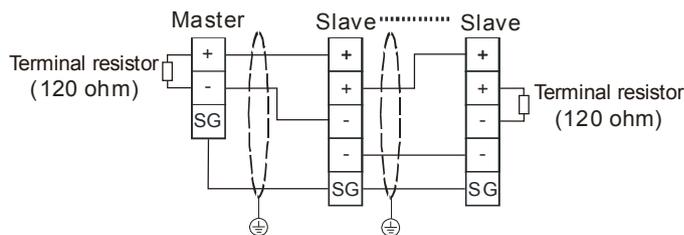
There are two sets of terminals + and – on the RS485 port of AS-PC03C; instead of connecting the signal cable to the same terminal, connecting to the next slave can be through the terminal + and - directly. And when AS-PS03C acts as the last slave, the terminal + and – can be used to connect to the terminal resistor.
