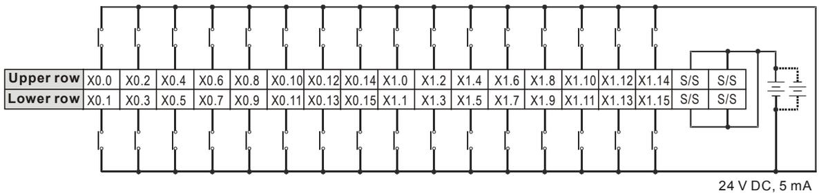
Note: UB-10-ID32A can be used with AS Series and DVP Series. The indications on the UB-10-ID32A board is for DVP Series. For the definitions of terminal connections for AS Series, you can see the reference table below. Or refer to the enclosed sticker for AS Series.
