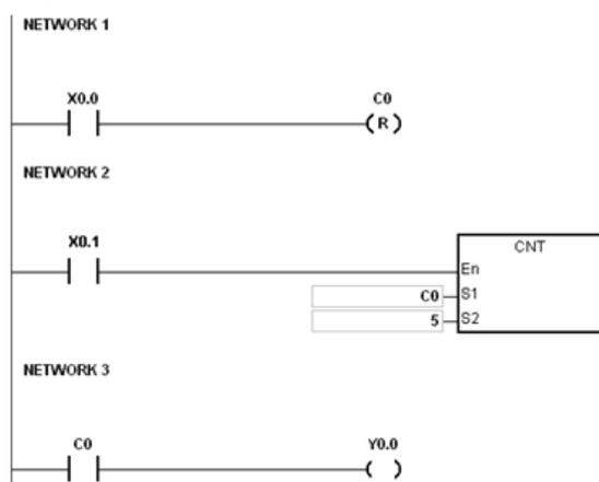
1. When X0.0=ON, the instruction RST will be executed and the current value of C0 will be reset to zero and the output contact of the counter C0 will be FF.
