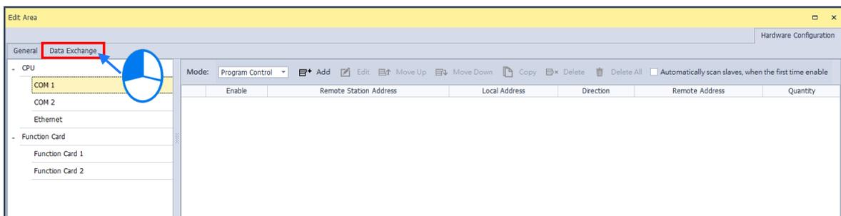
AS Series PLC CPU is built with two ports, two COM ports or one COM port and one Ethernet port varied by different models. When acted as a Master and performs data exchange with a remote Slave, the data exchange through COM1 and COM2 is via the Modbus protocol; if the data exchange through Ethernet is via the Modbus TCP protocol. The setting items for COM1, COM2 and Ethernet are the same.
