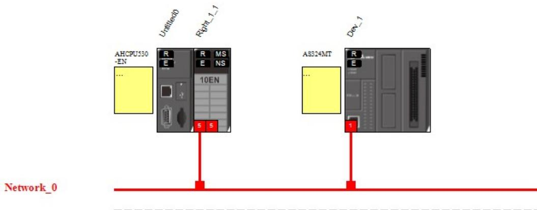
(c) Once the connection is established, click the network line "Network\_0" to see all the connected devices in this network in the Information window.
