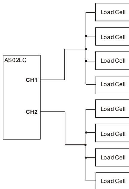
\*1. Connect the  $\oplus$  of the power module and the  $\oplus$  of the load cell module to the system ground terminal. Use the system ground as the third grounding or connect it to the control box.
