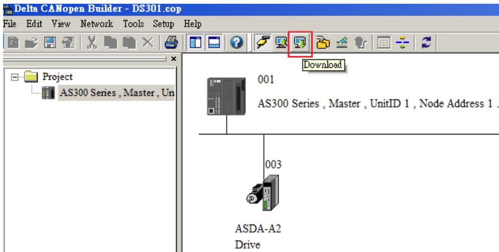
Note: you must reboot the AS300 Series PLC to enable the downloaded parameters.
