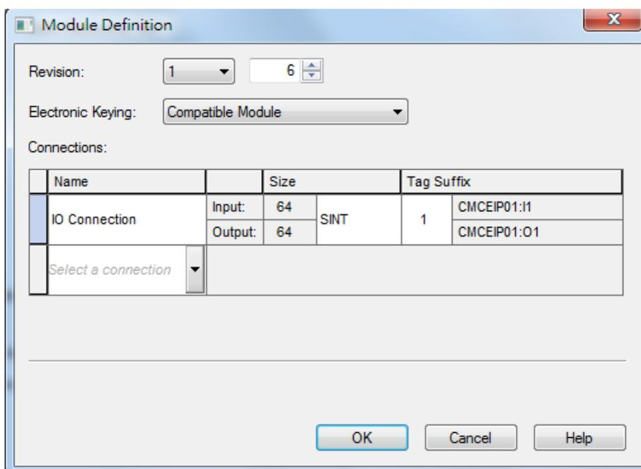
※ In general, there is no need to change the parameters from the imported EDS files which can usually be used without modification.
