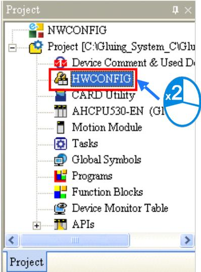
In the **HWCONFIG** window, the default setting is for a CPU module. Refer to Chapter 8 for more information on settings for other types of modules.
