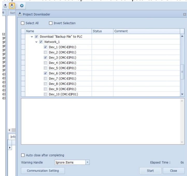
Step 3: Make sure you have the backup file ready and the IP addresses and Slave IDs in the backup file of the SD card are identical to the ones that need to be restored.
