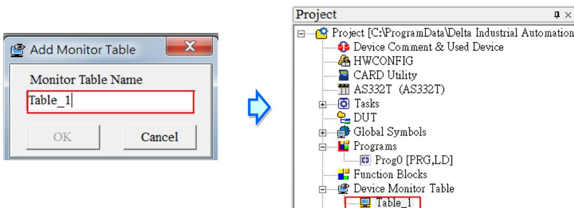
After you double-click the item, a item monitoring window appears. You can add items to be monitored to the window. To add an item to the window, double-click the blank space in the monitoring table, type a device name, type a start address, and the number of devices to be monitored in the **Device Monitor Input** dialog box. You can add up to 100 items to a monitoring table.
