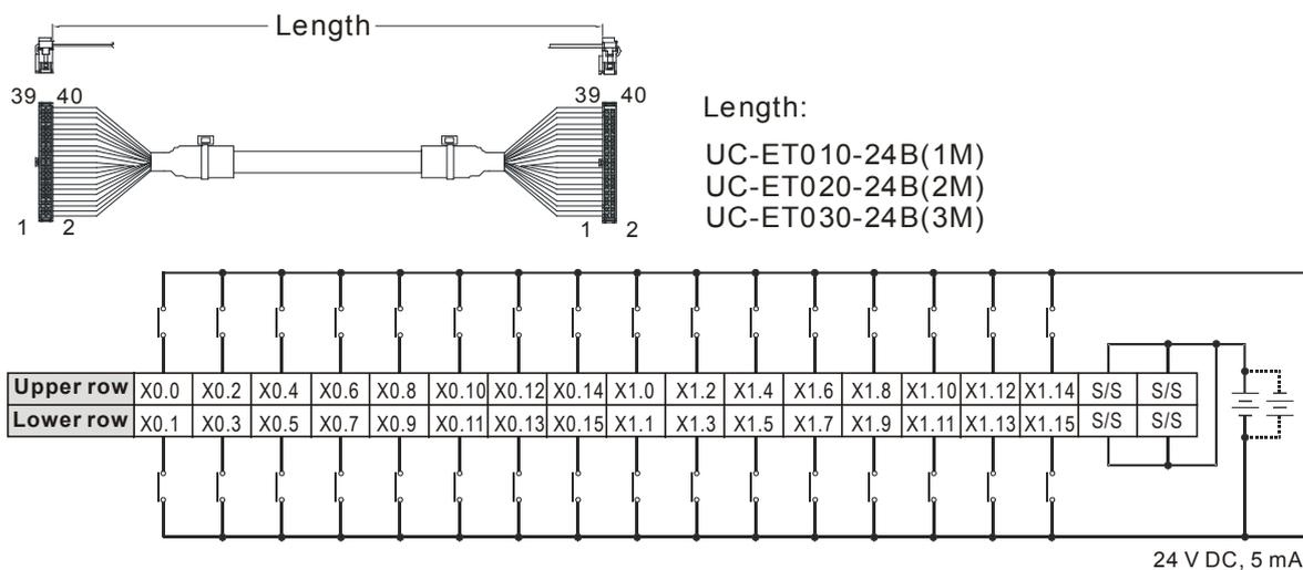
Note: UB-10-ID32A can be used with AS Series and DVP Series. The indications on the UB-10-ID32A board is for DVP Series. For the definitions of terminal connections for AS Series, you can see the reference table below.
