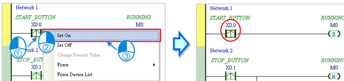
However, you can force an input contact ON or OFF during a test. Click an input or output contact to set, right-click the contact, point to **Force**, and click **On (X/Y)**, **Off (X/Y)**, **Release (X/Y)**, or **Release All**. If you force an input or output contact ON or OFF, a lock symbol appears at the left side of the contact.
