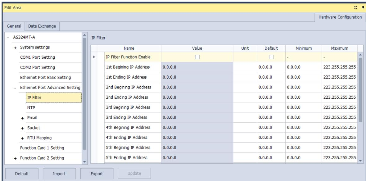
Select **IP Filter Function Enable** checkbox to enable the IP filter function and type the start address and end address of group 1~8 IP.
