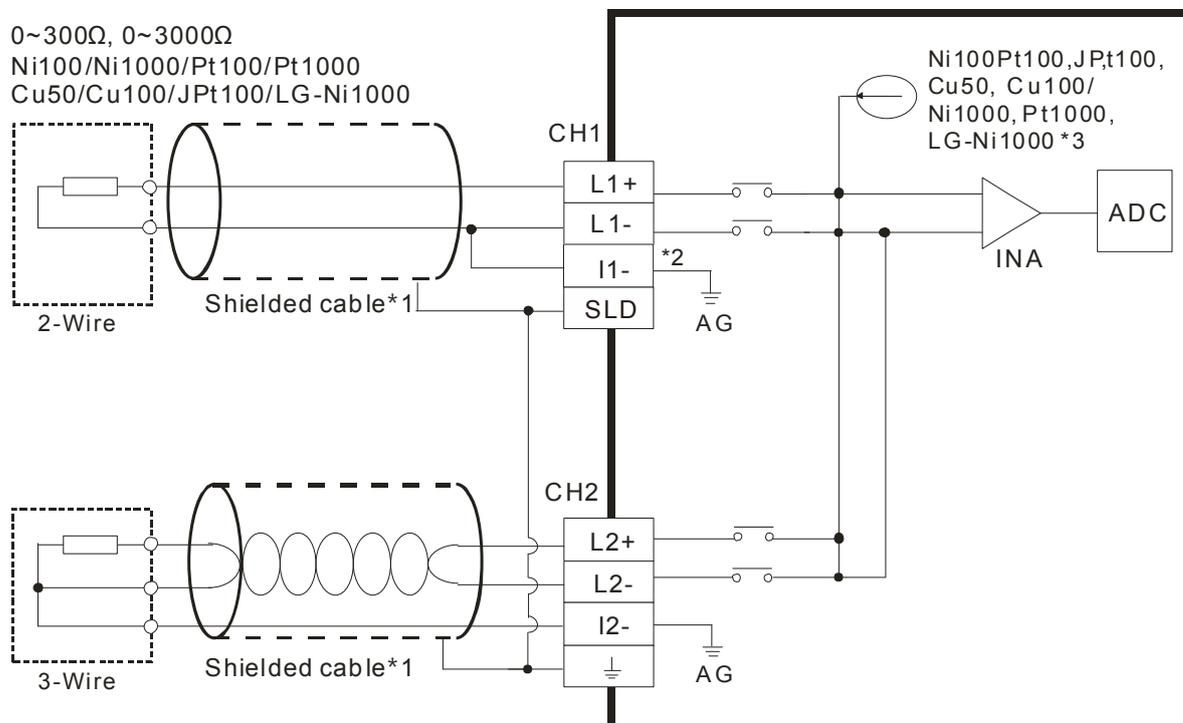
\*1. Use shielded twisted pair cables for temperature sensors, and keep them away from power cables and other cables that generate noise.
