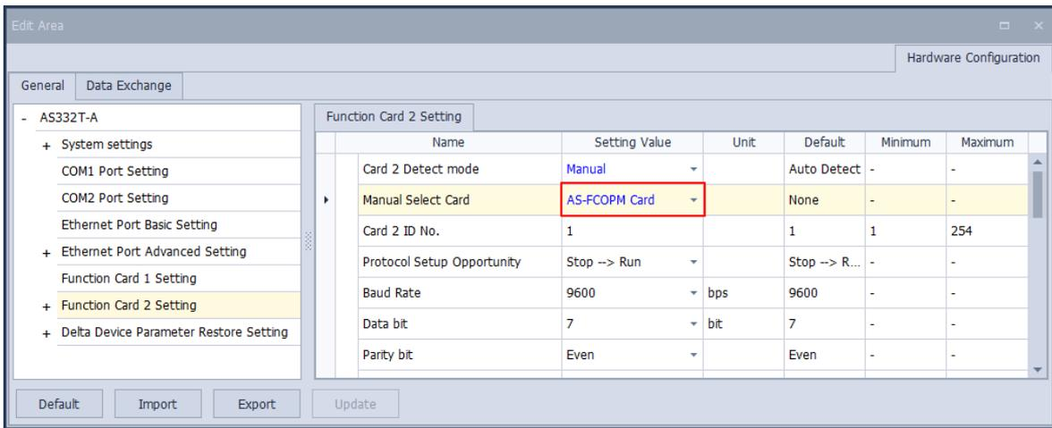
3. Select the working mode, node ID and the bit rate for AS-FCOPM.
