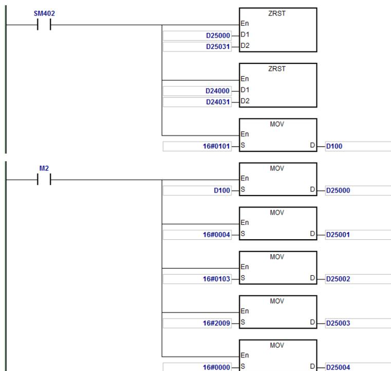
When M2=ON, after reading succeeds, the program stores the data from the target device in D24000–D24005. The value of D24005: 100 (hex) is the value read from P0-09.
