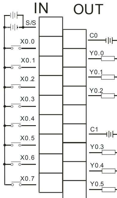
4.6.9.4 Wiring Details on AS218PX-A/AS218RX-A/AS218TX-A
