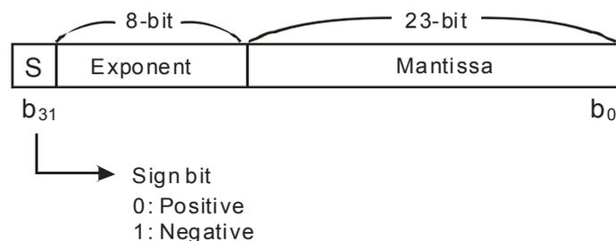
$$\text{Equation: } (-1)^S \times 2^{E-B} \times 1.M; B = 127$$
