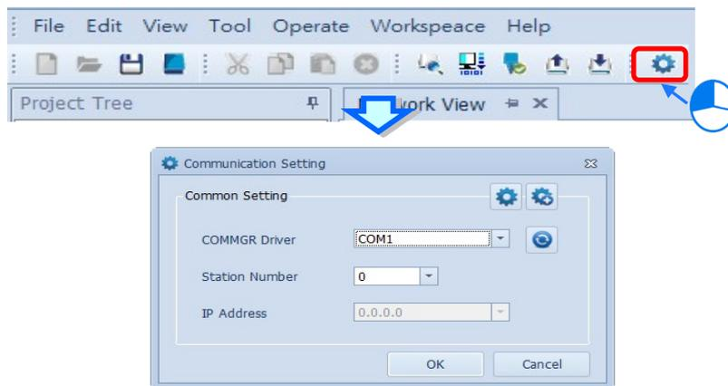
2. Once your PC is connected to the EIP Scanner, there are 3 ways to set up the network communication.
