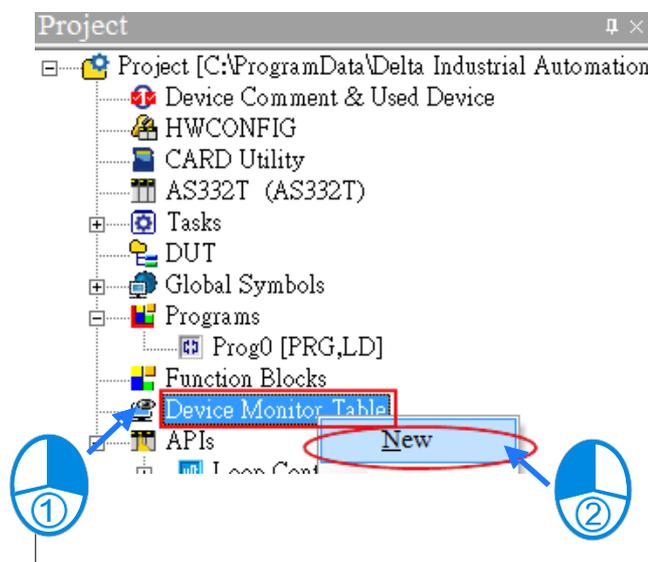
Type a table name in the **Add Monitor Table** dialog box, and then click **OK**. An item appears under **Device Monitor Table** in the project management area. Double-click the item to open the monitoring table. You can create several monitoring tables in the project, and the monitoring tables are saved with the project.
