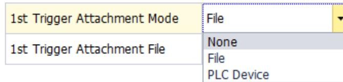
The options on the drop-down menu of **Trigger Attachment Mode** decide whether to add an attachment to the email. Please make sure the maximum size of the email file allowed before setting an attachment. For more information, refer to relevant operation manuals.
