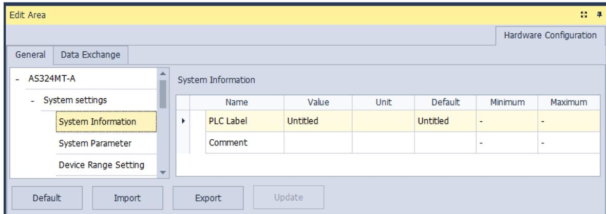
After the project is created, you can find the PLC label behind the product name in the project management area. You can change the PLC label in HWCONFIG as it is mentioned above. The PLC label is very useful when you have more than one PLC in the project. This label can be seen as the PLC identity. So that you will not change other PLC parameters by mistake. To prevent errors, when you download/upload the program, the system will remind you to check the name of the PLC CPU and the PLC label.
