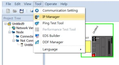
◆ The IP Manager can be the BOOTP/DHCP Server, receiving IP address requests from devices. The IP Manager window is shown below.
