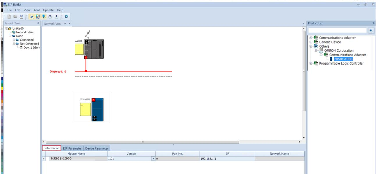
9. Drag and drop the red spare to have the Ethernet communication port connected to the network.
