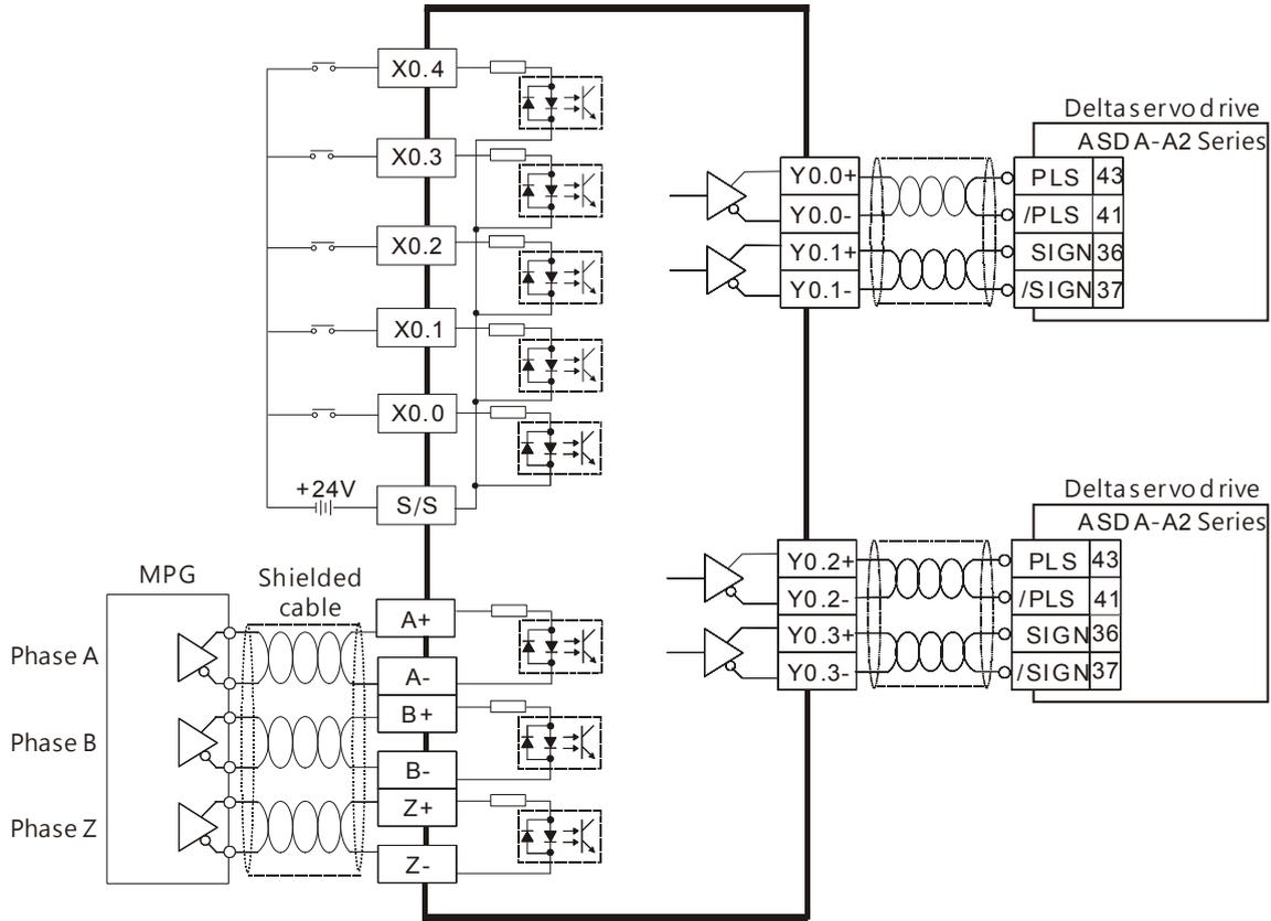
Note: Refer to API1402 from Chapter 6 in AS Series Programming Manual and Delta Servo Manual for more details on the output modes and operations.
