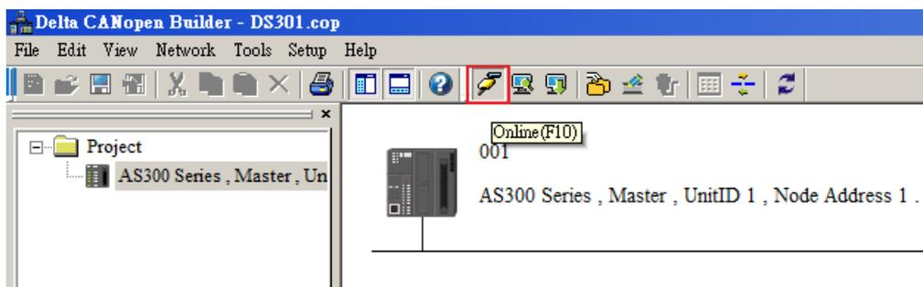
D. Click the Scan Network
