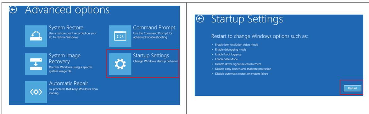
5. Press the 7 or F7 key on your keyboard to choose **Disable driver signature enforcement**. Press Enter and the system directs you back to the Windows 8 operating system. Install the Delta PLC USB driver now by connecting the AS Series CPU module to your computer's USB port. Refer to Section A2 for the steps to install the USB driver.
