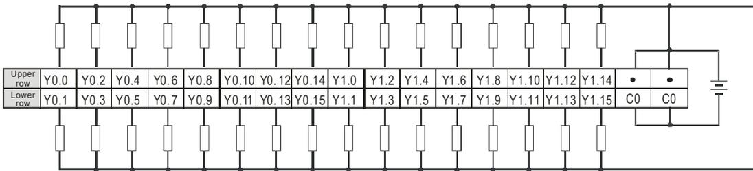
Note: UB-10-OT32A can be used with AS Series and DVP Series. The indications on the UB-10-OT32A board is for DVP Series. For the definitions of terminal connections for AS Series, you can see the reference table below. Or refer to the enclosed sticker for AS Series.
