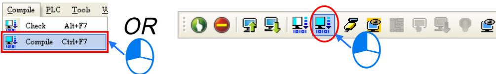
After you complete the check, the **Compile Message** page shows the check result. If there are any errors in the project, the **Compile Message** window shows the related message. After you click the message, the system automatically shows you where the error occurs. You can run the **Check** function or the **Compile** function after you correct the error.
