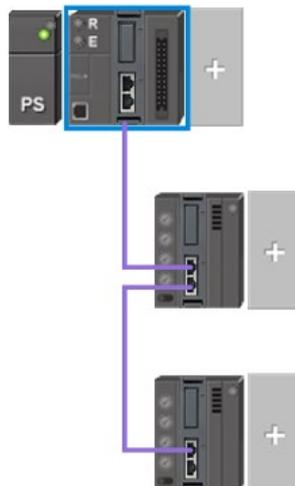
You can add more digital IO modules or analog modules to the remote module.
