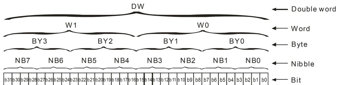
The PLC uses four types of values to execute the operation according to different control purposes. The following illustrates the values of these functions.:
