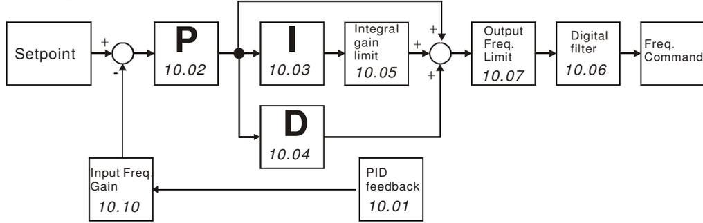
**10.07** **PID Output Frequency Limit** Unit: 1
