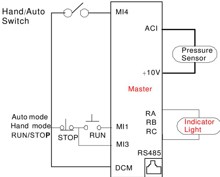
If any error occurred on the inverter of the multi-pump system, the RLY will be turned on
