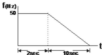
Therefore the distance travelled by the motor after the stop command is given = number of rounds x circumference =  $175 \times 2\pi r$ . That means the turtable went back to the top after 175 rounds.
