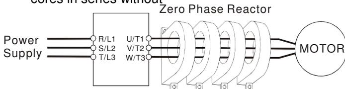
**Note 1:** The table above gives approximate wire size for the zero phase reactors but the selection is ultimately governed by the type and diameter of cable fitted i.e. the cable must fit through the center hole of zero phase reactors.
