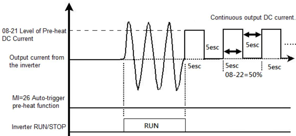
The figure below shows the Sequential Relation between Pre-heat function & enabling DC brake.
