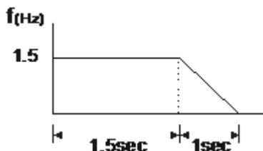
Therefore the distance travelled by the motor after the stop command is given = number of rounds x circumference =  $1.5 \times 2\pi r$ . That means the turtable stopped after 1.5 rounds.
