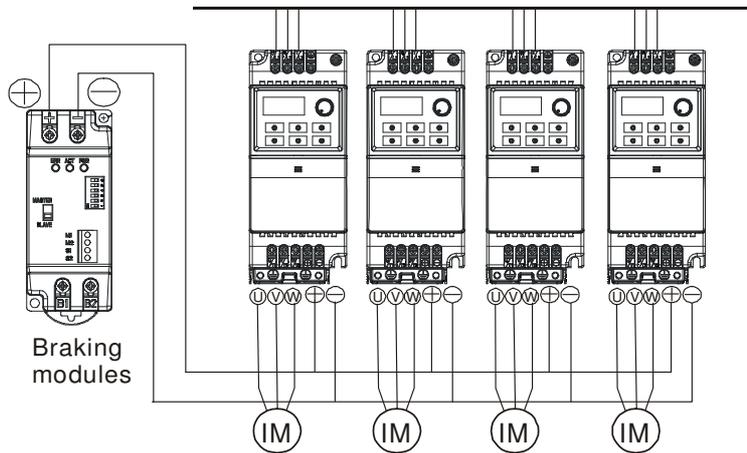
For frame A and B, terminal + (-) is connected to the terminal + (-) of the braking module.
