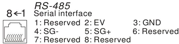
Each VFD-EL AC motor drive has a pre-assigned communication address specified by Pr.09.00. The RS485 master then controls each AC motor drive according to its communication address.
