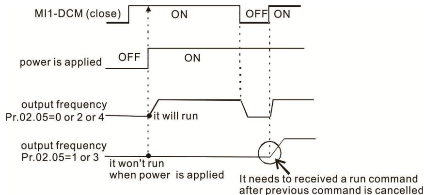
📖 When the operation command source isn't from the external terminals, independently from whether the AC motor drive runs or stops, the AC motor drive will operate according to Pr.02.05 if the two conditions below are both met.
