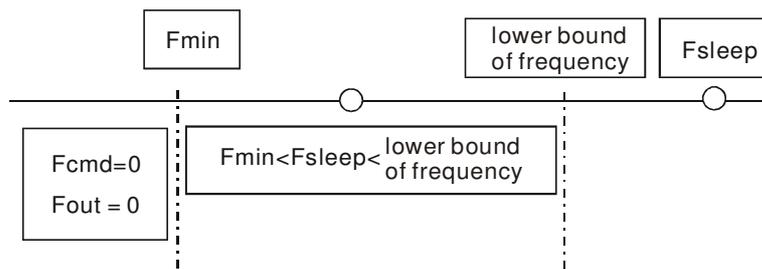
When output frequency  $\leq$  sleep frequency and time  $>$  detection time, it will go in sleep mode.
