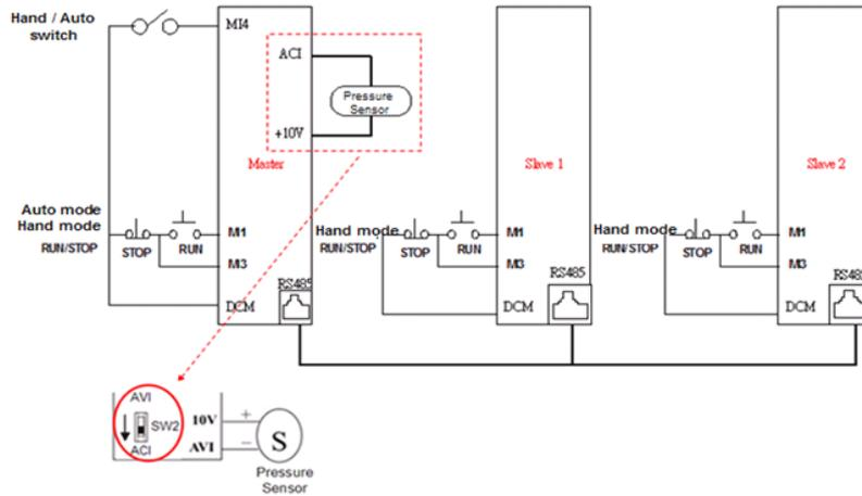
Wiring of the pressure sensor:
