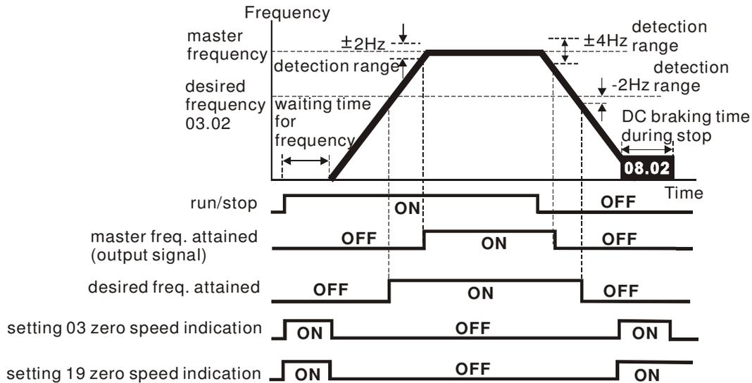
**output timing chart of multiple function terminals
