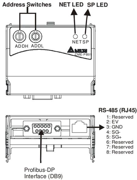
1. SP LED: Indicating the connection status between VFD-EL and CME-PD01.
