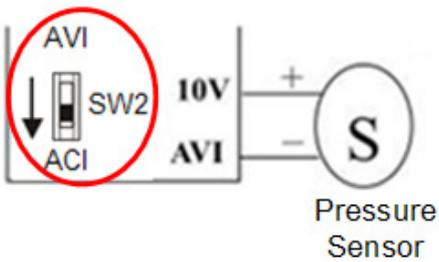
Wiring of the pressure sensor:
