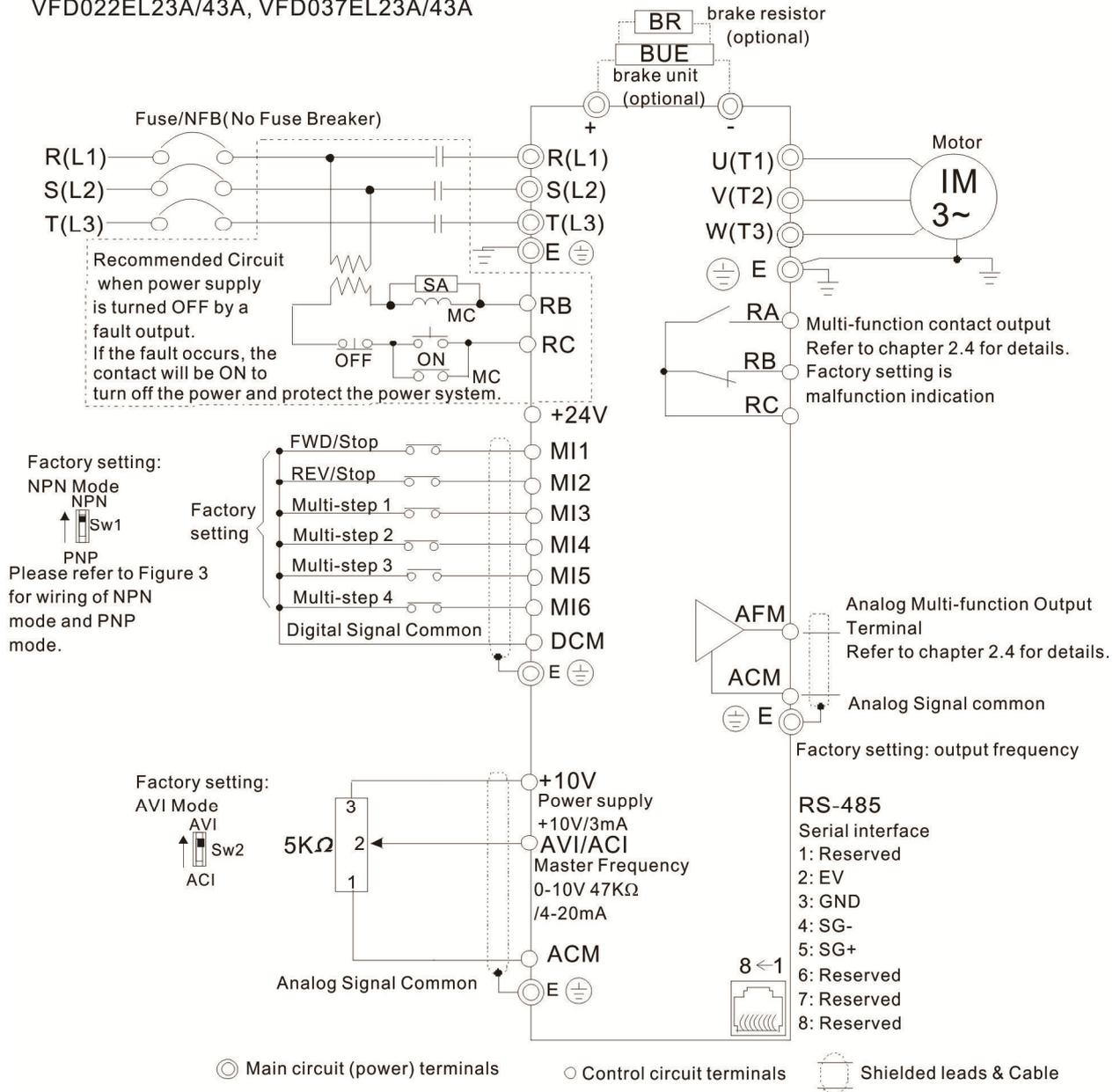
Figure 3 Wiring for NPN mode and PNP mode
