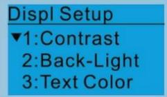
After you set the value, press ENTER to see the screen display after contrast is adjusted to +10.
