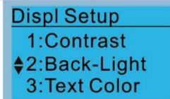
When the setting value is 10 Min, the backlight turns off in 10 minutes.
