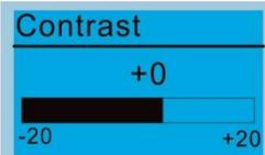
Press the Up / Down keys to adjust the setting value.
