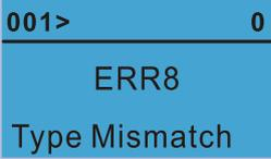
If you select “Option 1: Keypad→VFD”, check if the PLC program is built-in to the KPC-CC01 keypad. If the PLC program is not available in the keypad when you select “Option 1: Keypad→VFD”, an “ERR8 Warning: Type Mismatch” displays on the screen.
