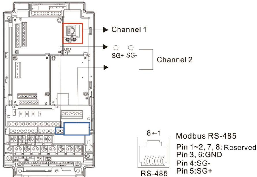
3. The client can simultaneously access data from the converter and internal PLC, which is performed through identification of the node. For instance, if the converter node is 1 and the internal PLC node is 2, then the client command will be
