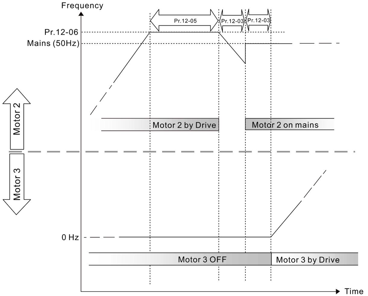
Diagram 12-4: Sequence of switching motors at Fixed Quantity Circulation with PID
