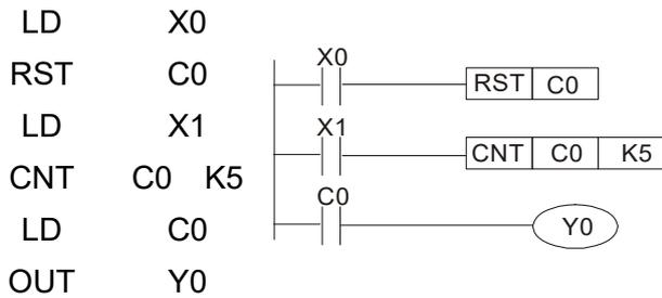
1. When X0 = ON and the RST command is executed, the current value of C0 will revert to 0, and the output contact will revert to OFF.
