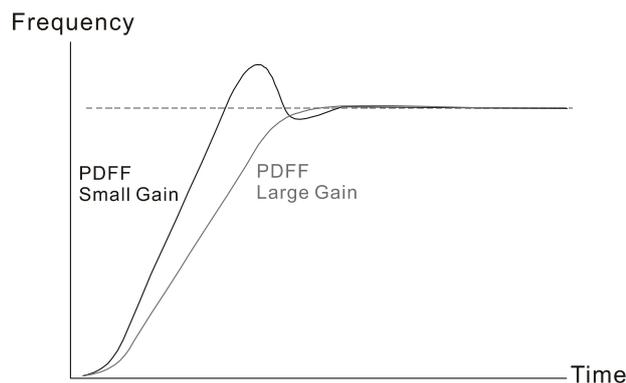
↗ **11-14** ASR Output Low Pass Filter Time
