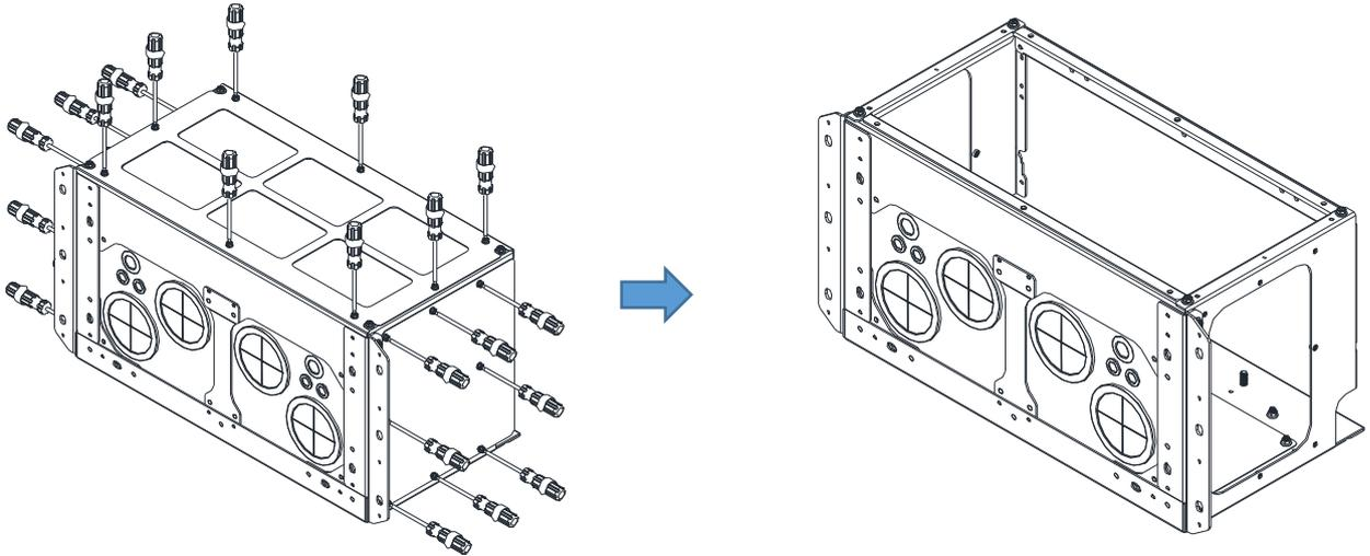
2. Remove the 4 covers of conduit box, and fasten the loosen screws back to the original location. Screw torque: 100–110 kg-cm / [86.7–95.4 lb-in] / [9.8–10.8 Nm]
