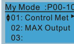
3. To delete a parameter, go to My Mode and select the parameter to delete. Press ENTER to enter the parameter setting screen. DEL appears in the bottom left corner of the screen. Press F4 to delete this parameter from My Mode.
