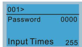
If the WPLSoft editor is installed uses password, enter the password to save the file to the keypad.
