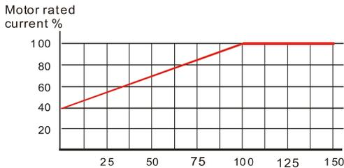
Motor cooling curve with shaft-fixed fan
