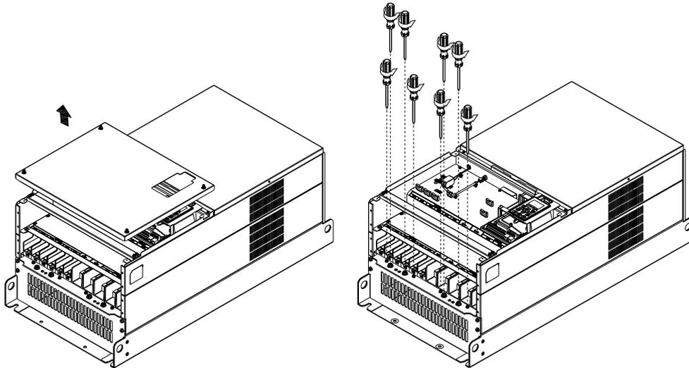
4. Install the conduit box by fastening all the screws shown in the following figure.
