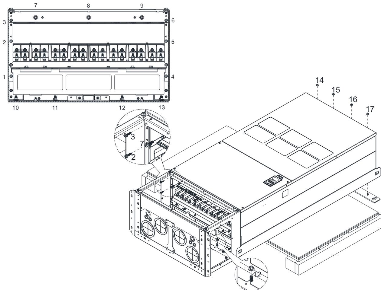
5. Fasten the 3 covers and screws, which are loosen from step1, to the original location.
