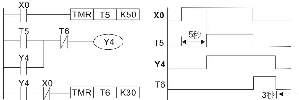
Example 12: Extended timing circuit
