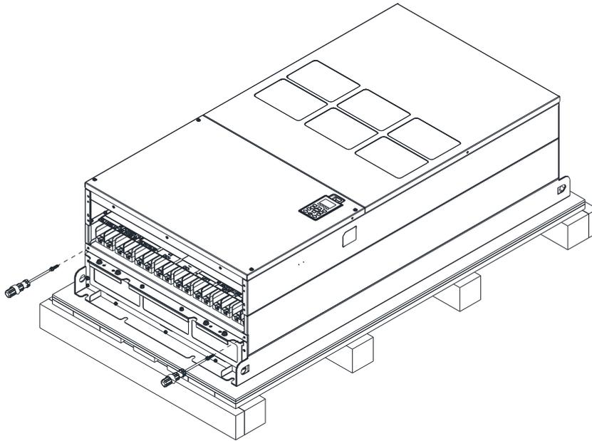
5. Install conduit box and accessories by fasten all the screws shown in the following figure.
