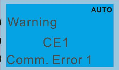
The LCD keypad display shows the word "Warning" at the top, "CE1" in the middle, and "Comm. Error 1" at the bottom. The word "AUTO" is visible in the top right corner of the display area.
