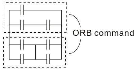
In the case of ANB and ORB operations, if a number of blocks are connected, they should be combined to form a block or network from the top down or from left to right.
