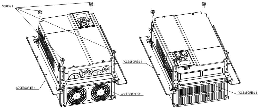
2. Plate installation, place 8 of the screw 2 (M6) through Accessory 1&2 and the plate, then fasten the screws. Screw torque: 25–30 kg-cm / [21.7–26 lb-in.] / [2.5–2.9 Nm] (As shown in the following figure)
