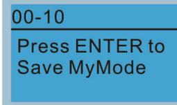
2. The parameter (Pr) displays in My mode if it is properly saved. To correct or to delete this parameter, press F4 for DEL.
