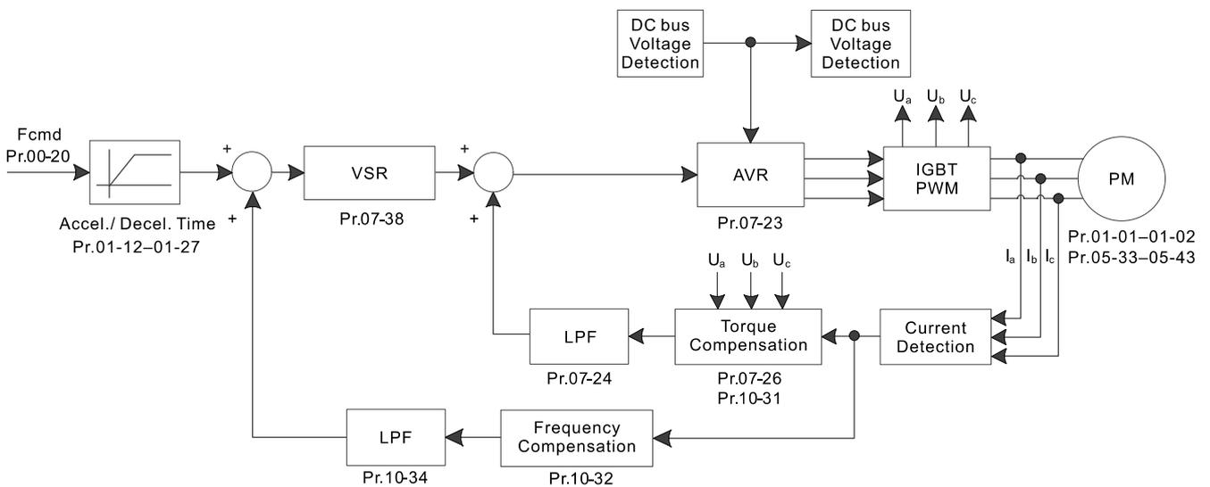
When you set Pr.00-11 to 6, PM FOC Sensorless control diagram is as follows:
