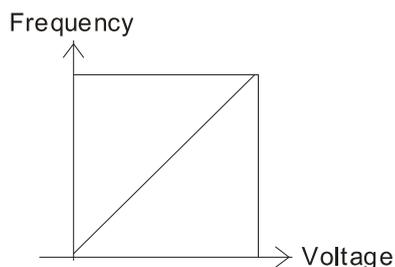
$$F_{cmd} = [(ay \pm bias) * gain] * \frac{F_{max}(01-00)}{10V \text{ or } 16mA \text{ or } 20mA}$$
