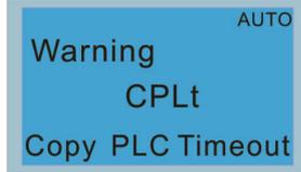
If you unplug the keypad and plug it back while copying the PLC program, the screen displays a CPlt warning.
