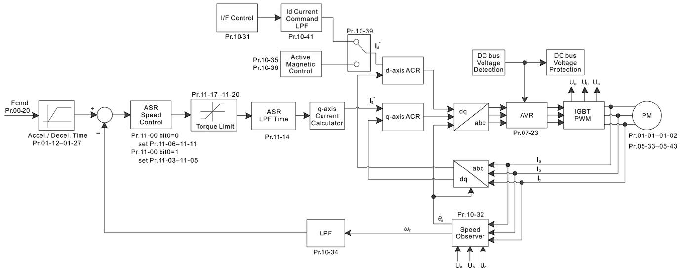
When you set Pr.00-11 to 8, SynRM Sensorless control diagram is as follows:
