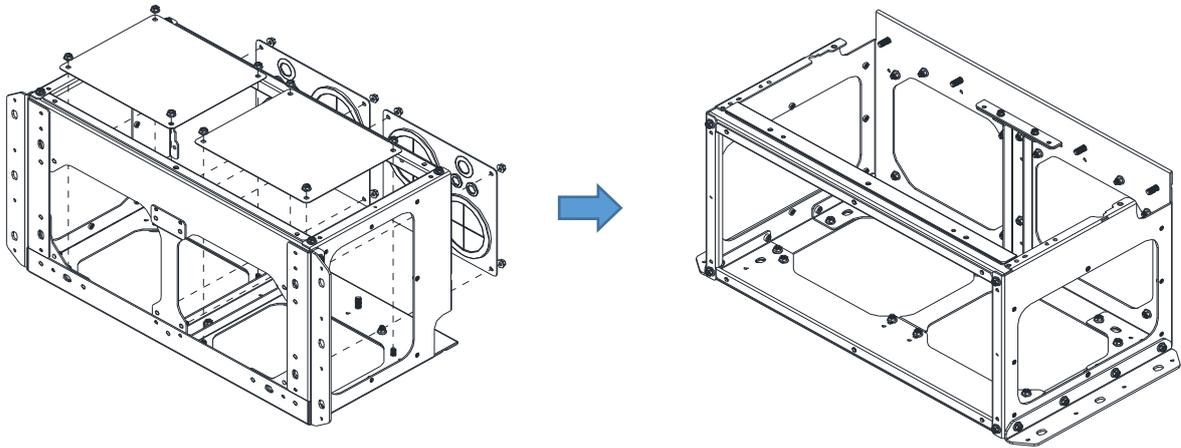
3. Remove the parts and screws as below figure shown.
