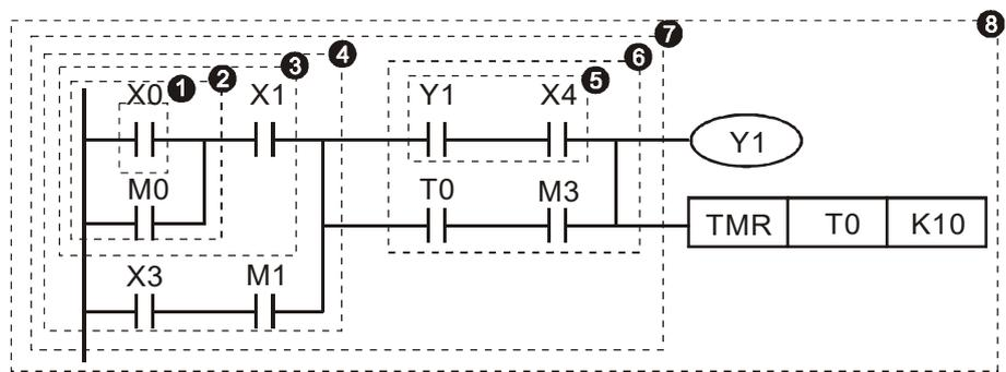
Explanation of basic structure of ladder diagrams
