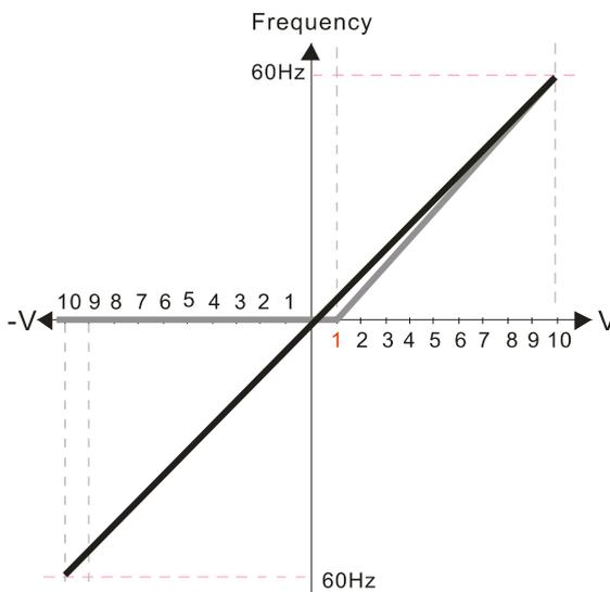
Pr.00-21=0 (Digital keypad control and run in FWD direction)
