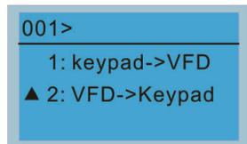
Press ENTER to go to the “VFD→Keypad” screen.
