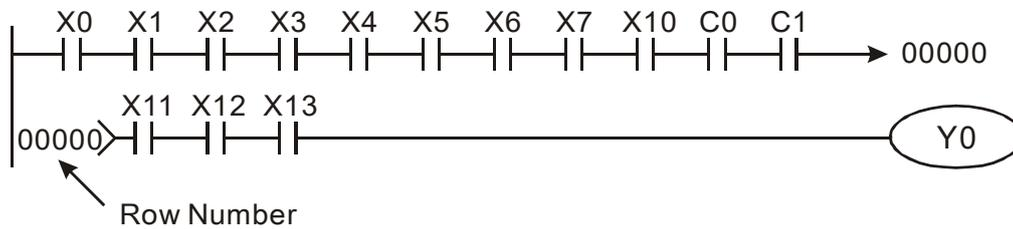
The ladder diagram programming method involves scanning from the upper left corner to the lower right corner. The coils and applications command computing box are handled in the output, and the ladder diagram is placed on the farthest right. Taking the figure below as an example, we can gradually analyze the procedural sequence of the ladder diagram. The number in the upper right corner gives the sequential order.
