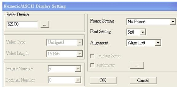
Click [...]. In the **Refer Device** dialog box, choose the VFD communication port that you need. If you want to read the output frequency (H), set the **Absolute Addr.** to 2202. For other values, refer to the ACMD Modbus Comm Address List (see Pr.09-04 in Chapter 12 Group 09 Communication Parameters).
