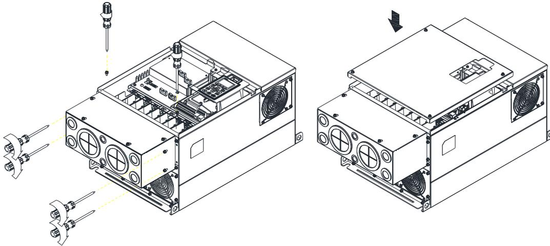
3. Fasten the 4 screws shown in the following figure. Screw torque: 12–15 kg-cm / [10.4–13 lb-in.] / [1.2–1.5 Nm]
