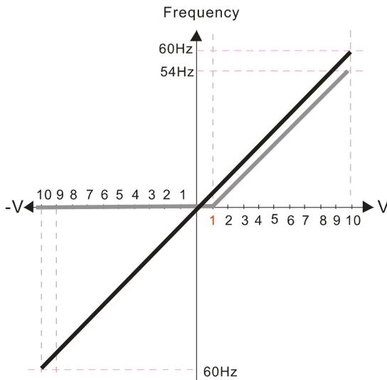
Pr.00-21=0 (Digital keypad control and run in FWD direction)
