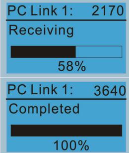
Start to upload parameters to VFDSOft
