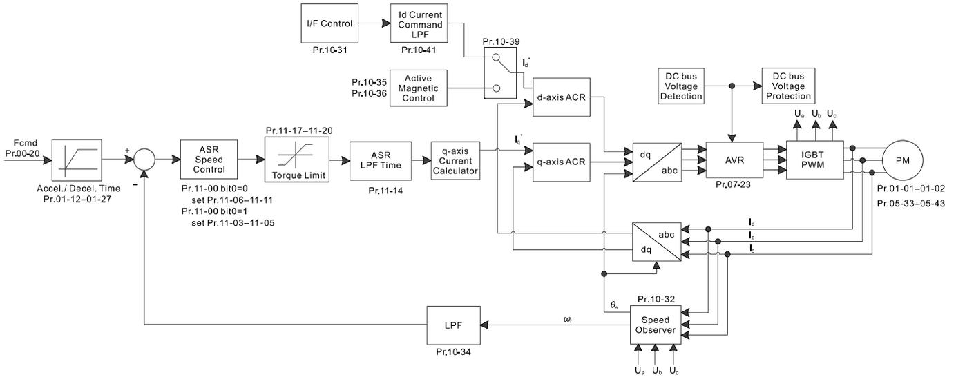
※ PM Sensorless FOC control is the control method dedicated for PM; it uses the high salient pole characteristic of PM to detect positions of NS magnetic poles. By doing this, it calculates the motor's rotor position at low-speed frequency.
