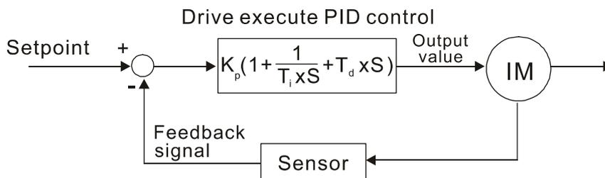
$K_p$  Proportional Gain (P),  $T_i$  Integral Time (I),  $T_d$  Differential Time (D), S Calculation
