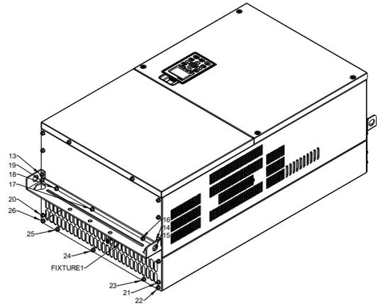
5. Place 4 of the M12 screws through Fixture 1&2 and plate then fasten the screws.
