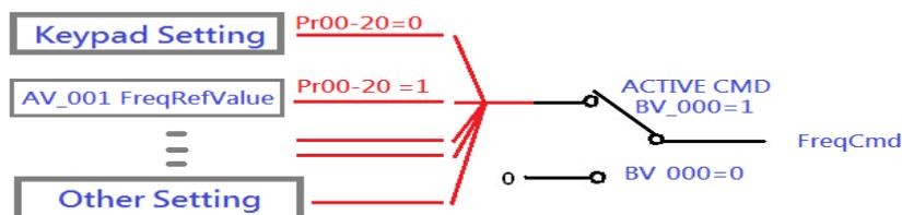
PS. In CP2000, base on different Pr setting or IO setting, we can make FreqCmd with different source of Reference Value.
