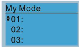
Press F4 in parameter setting screen to save the parameter to My Mode. To delete or correct the parameter, select this parameter and press F4 for DEL in the bottom right corner.
