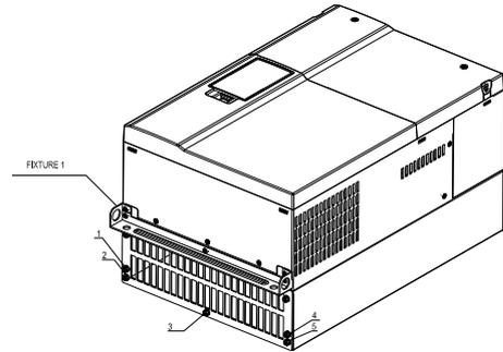
7. Place 4 screws (M10) through Fixture 1&2 and the plate then fasten the screws. (as shown in the following figure)
