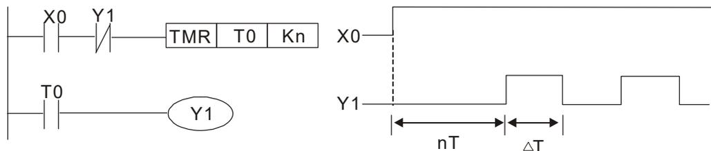
Example 8: Flashing circuit
