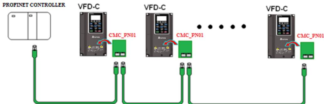
When the hardware is installed and power on, the current set value of Pr.09-60 will be 12, and shows "PROFINET" on the display. If the above information does not show on the display, check the version of CP2000 and the connection of the card.
