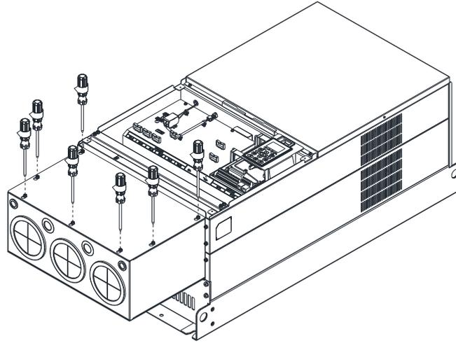
6. Place the cover back to the top and fasten the screws (as shown in the figure).
