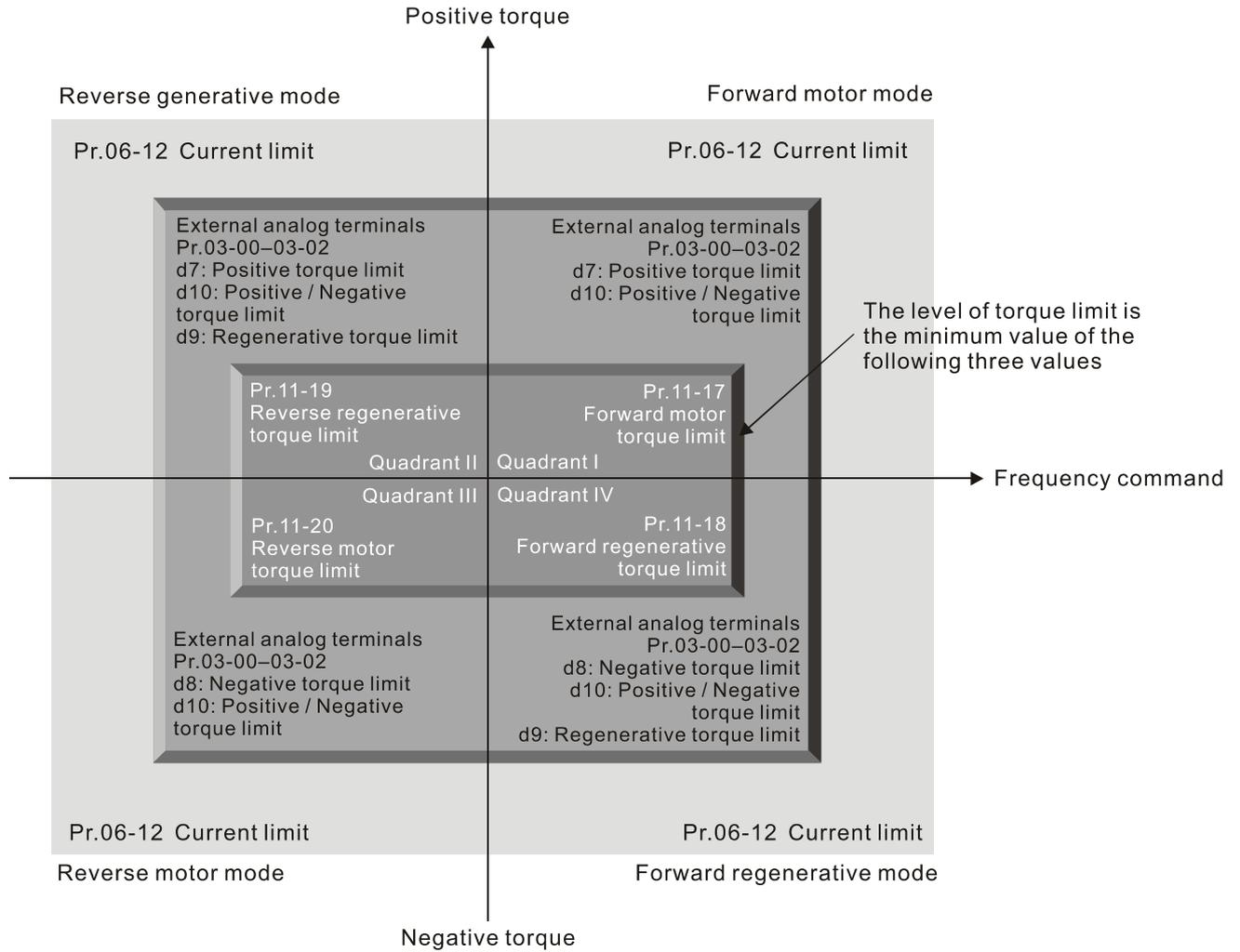
📖 All control mode is based on 100% of the motor rated current except for these four modes: IM: VF, SVC and PM: PMSVC modes.
