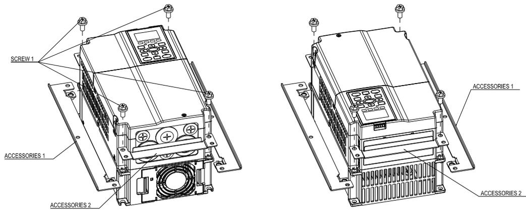
2. Plate installation, place 6 of the screw 2 (M6) through accessory 1&2 and the plate, then fasten the screws. Screw torque: 25–30 kg-cm / [21.7–26 lb-in.] / [2.5–2.9 Nm] (As shown in the following figure)
