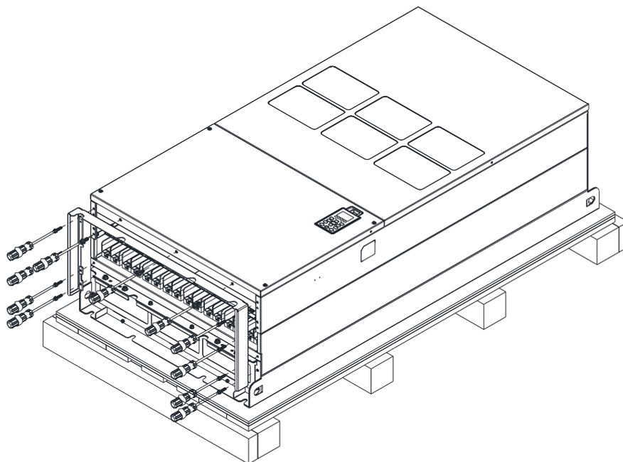
3. Fasten the M6 screws to locations shown in below figure.
