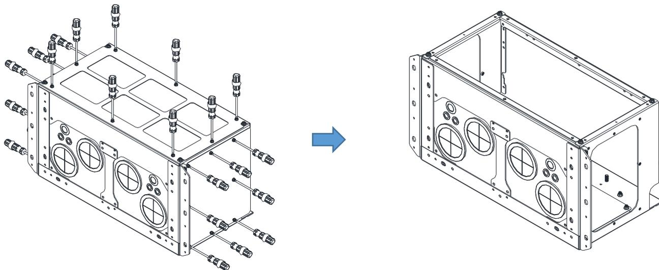
2. Loosen the screws as below figure shown.
