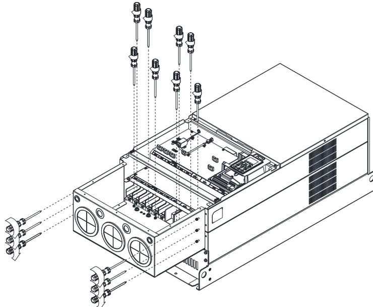
5. Fasten all the screws. Screw torque: 24–26 kg-cm / [20.8–22.6 lb-in.] / [2.4–2.5 Nm]
