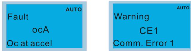
1. Press the STOP / RESET key to reset the fault code. If there is no response, contact your local distributor or return the unit to the factory. To view the fault DC bus voltage, output current and output voltage, press MENU and then choose 6: Fault Record.
