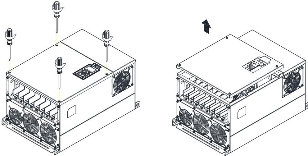
2. Fasten the 6 screws shown in the following figure and place the cover back to the original position. Screw torque: 24–26 kg-cm / [20.8–22.6 lb-in.] / [2.4–2.5 Nm]
