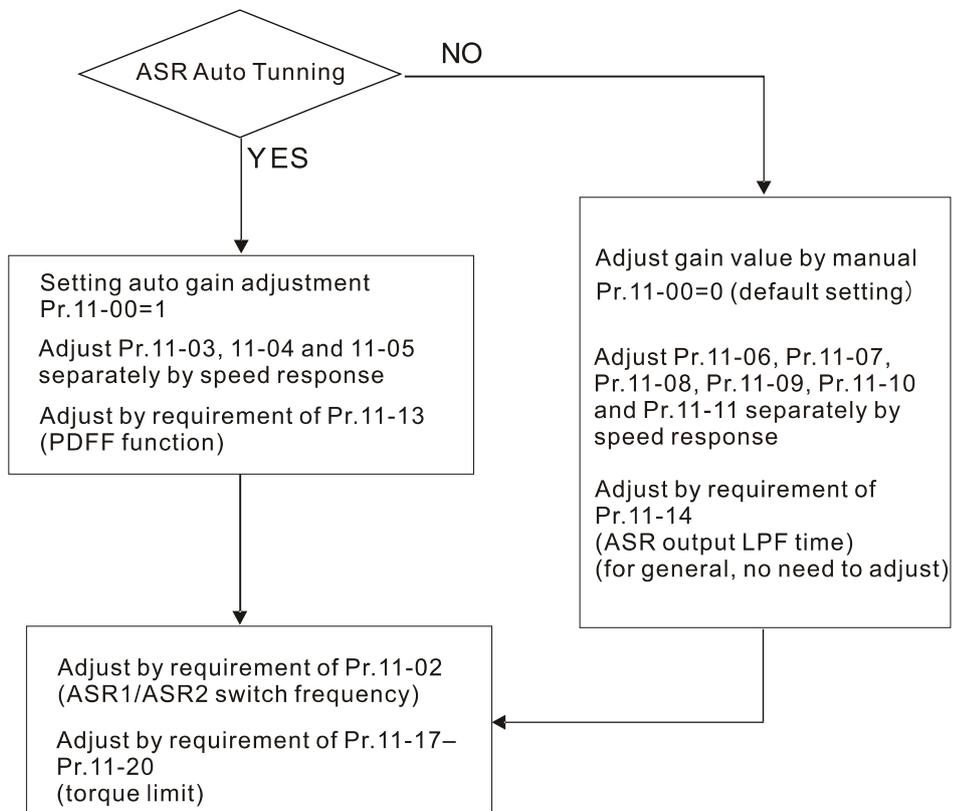
📖 When the drive needs to keep a certain torque at zero-speed, or it needs a steady frequency output at extreme low speed, increase Pr.11-05 zero-speed bandwidth appropriately. If there is serious output current vibration that cause the drive vibrates in high-speed area, then decrease the high-speed bandwidth.
