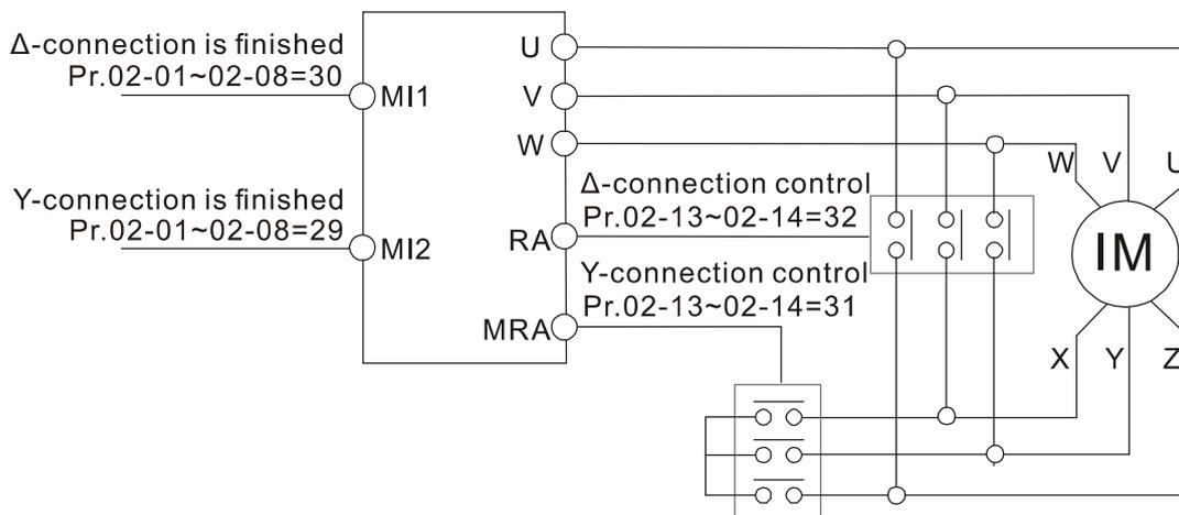
Y-Δ connection switch: can be used for wide range motor
