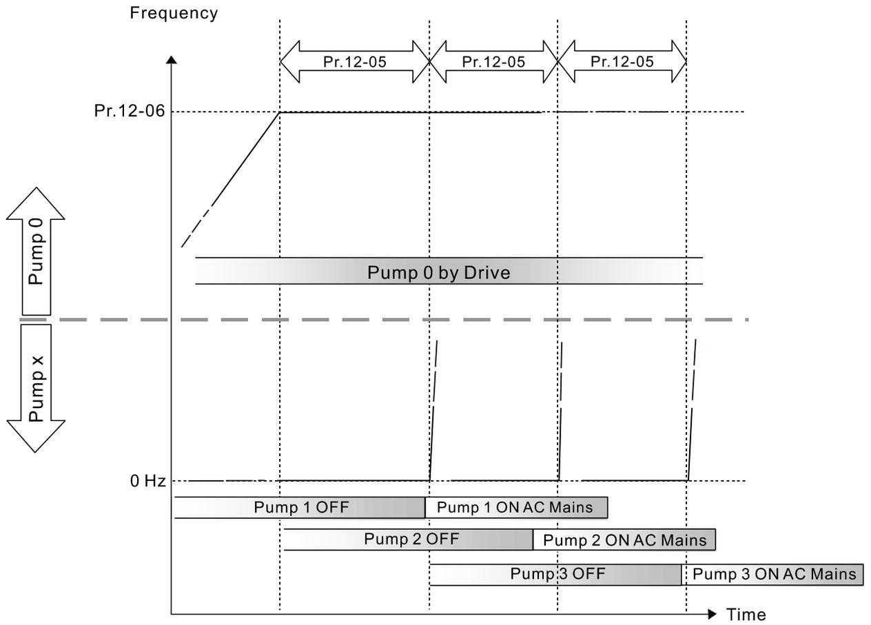
Diagram 12-9: Sequence of switching motors at Fixed Quantity Control with PID
