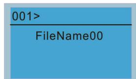
Press the Up / Down keys to select a symbol. Press the Left / Right keys to move the cursor to select a file name.
