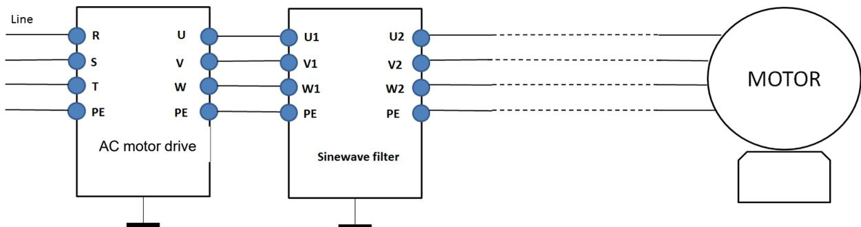
Wiring of non-shielded cable Figure 7-39
