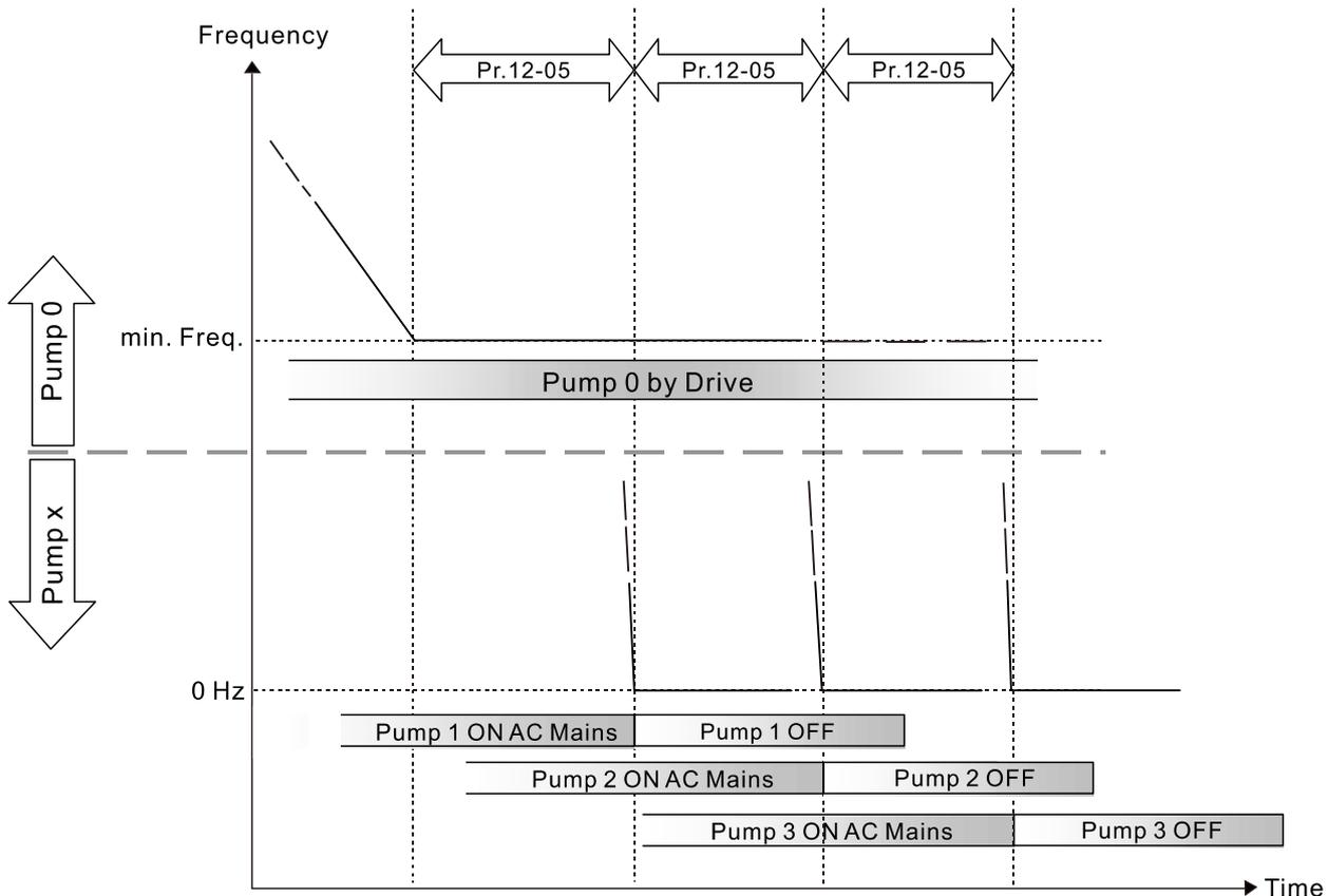
Diagram 12-11: Sequence of switching motors at Fixed Quantity Control with PID
