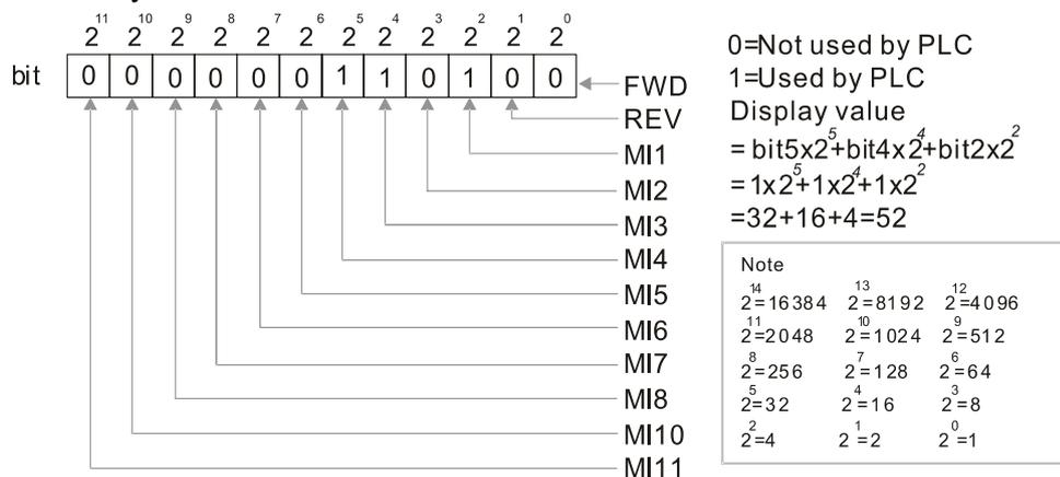
**02-53** Display the External Multi-function Output Terminals Used by PLC
