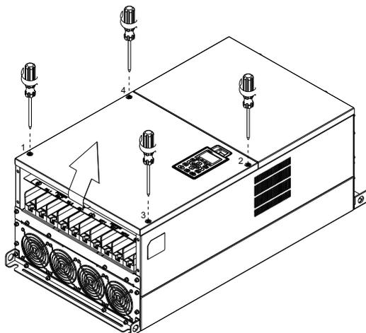
2. Install the conduit box by fastens the 4 screws, as shown in the following figure. Screw torque: 24–26 kg-cm / [20.8–22.6 lb-in.] / [2.4–2.5 Nm]
