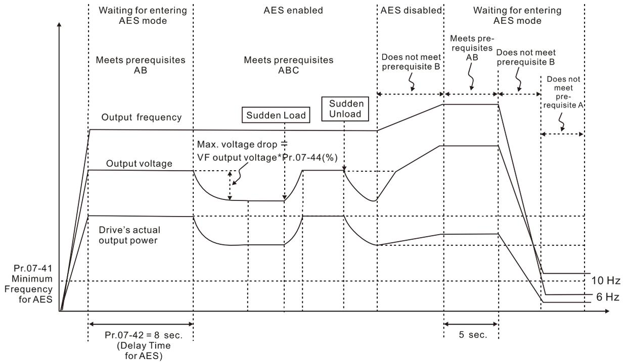
📖 The energy-saving function is invalid during the drive's acceleration and deceleration. To make it valid, the prerequisites need to be verified again.
