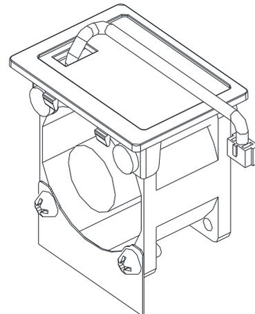
**Frame C****Heat sink Fan 『MKC-CFKM』****Following Models use one set of MKC-CFKM:**
