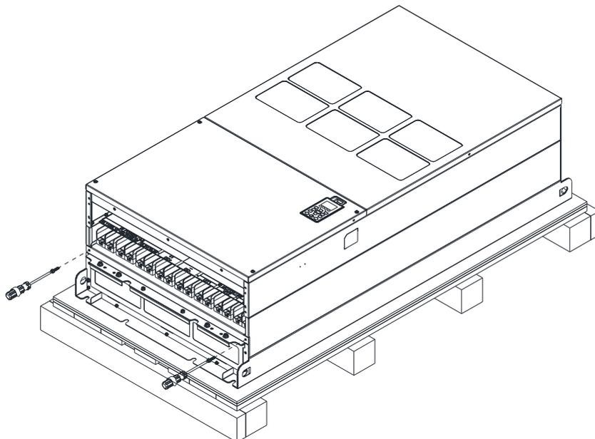
4. Install the conduit box by fasten all the screws shown in the following figure
