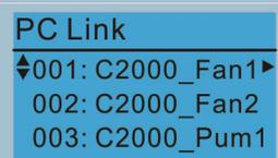
Press the Up / Down keys to select a parameter group to upload to VFDSOft.
