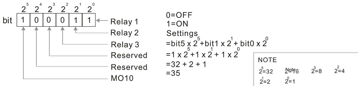
**02-52** Display the External Multi-function Input Terminals Used by PLC
