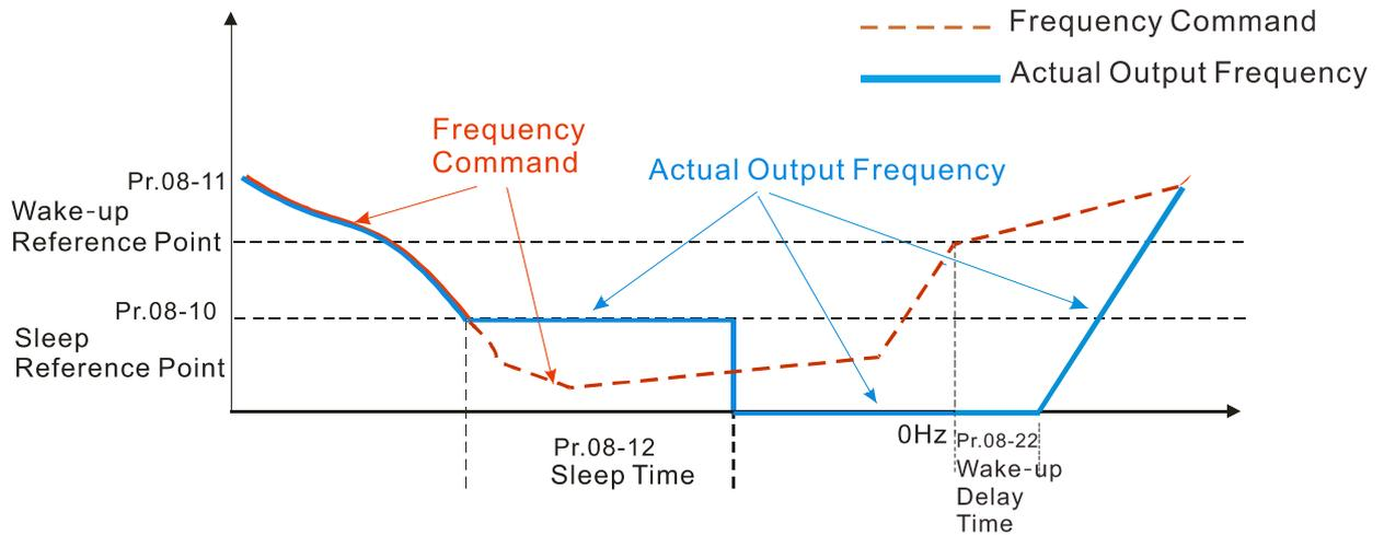
2. Internal PID Calculation Frequency Command (PID is in use, Pr.08-00  $\neq$  0 and Pr.08-18 = 0)
