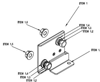
Diagram of power terminal connection
