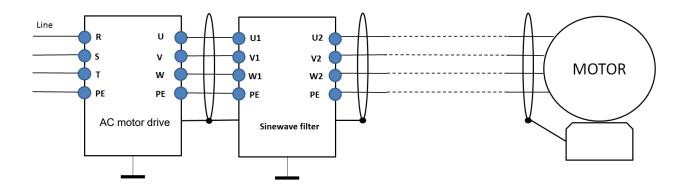
Wiring of shielded cable Figure 7-40
