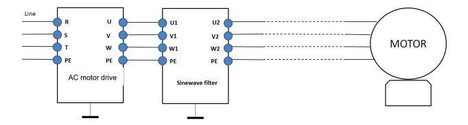
Wiring of non-shielded cable Figure 7-39
