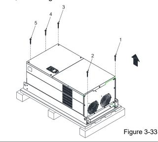
Loosen the 12 screws fasten the drive on the pallet, and then remove the wood plates and the conduit box.
