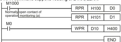
Recommendation Take care when using the WPR command. When writing parameters, because most parameters are recorded as they are written, these parameters may only be revised 109 times; a memory write error may occur if parameters are written more than 109 times.
