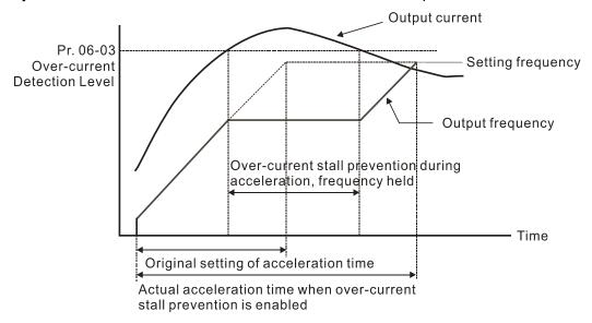
Refer to Pr.06-16 for more details of stall level in flux weakening region. The protection curve is as following:
