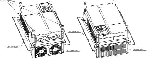
Plate installation, place 8 of the screw 2 (M6) through Accessory 1&2 and the plate, then fasten the screws. Screw torque: 25–30 kg-cm / [21.7–26 lb-in.] / [2.5–2.9 Nm] (As shown in the following figure)
