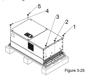
Loosen the five screws fasten the drive on the pallet, and then remove the wood plates and the conduit box.
