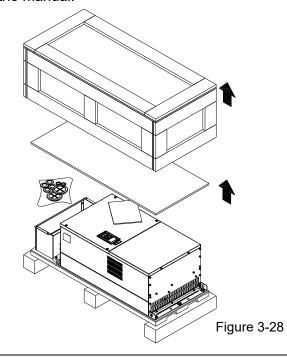
Loosen the five screws fasten the drive on the pallet, see the figure below.
