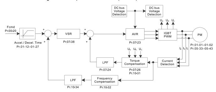
When you set Pr.00-11 to 6, PM FOC Sensorless control diagram is as follows:
