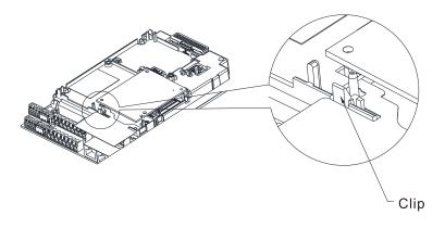
Twist to open the other clip to remove the PCB.
