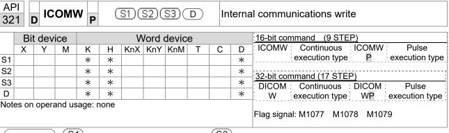
S1: Selection of slave device. S2: Device selection (0: converter, 1: internal PLC). S3: Read address. D: Saving target.
