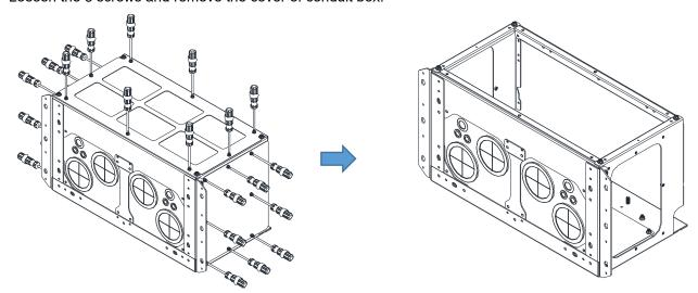
2. Remove the 4 covers of conduit box, and fasten the loosen screws back to the original location. Screw torque: 100–110 kg-cm / [86.7–95.4 lb-in] / [9.8–10.8 Nm]
