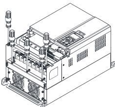
3. Install the conduit box by fasten the 5 screws shown in the following figure. Screw torque: 24–26 kg-cm / [20.8–22.6 lb-in.] / [2.4–2.5 Nm]
