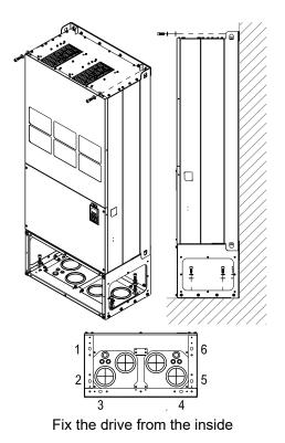
Fix the drive from the inside Screw M12\*8 Torque: 340–420 kg-cm / [295.1–364.6 lb-in.] / [33.3–41.2 Nm]
