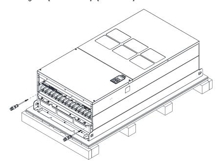
4. Install the conduit box by fasten all the screws shown in the following figure Screw 1–6: M6 screw torque: 55–65 kg-cm / [47.7–56.4 lb-in] / [5.4–6.4 Nm] Screw 7–9: M8 screw torque: 100–110 kg-cm / [86.7–95.4 lb-in] / [9.8–10.8 Nm] Screw 10–13: M10 screw torque: 250–300 kg-cm / [216.9–260.3 lb-in] / [24.5–29.4 Nm] Screw 14–17: M8 screw torque: 100–110 kg-cm / [86.7–95.4 lb-in] / [9.8–10.8 Nm]
