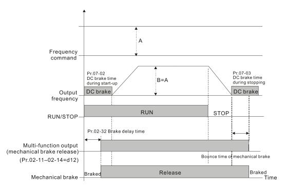
This parameter is invalid if it is used without DC brake. Refer to the following operation timing.
