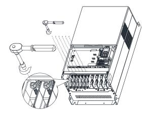
4. Install the 3pcs copper assy., as shown in the following figure 1. Fasten the upper M8 nuts (1–6) with a sleeve wrench (12 mm of the sleeve), as shown in the figure 2 below.
