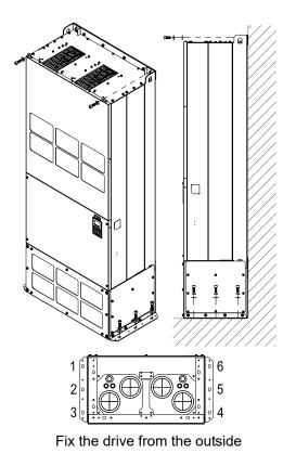
Fix the drive from the outside Screw M12\*8 Torque: 340–420 kg-cm / [295.1–364.6 lb-in.] / [33.3–41.2 Nm]
