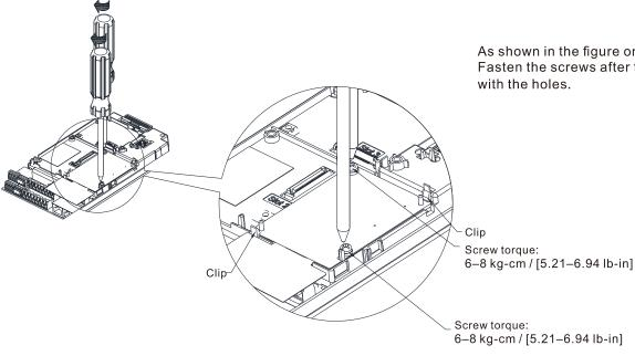
As shown in the figure on the left. Fasten the screws after the PCB is clipped with the holes.
