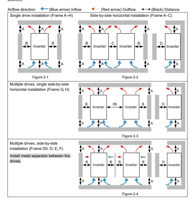
Multiple drives side-by-side vertical installation
