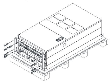
3. Fasten the M6 screws to locations shown in below figure. Screw torque: 35–45 kg-cm / [30.3–39 lb-in.] / [3.4–4.4 Nm]
