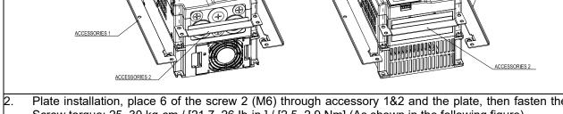
Plate installation, place 6 of the screw 2 (M6) through accessory 1&2 and the plate, then fasten the screws. Screw torque: 25–30 kg-cm / [21.7–26 lb-in.] / [2.5–2.9 Nm] (As shown in the following figure)
