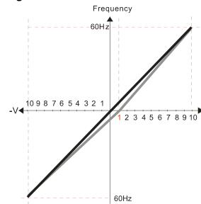
Pr.00-21=0 (Digital keypad control and run in FWD direction) Pr.03-05 Analog Positive Voltage Input Bias (AVI2) = 10%
