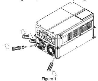
(As shown in Figure 2), remove the power connector, loosen the screw and remove the fan kit. When installing
