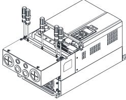
4. Fasten the 2 screws shown in the following figure. Screw torque: 12–15 kg-cm / [10.4–13 lb-in.] / [1.2–1.5 Nm]
