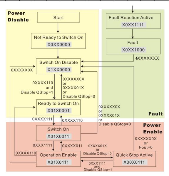
Set command 6040 = 0xE, then set another command 6040 = 0xF. Then you can switch the motor drive to Operation Enable. The Index 605A determines the direction of the lines from Operation Enable when the control mode changes from Quick Stop Active. When the setting value is 1–3, both direction lines are active, but when the setting value of 605A is not 1–3, once the motor drive is switched to Quick Stop Active, it is not be able to switch back to Operation Enable.
