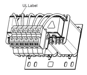
Terminals: 16 mm<sup>2</sup> Tightening torque: 1.2–1.4 Nm
