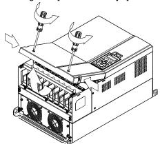
2. Remove the 5 screws shown in the following figure. Screw torque: 24–26 kg-cm / [20.8–22.6 lb-in.] / [2.4–2.5 Nm]
