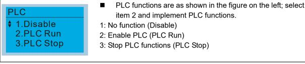
■ When the external multifunctional input terminals (MI1–MI8) are in PLC Mode select bit0 (51) or PLC Mode select bit1 (52), and the terminal contact is closed or open, it will compulsorily switch to the PLC mode, and keypad switching will be ineffective. Corresponding actions are as follows:
