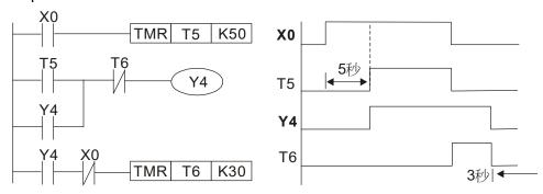
Example 12: Extended timing circuit
