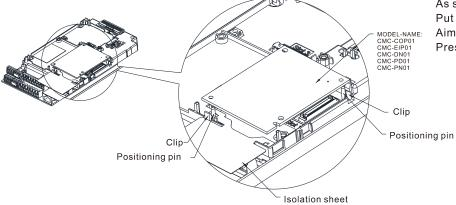
As shown in the figure on the left. Put the isolation sheet into the positioning pin. Aim the two holes at the positioning pin. Press the pin to clip the holes with the PCB.
