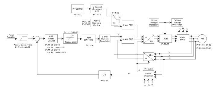
PM Sensorless FOC control is the control method dedicated for PM; it uses the high salient pole characteristic of PM to detect positions of NS magnetic poles. By doing this, it calculates the motor's rotor position at low-speed frequency.
