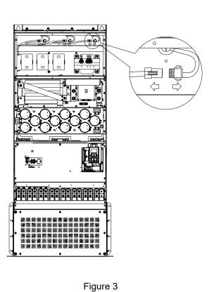
4. Loosen the screw 1–6 (as shown below) and remove the fan. Make sure fan power is disconnected before removal. Screw torque: 24-26kg-cm / [20.8-22.6 Ib-in.] / [2.4-2.5 Nm]
