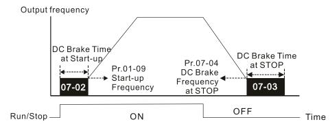
DC Brake Output Timing Diagram
