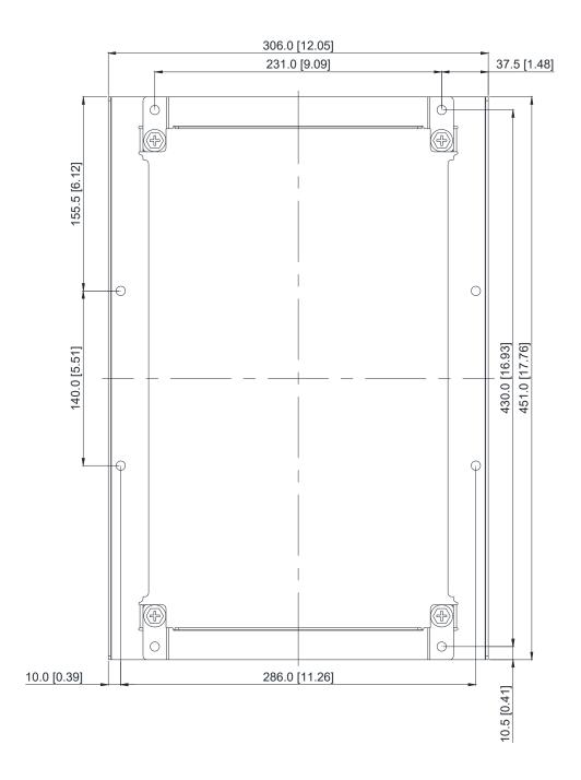
『MKC-CFM』 Installation 1. Install accessory 1 & 2 by fastening 4 of the screw 1 (M8). Screw torque: 50-55 kg-cm / [43.4-47.7 lb-in.] / [4.9–5.4 Nm] (As shown in the following figure)
