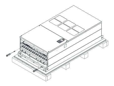
5. Install conduit box and accessories by fasten all the screws shown in the following figure. Screws 1–6: M6 screw torque: 55–65 kg-cm / [47.7–56.4 lb-in] / [5.4–6.4 Nm] Screws 7–9: M8 screw torque: 100–110 kg-cm / [86.7–95.4 lb-in] / [9.8–10.8 Nm] Screws 10–13: M10 screw torque: 250–300 kg-cm / [216.9–260.3 lb-in] / [24.5–29.4 Nm] Screws 14–17: M8 screw torque: 100–110 kg-cm / [86.7–95.4 lb-in] / [9.8–10.8 Nm]
