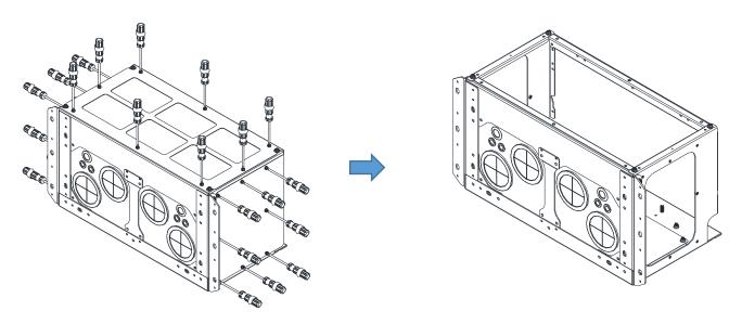
2. Loosen the screws as below figure shown.
