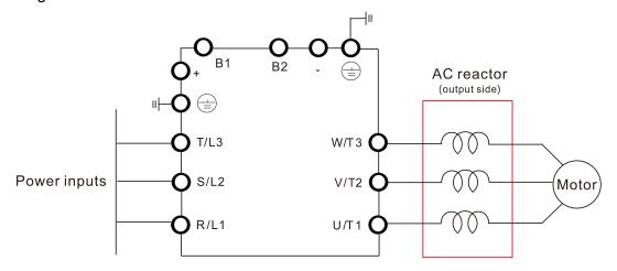
Wiring of AC output reactor
