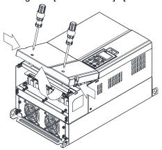
Remove the 5 screws shown in the following figure. Screw torque: 24–26 kg-cm / [20.8–22.6 lb-in.] / [2.4–2.5 Nm]
