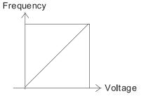
Fcmd=[(ay±bias)\*gain]\* Fmax(01-00) 10V or 16mA or 20mA Fcmd: the corresponding frequency of 10V or 20mA
