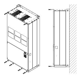
Screw M12\*6 Torque: 340–420 kg-cm / [295.1–364.6 lb-in.] / [33.3–41.2 Nm]
