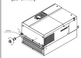
6. Fasten 5 screws (as shown in the following figure). Screw torque: 24–26 kg-cm / [20.8–22.6 lb-in.] / [2.4–2.5 Nm]
