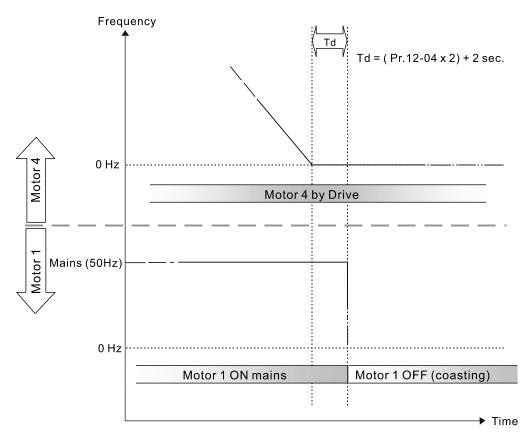
Diagram 12-6: Sequence of switching motors at Fixed Quantity Circulation with PID
