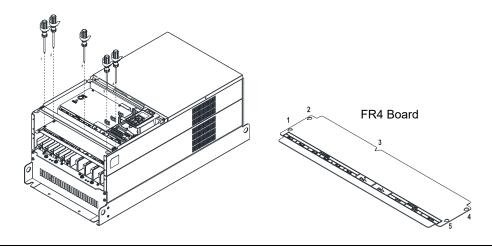
3. Loosen the upper M8 nuts (1–6) with a sleeve wrench (12mm of the sleeve). M8 Torque: 90 kg / [78.1 lb-in] / [8.8 Nm]
