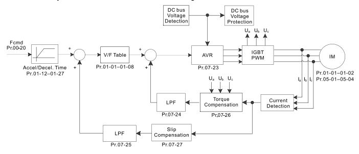
When you set Pr.00-11 to 2, the space vector control diagram is as follows. Induction Motor Space Vector Control (IMSVC)
