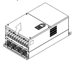
2. Loosen the screw (figure 2) and remove the cover. Screw torque: 24–26 kg-cm / [20.8–22.6 lb-in.] / [2.4–2.5 Nm]
