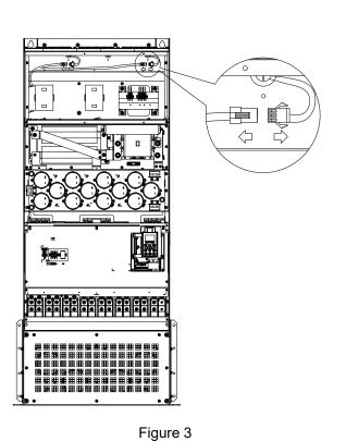
4. Loosen the screw 1–4 (as shown below) and remove the fan. Make sure fan power is disconnected before removal. Screw torque: 24–26kg-cm / [20.8–22.6 lb-in.] / [2.4–2.5 Nm]
