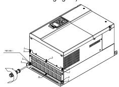
4. Fasten 5 screws (as shown in the following figure). Screw torque: 30–32 kg-cm / [26.0–27.8 lb-in.] / [2.9–3.1 Nm]
