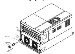
3. Fasten 4 screws (as shown in the following figure). Screw torque: 30–32 kg-cm / [26.0–27.8 lb-in.] / [2.9–3.1 Nm]
