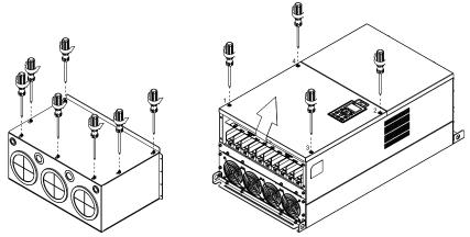
3 Remove the top cover and loosen the screws.
