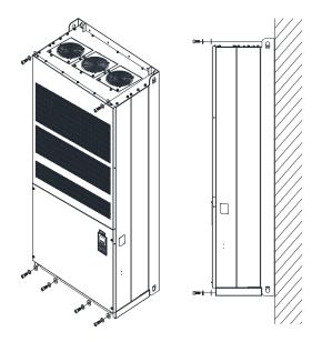
Screw M12\*6 Torque: 340-420 kg-cm / [295.1-364.6 lb-in.] / [33.3-41.2 Nm]
