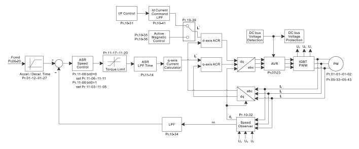
When you set Pr.00-11 to 8, SynRM Sensorless control diagram is as follows:
