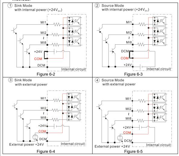
☑ When the photo coupler uses the internal power supply, the switch connection for Sink and Source modes shows as Figure 6-2 and Figure 6-3:
