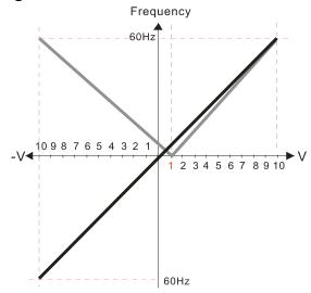
Pr.00-21=0 (Digital keypad control and run in FWD direction) Pr.03-05 Analog Positive Voltage Input Bias (AVI2) = 10%
