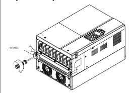
5. Fasten 4 screws (as shown in the following figure). Screw torque: 24–26 kg-cm / [20.8–22.6 lb-in.] / [2.4–2.5 Nm]
