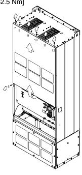
3. Press the latch to disconnect fan power (as shown in 4. Loosen the screw 13–18 and remove the fan. the enlarged picture of figure 3).
