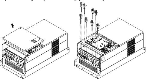
4 Install the conduit box by fastening all the screws shown in the following figure. M5 Screw torque: 24–26 kg-cm / [20.8–22.6 lb-in] / [2.4–2.5 Nm] M8 Screw torque: 100–120 kg-cm / [86.7–104.1 lb-in] / [9.8–11.8 Nm]
