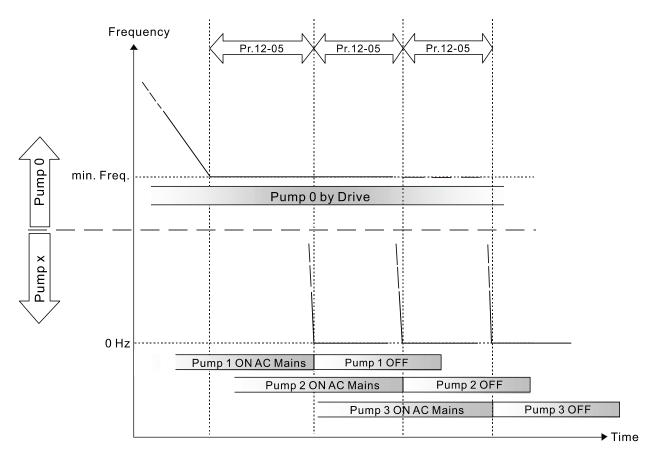
Diagram 12-11: Sequence of switching motors at Fixed Quantity Control with PID
