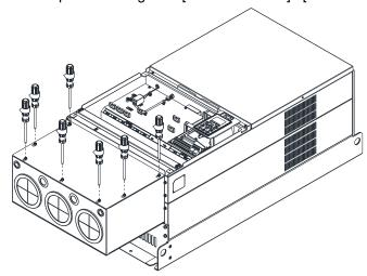
6. Place the cover back to the top and fasten the screws (as shown in the figure). Screw torque: 12–15 kg-cm / [10.4–13 lb-in.] / [1.2–1.5 Nm]
