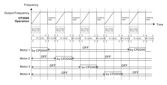
Diagram 12-1: Sequential Diagram of Fixed Time Free Runs Circulation (by time)
