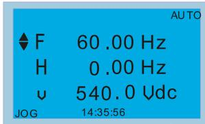
→ The top line of LCD displays the status of drive.
