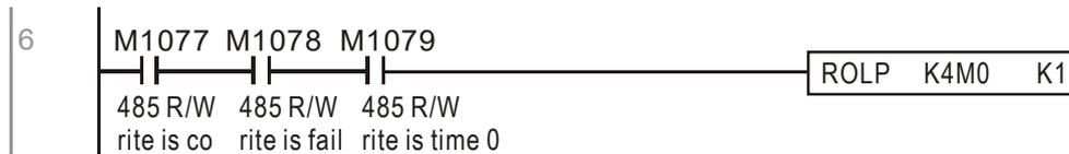
If time out occurs or an error is reported, the M1077 will change to ON. At this time, after a delay of 30 scanning cycles, it will re-issue the original command once
