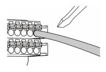
(4) Withdraw the screwdriver to complete the wiring.
