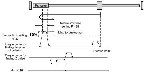
Note: the actual max. torque output of the motor is 10% higher than the torque limit setting (P1-87). For Example, if you set the torque limit P1-87 to 50%, and the max. torque output of the motor will be 60%.
