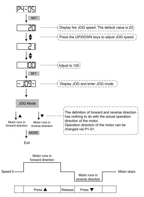
If the motor does not run, please check if the wiring between UVW and encoder cable is correct. If the motor runs abnormally, please check if the UVW phase sequence is correct.
