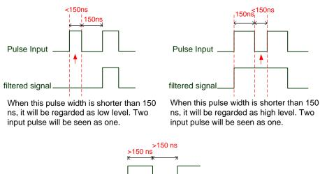
When High, Low duty of the pulse width are longer than 150 ns, it can ensure the pulse command will not be filtered.
