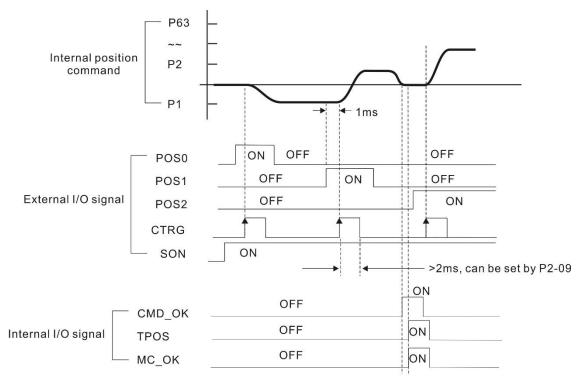
$\mathsf{CMD\_OK}:\mathsf{CMD\_OK}$  is activated when the servo drive has detected that  $\mathsf{Pr}$  command has been completed
