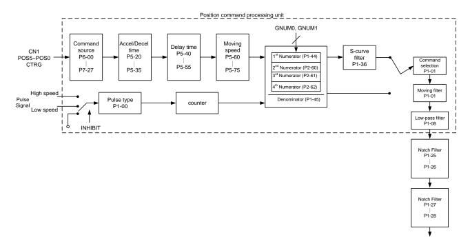
The upper path of the above diagram is PR mode and the lower one is PT mode, which could be selected via P1-01. Both modes can set E-gear ratio for the proper position resolution. Moreover, either S-curve filter or low-pass filter can be used to smooth the command. See the description in later parts.
