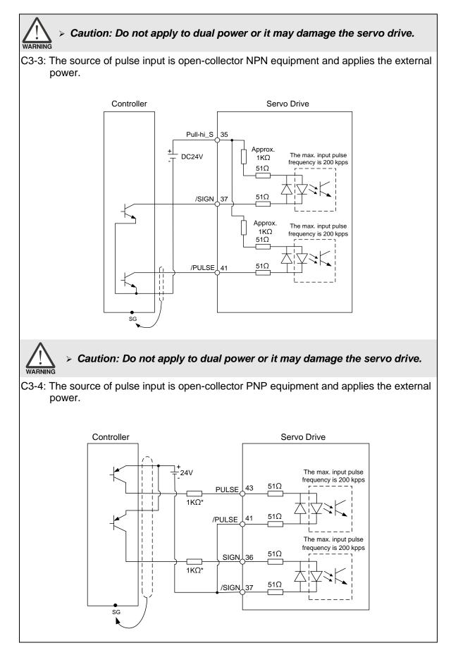
Note: Resistor of 1 k $\Omega$  (1 w) has to be connected.
