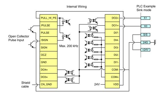
Wiring and installation of CN1 quick connector:
