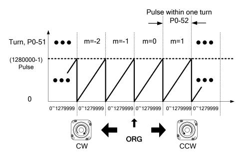
Figure 12.1 Pulse counting in absolute coordinate system
