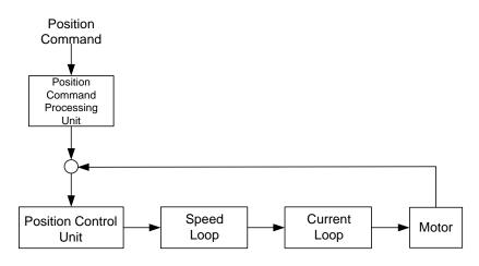
For a better control, the pulse signal should be processed and modified through position command processing unit. The structure is shown as the diagram below.
