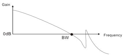
If users know the resonance frequency, notch filter (parameter P2-23 and P2-24) can directly eliminate the resonance. The frequency setting range of notch filter is merely from 50 to 1000 Hz. The suppression strength is from 0 to 32 dB. If the resonance frequency is not within the range, it is suggested to use low-pass filter (parameter P2-25).
