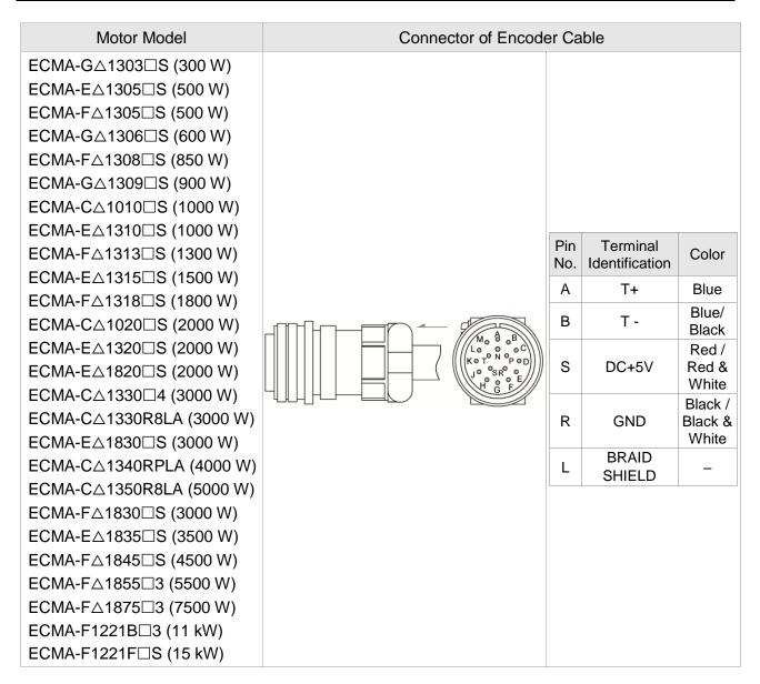
Please select shielded multi-core and the shielded cable should connect to the SHIELD end. Please refer to the description of Section 3.1.6.
