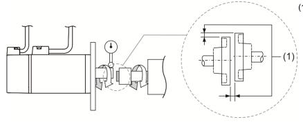
(1) The distance is measured at four different positions on the circumference for the centering accuracy. The difference between the maximum and minimum measurement values must be 0.03 mm or less; and even within this range, you can make adjustments to increase the centering accuracy as much as possible.
