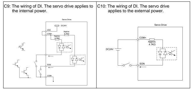
PNP transistor, common emitter (E) mode (SOURCE mode)
