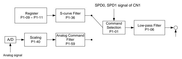
The upper path is the command from register while the lower one is external analog command. The command is selected according to the status of SPD0, SPD1, and P1-01 (S or Sz). Usually, S-curve and low-pass filter are applied for having a smooth resonance of command.
