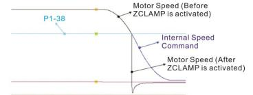
1: The command source is analog speed command. ZCLAMP function will use the analog speed command without acceleration / deceleration processing to judge if this function is enabled. When ZCALMP conditions are established, the motor speed decelerates to 0 through S-curve. If not, the motor follow the analog speed command through S-curve.
