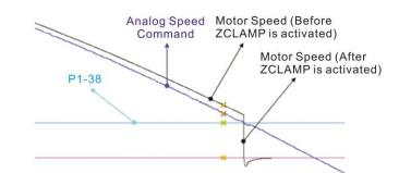
0: The command source is register. ZCLAMP function will use the register speed command with acceleration / deceleration processing to judge if this function is enabled. The motor will be locked at the position where ZCALMP conditions are established.
