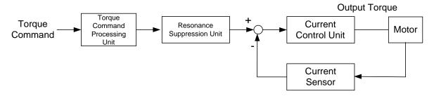
The torque command processing unit is to select torque command source according to Section 6.4.1, including the scaling (P1-41) setting and S-curve setting. The current control unit manages the gain parameters of the servo drive and calculates the current for servo motor in time. Since the current control unit is very complicated and is not relevant to the application, there is no need to adjust parameters. Only command end setting is provided.
