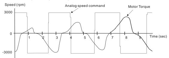
Analog speed command filter smoothes the analog input command. Its time program is the same as S-curve filter in normal speed. Also, the speed curve and the acceleration curve are both continuous. The above is the diagram of analog speed command filter. The slope of speed command in acceleration and deceleration is different. Users could adjust the time setting (P1-34, P1-35, and P1-36) according to the actual situation to improve the performance.
