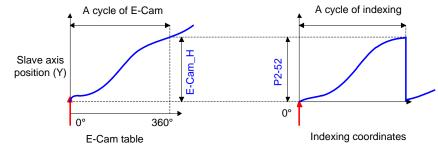
Note 1: ECAM\_H (height of E-Cam table) = E-Cam table (last point - first points)
