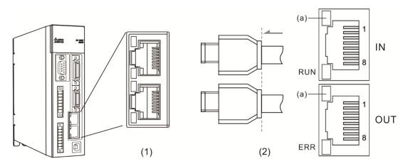
(1) CN6 connector (Female); (2) CN6 connector (Male) (a) Network status indicator
