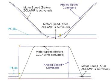
1: The command source is register. ZCLAMP function will use the register with acceleration / deceleration processing to judge if this function is enabled. When ZCLAMP conditions are established, the motor speed will be set to 0.
