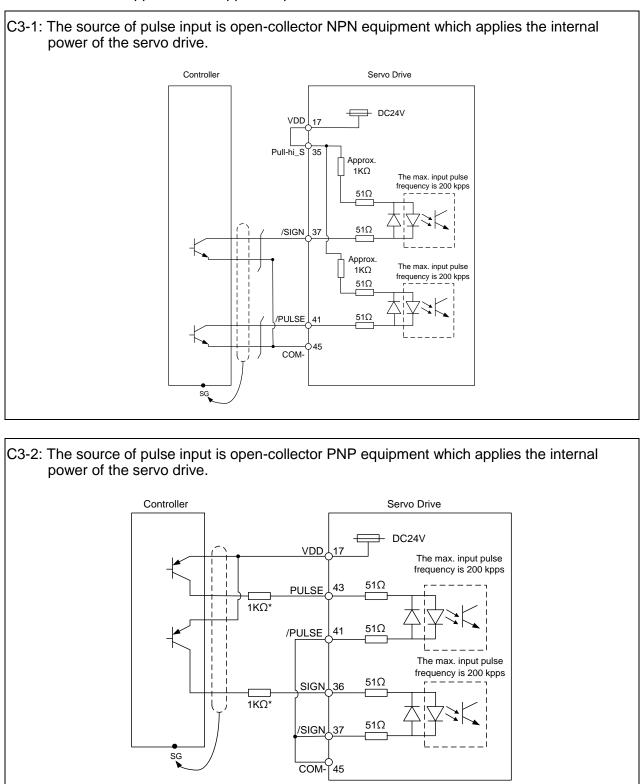
Note: Resistor of 1 k $\Omega$  (1 w) has to be connected.
