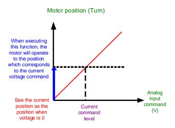
1: After the servo is on, if the command level is not changed, the motor will not operate. The position the motor stops at is the position that corresponds to the current command level.
