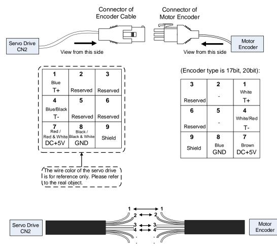
If not using housing and directly wiring the cores, please follow the corresponding core number for wiring. For example, core number 1 from the servo drive CN2 should connect to core number 1 from the motor encoder; core number 2 from the servo drive CN2 should connect to core number 2 from the motor encoder and so on. Please number the cores from the servo drive in order and then connect it to the encoder.
