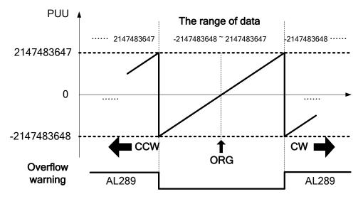
Figure 12.2 PUU counting in absolute coordinate system
