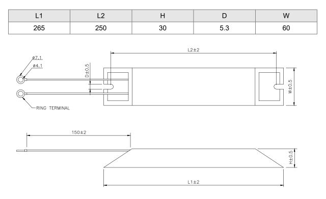
Delta Part Number: BR1K0W020 (1 kW 20Ω), BR1K5W005 (1.5 kW 5Ω)
