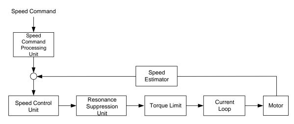
The speed command processing unit is to select speed command source according to Section 6.3.1, including the scaling (P1-40) setting and S-curve setting. The speed control unit manages the gain parameters of the servo drive and calculates the current command for servo motor in time. The resonance suppression unit is to suppress the resonance of mechanism. Detailed descriptions are shown as the following:
