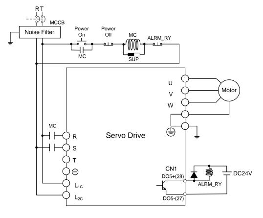
■ Wiring Method of Three-phase Power Supply (suitable for all series)
