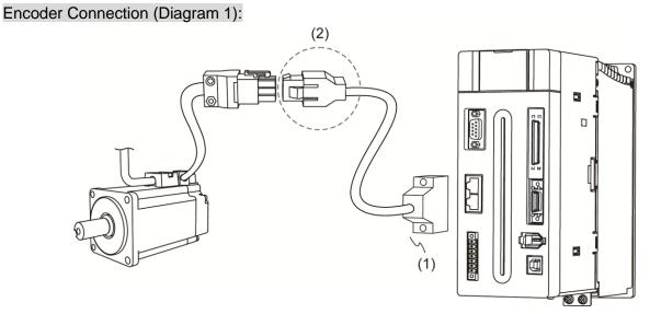
(1) CN2 connector; (2) Quick connector (connector of encoder cable)
