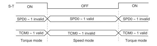
In torque mode (S-T is ON), the torque command is selected via TCM0 and TCM1. When switching to speed mode (S-T is OFF), the torque command is selected via SPD0 and SPD1. The motor operates according to the speed command. When S-T is ON, it goes back to the torque mode again. Please refer to the introduction of single mode for DI signal and the selected command of each mode.
