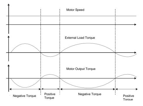
Negative torque: TL × Wr TL: external load torque
