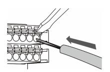
(3) Insert the stripped wire into the pin.
