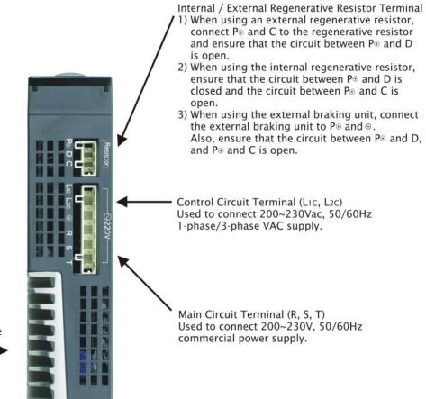
Heatsink Used to secure servo drive and for heat dissipation.
