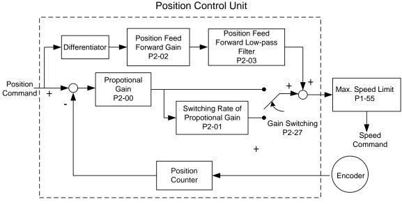
When the value of proportional gain, KPP, is set too big, the bandwidth of position loop will be increased and diminish the phase margin. And the motor rotor rotates vibrantly in forward and reverse directions at the moment. Thus, KPP has to be decreased until the rotor stops vibrating. When the external torque interrupts, the over-low KPP cannot meet the demand of position error. In this situation, parameter P2-02 can effectively reduce the following error.
