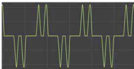
Motor drive without DC choke THDi 107%
